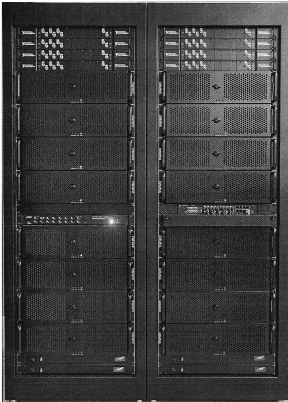
Figure 2.7: Front view of the 16-Node PC-Cluster at UBC Power Lab
