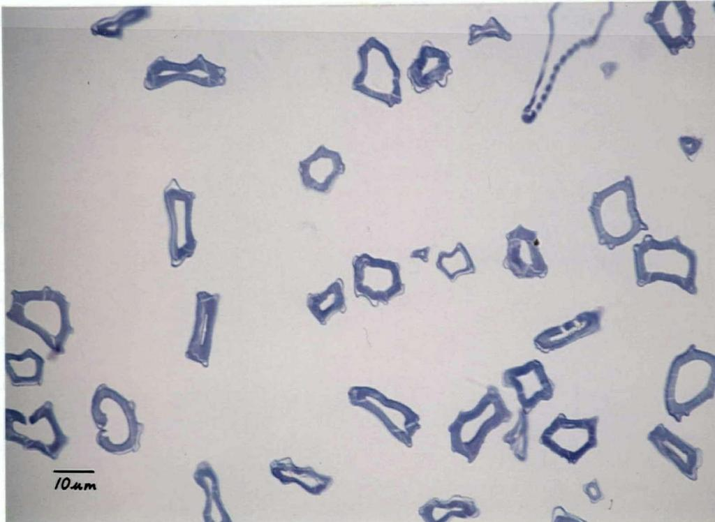
Figure 5.12a. Unbeaten birch kraft pulp fibres in cross section showing gaps between the  $S_1$  and  $S_2$  layers in bright field illumination.
