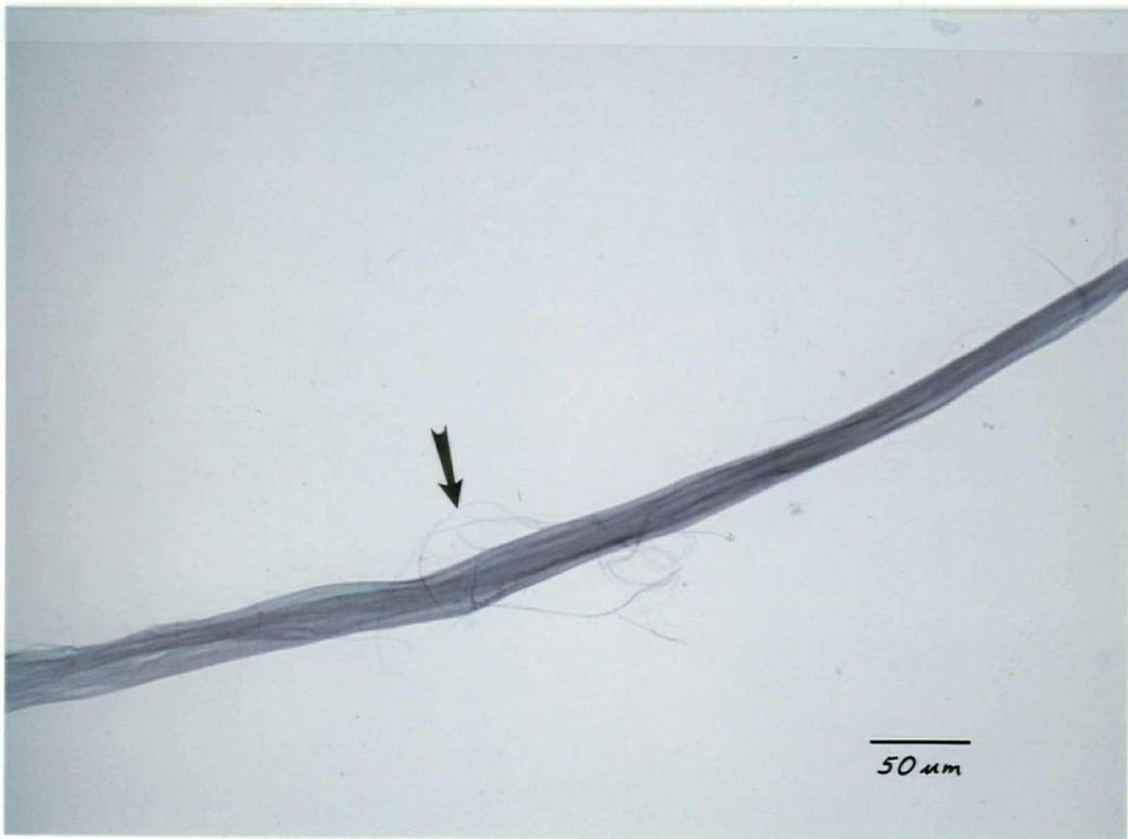
Figure 5.38. Isolated G-layer showing fine cellulose filaments detaching from the surface. Fraction 48/100 fraction of pulp A-TMP3.
