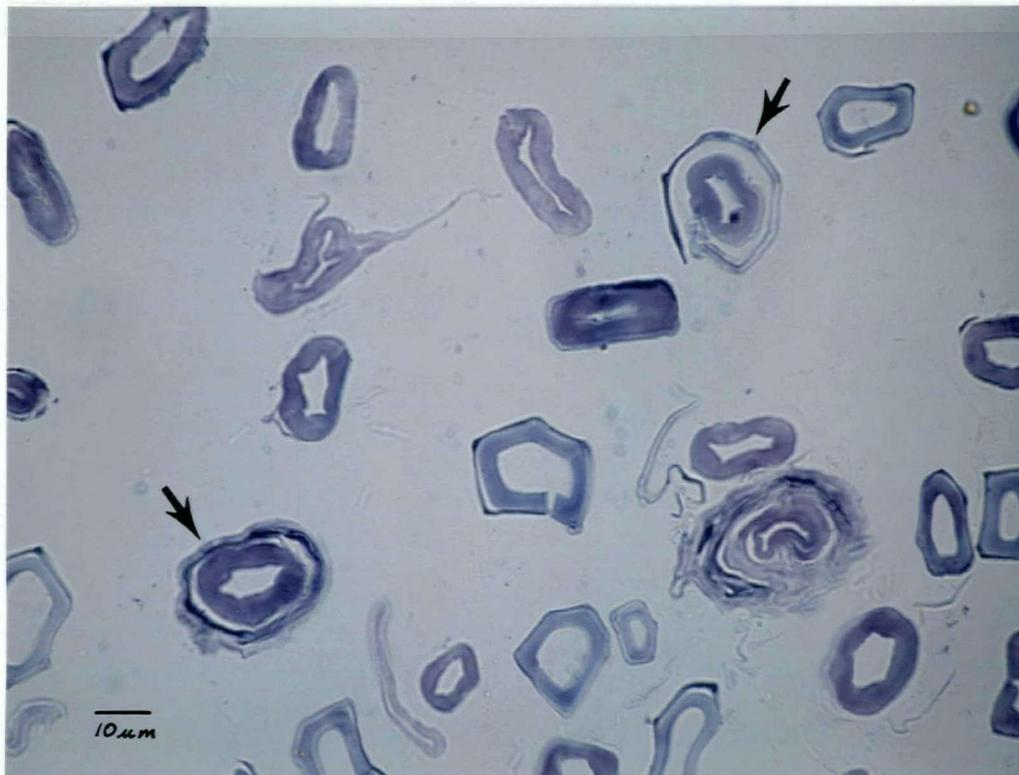
Figure 5.14. Birch CMP pulp fibres in cross section. Note the fibres in which the S<sub>1</sub> layer has completely separated but surrounds the fibre (pulp B-CMP4).
