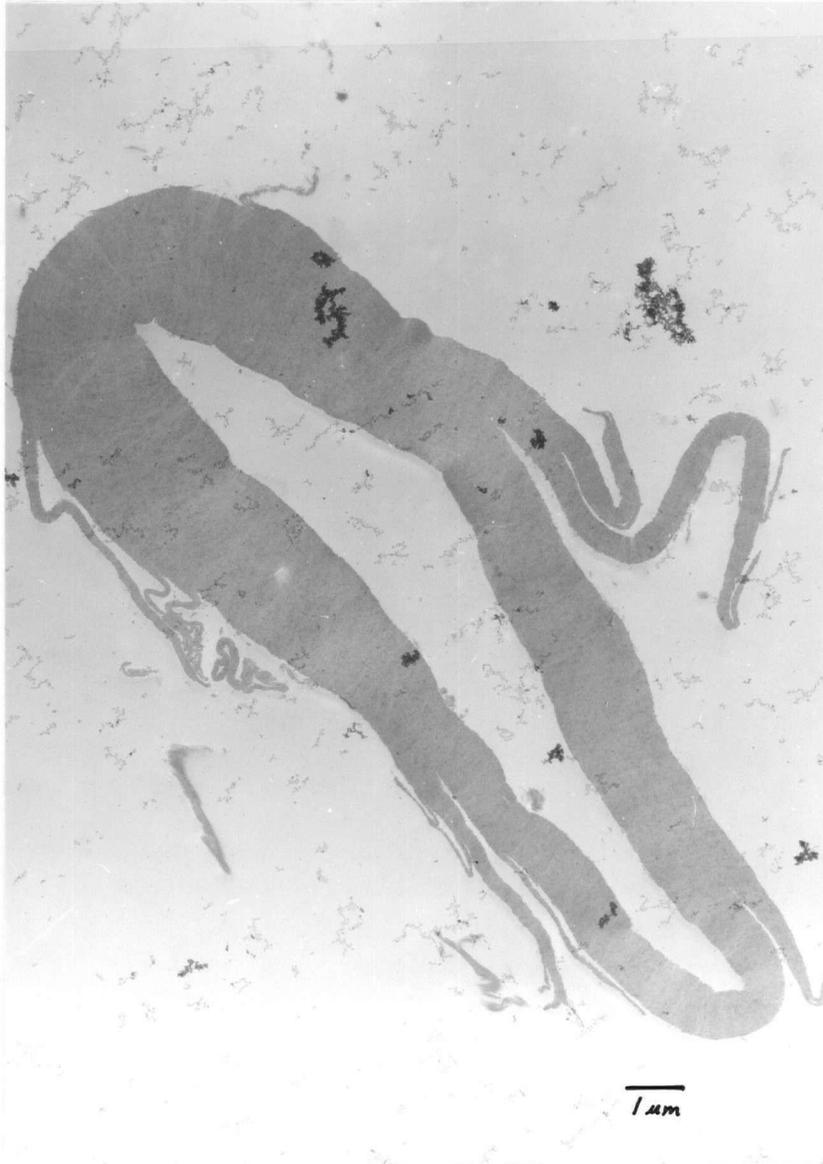
Figure 5.25. TEM photograph of a birch CMP fibre in cross section showing delamination of the S<sub>2</sub> layer (pulp B-CMP4).
