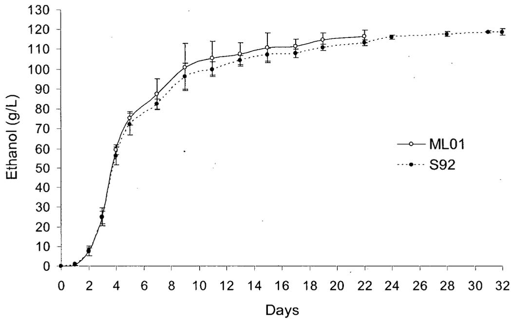
**Figure 15.** Ethanol production by ML01 (?) and S92 (?) in high-acid Chardonnay grape must fermented at 20 °C was positively affected by introduction of the malolactic cassette into a *URA3* locus in the industrial wine yeast S92. ML01 completed the alcoholic fermentation to a specific gravity of 0.996 in 22 days and the parental strain in 32 days. Duplicate biological replications were analysed in triplicate.
