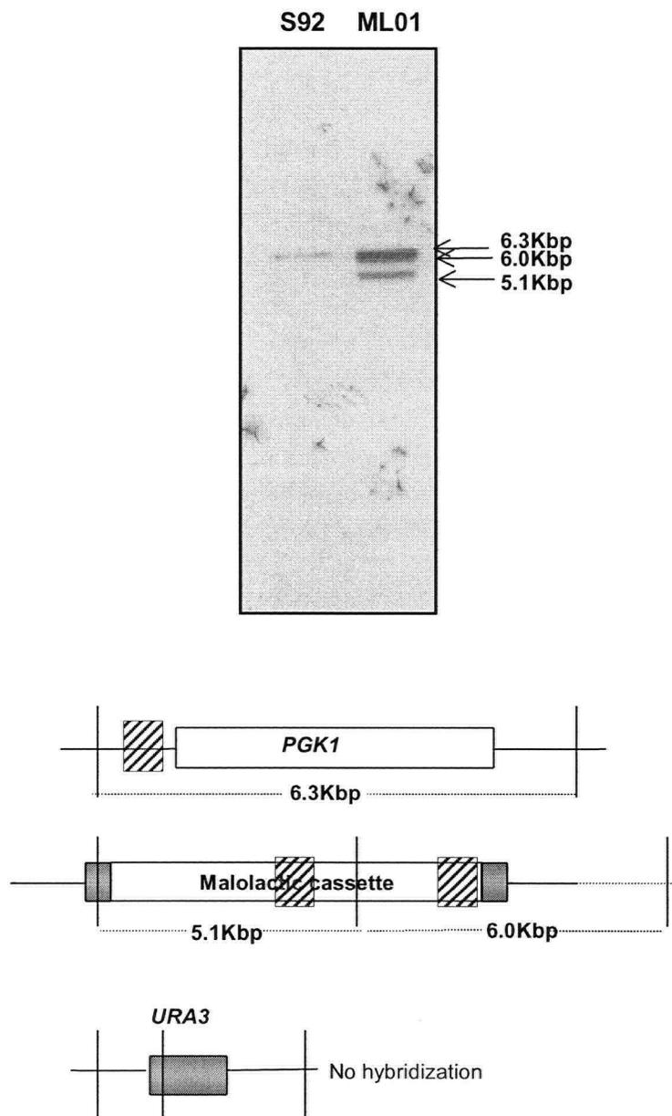
**Figure 25.** Integration of the malolactic cassette into the *URA3* locus of S92 was confirmed by Southern blot analysis using a *PGK1* promoter probe. The schematic representation illustrates the *EcoRV* restriction sites with vertical lines and the *PGK1* promoter probe hybridization site is depicted as hatched boxes in the lower panel.
