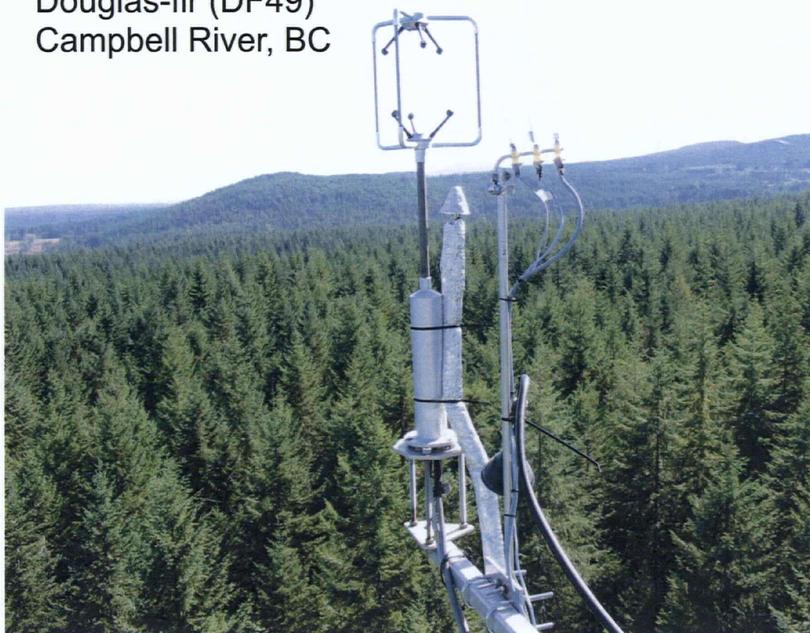
Figure A-2. View of the 56-year-old Douglas-fir stand on Vancouver Island. The (eddy covariance) system consists of a 3-D sonic anemometer and a closed-path infrared gas analyzer.
