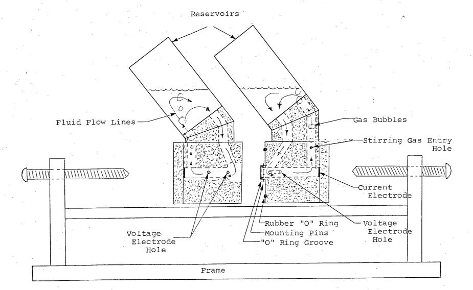
mixture of 95% O<sub>2</sub> and 5% CO<sub>2</sub> was used to provide adequate oxygenation in the absence of intact tracheal connections. Fluid circulation was both rapid and turbulent inside the chambers especially near the membrane as determined by injection of dye at various points in the chamber and reservoirs. Injected dye returned to its starting point in much less than a second and fluid in the reservoirs and chambers became uniformly colored by the dye within a few seconds.
