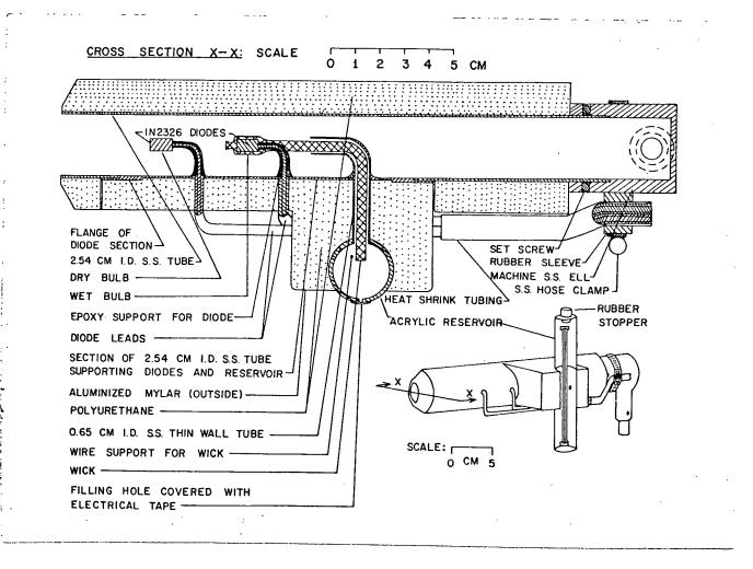
Figure 2 Sensing head design. The second head is a mirror image of the head illustrated.
