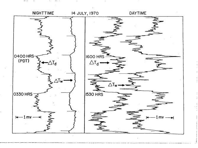
Figure 5 Typical traces of dry bulb and wet bulb differences over 1 meter ( $\Delta T_d$  and  $\Delta T_w$ ) obtained with the psychrometric apparatus. Diode sensitivity is 2.25 mv C-1.
