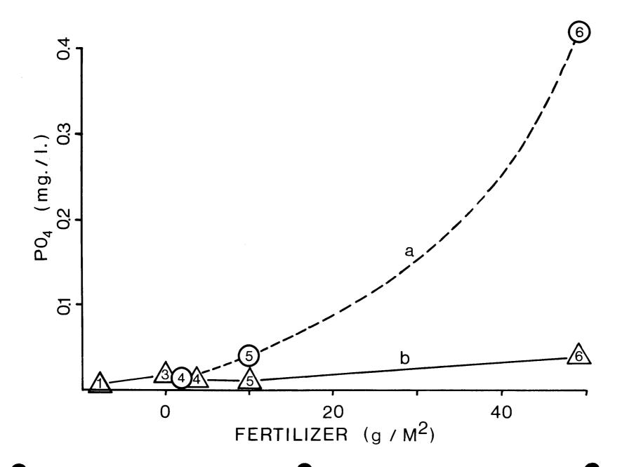
Fig. 5 Ortho phosphate concentrations in the water of the two small enclosures over time following the addition of two different amounts of fertilizer. (enclosures flushed on day 12)
