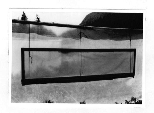
were accomplished in a further set of enclosures. These plywood structures were 1 m square and had sliding sides which could be removed to expose the enclosed sediment to the full flushing of the water current. They were located adjacent to the larger enclosures in positions marked "a" and "b" in (Fig. 1).
