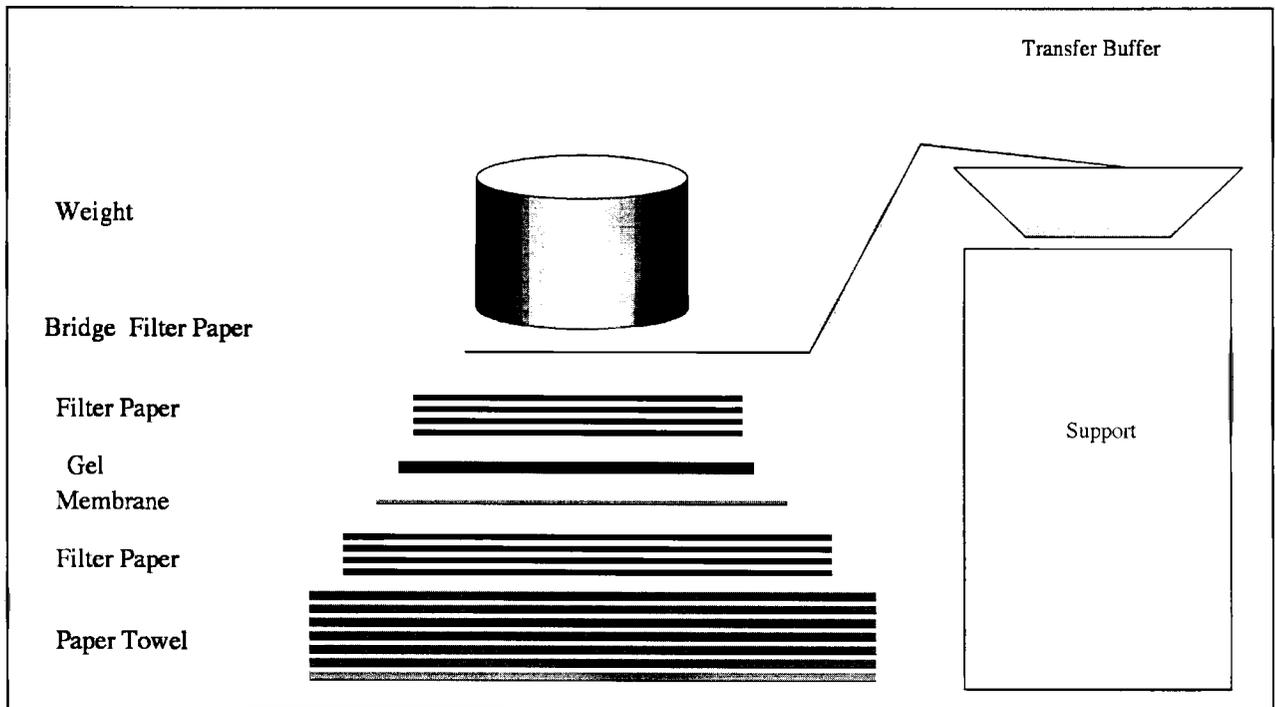
Figure 4- **Passive transfer by denaturing agarose blotting for Southern blots.** This low-tech method for agarose transfer is by a passive, alkaline, downward elution. The pyramid like setting prevents the shortcircuit between the membrane and the layers, and allows a safe and complete transfer
