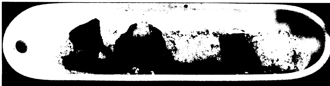
Figure 3.3: \text{BaCuO}_2 ceramic after oxygen anneal to remove \text{CO}_2 and subsequent brief storage at room temperature. Upon removal from the furnace, all pieces were black. The oxygen was flowing from right to left, so the pieces to the right had nearly all carbon dioxide removed, while those downstream, to the left, did not. For \text{CO}_2 to re-enter the ceramic at right, the ceramic had to decompose.
