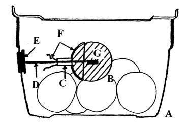
Figure 6.1 Particle and thermocouple structure for thermal indicator studies – rigid thermocouple.
