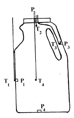
Figure 7.1 Thermocouple junction and DSC pan (thermal indicator) placement for pasteurisation studies – plastic jugs. Letters "P" with numerical subscripts denote DSC pans, letters "T" with numerical subscripts denote thermocouples.
