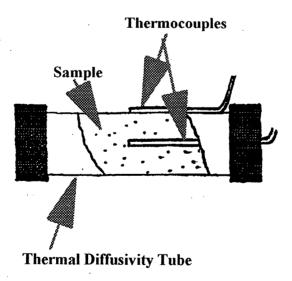
Figure 3.1. Assembly of thermal diffusivity tube.
