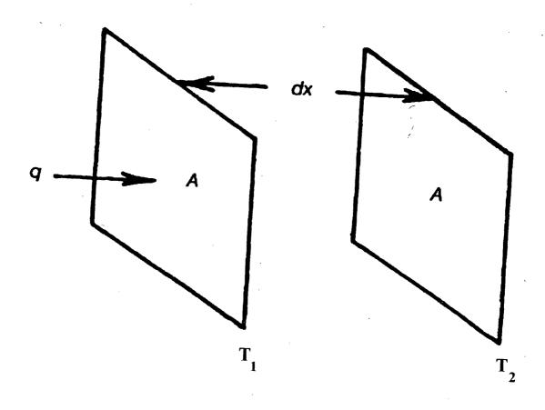
Figure 2.1. Conventions for conductive heat flow (Watson and Harper, 1987).
