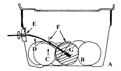
Figure 6.2 Particle and thermocouple structure for thermal indicator studies - flexible thermocouple. Legend: A) 307 OMNI® bowl, B) potato/alginate gel particle, C) rubber tubing, D) thermocouple, E) mounting receptacle, F) dental floss, G)DSC pan.
