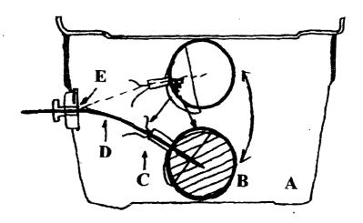
Figure 4.3. Structure and use of a flexible thermocouple mounted in a plastic container to monitor the centre temperature of a potato/alginate gel sphere. Legend: A) 307 OMNI® bowl, B) potato/alginate gel sphere, C) rubber tubing, D) thermocouple, E) mounting receptacle, F) dental floss.
