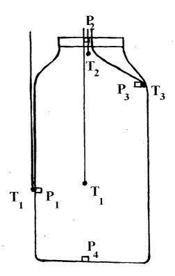
Figure 7.2 Thermocouple junction and DSC pan (thermal indicator) placement for pasteurisation studies – glass jar. Letters "P" with numerical subscripts denote DSC pans, letters "T" with numerical subscripts denote thermocouples.
