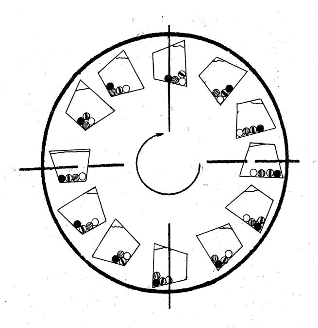
Figure 4.4 Movement of free particles at 2.8 rpm.
