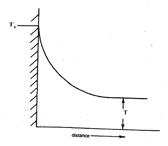
Figure 2.2. Temperature profile in a fluid moving past a surface at temperature  $T_s$  (Watson and Harper, 1987).
