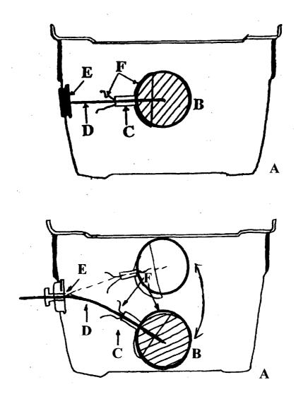
Figure 5.1 Rigid versus flexible thermocouples. Legend: A) 307 OMNI® bowl, B) potato/alginate sphere, C) rubber tubing, D) thermocouple, E) mounting receptacle, F) dental floss.
