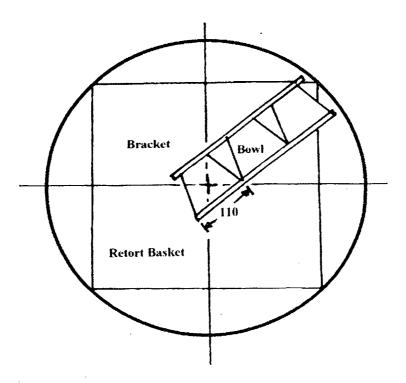
Figure 4.2. Orientation of bowls for videotape study of particle movement in Lagarde lab simulator retort at 2.8 rpm.
