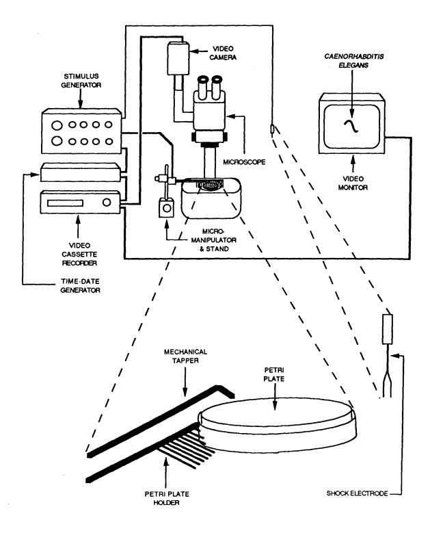
S88 stimulator which was set to deliver a signal of six 25-ms pulses at 60 V and a rate of 8.5 pulses per second. <u>Procedure</u>
