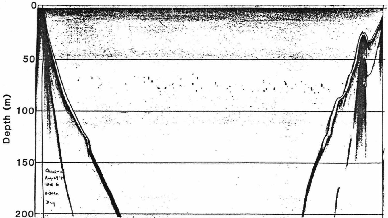
Figure 4-4. A) Diel echogram sequence from Quesnel Lake on Aug.23-24, 1986, indicating daytime disappearance of fish targets from field of 15 degree transducer (echogram marks between 40-80 m due largely to electrical noise), and B) daytime echogram with 6 degree transducer showing juvenile sockeye fish targets between 60-90 m.
