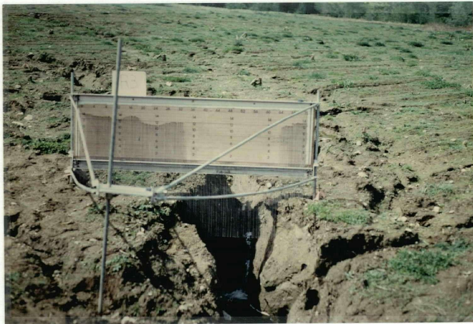
Figure 1.9: Accelerated rill erosion due to a blocked ditch culvert.
