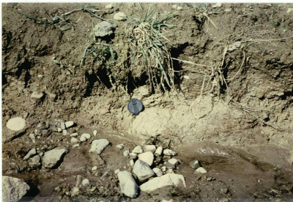
Figure 2.6: Rill erosion exposing the A_p horizon and the underlying C horizon
