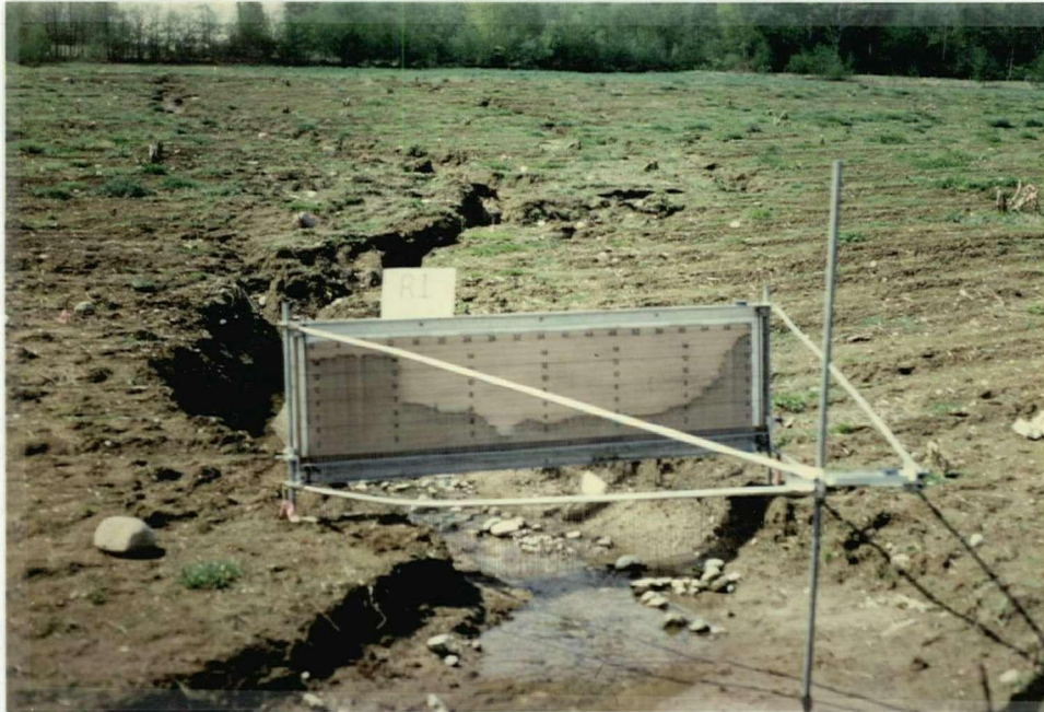
Figure 1.3: The portable photographically recording rill meter.
