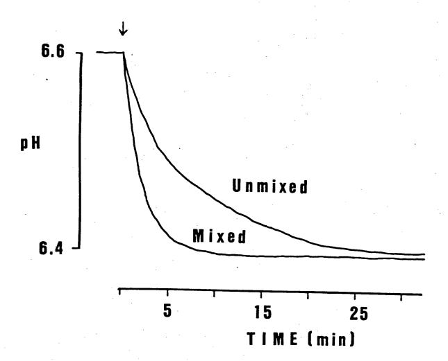
the system detects pH differences due to  ${\rm CO_2}$  hydration, and the  ${\rm t_{1/2}}$  value for the mixed reaction is in approximate agreement with values given by Kern (1960) at the test pH and temperature.
