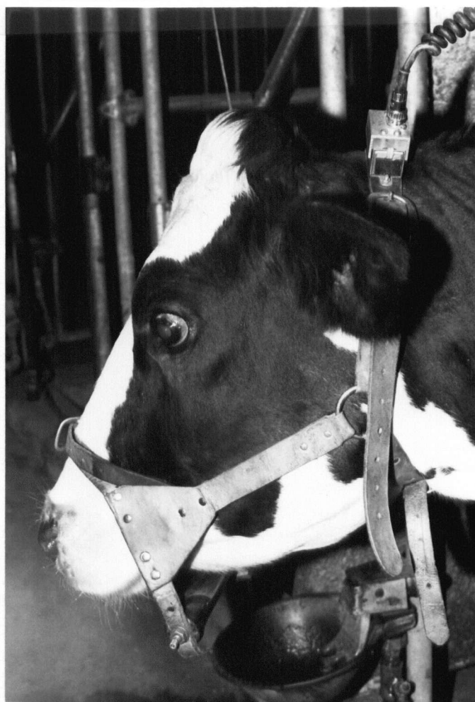
FIGURE 16: Chewing monitor halter with pneumatic device and pressure transducer mounted.
