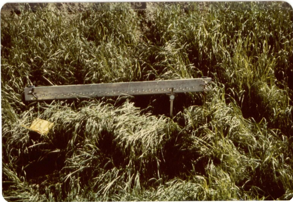
Figure 15. Rill-meter in use at Koksilah, April 1977.
