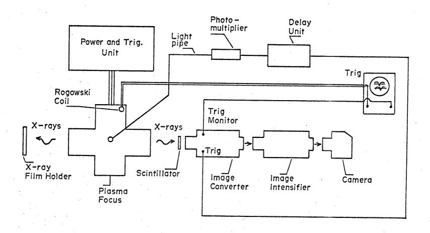
Figure 8. Triggering arrangement.
