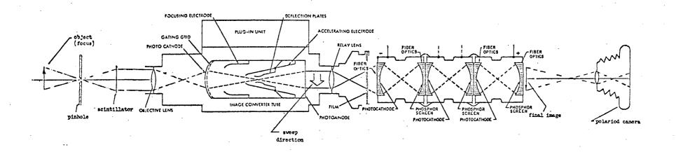
Figure 7. Electro-optical X-ray camera.
