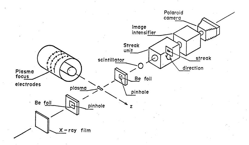
Figure 5. Illustration of optical arrangement.
