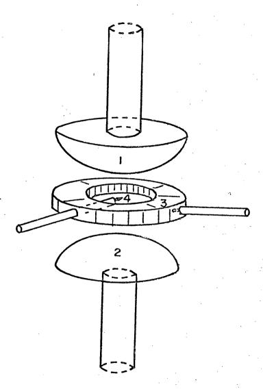
Figure 3. Spark gap electrodes.
