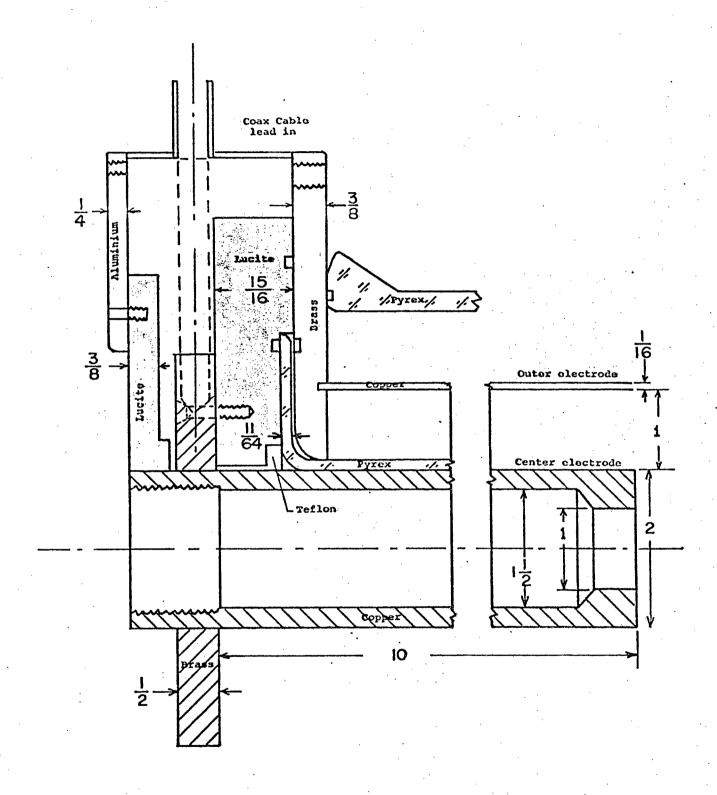
Figure 2. Electrode assembly.
