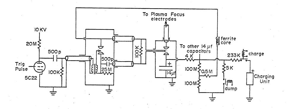
Figure 4. Electrical circuit of the plasma focus.
