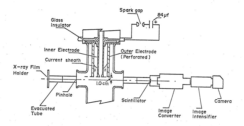
Figure 1. Experimental arrangement.
