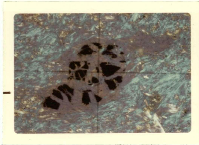
Plate 9: Photomicrograph of an aggregate of chlorite surrounding fragments of chrome spinel (#15; Van Decar Creek), crossed nicols with gypsum plate.
