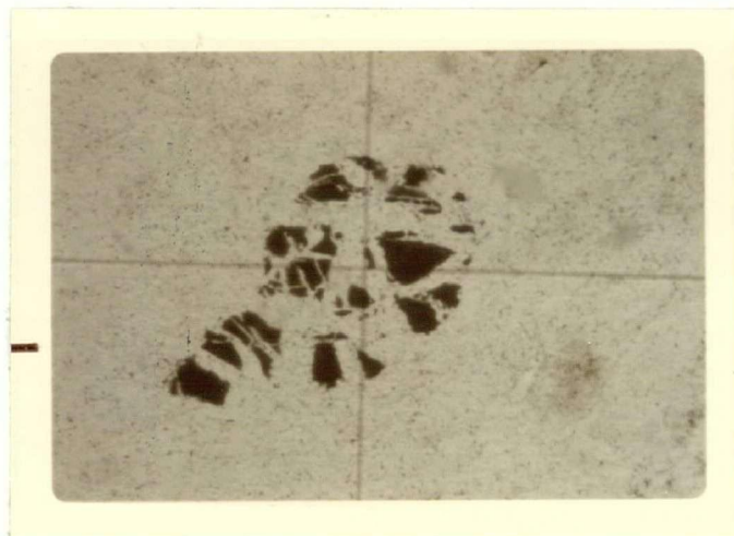
Plate 10: Photomicrograph of a fractured chrome spinel grain, partially replaced by chlorite (#15; Van Decar Creek), plane polarized light.
