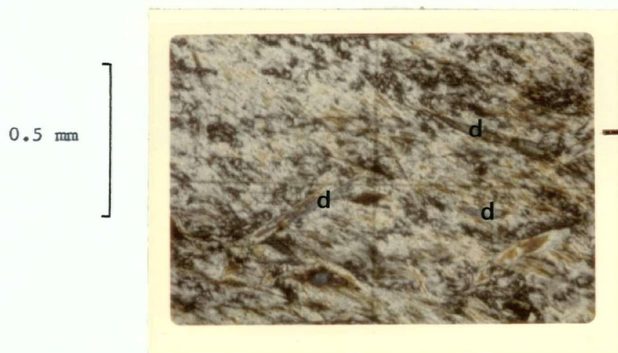
Plate 12: Photomicrograph of spindle-shaped diopside crystals (d), (#43; Ogden Mountain), crossed nicols.
