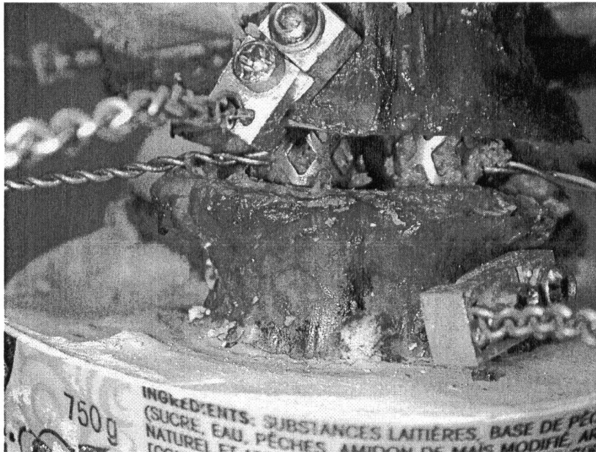
Figure 2.15 Close-up of braided wires coupled to vertebrae and cages.
