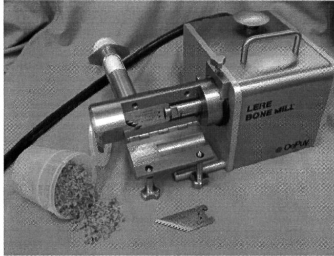
Figure 2.1: Pneumatic bone mill used to morsellize the femoral heads. The course blade is mounted and the fine blade is shown below the mill.
