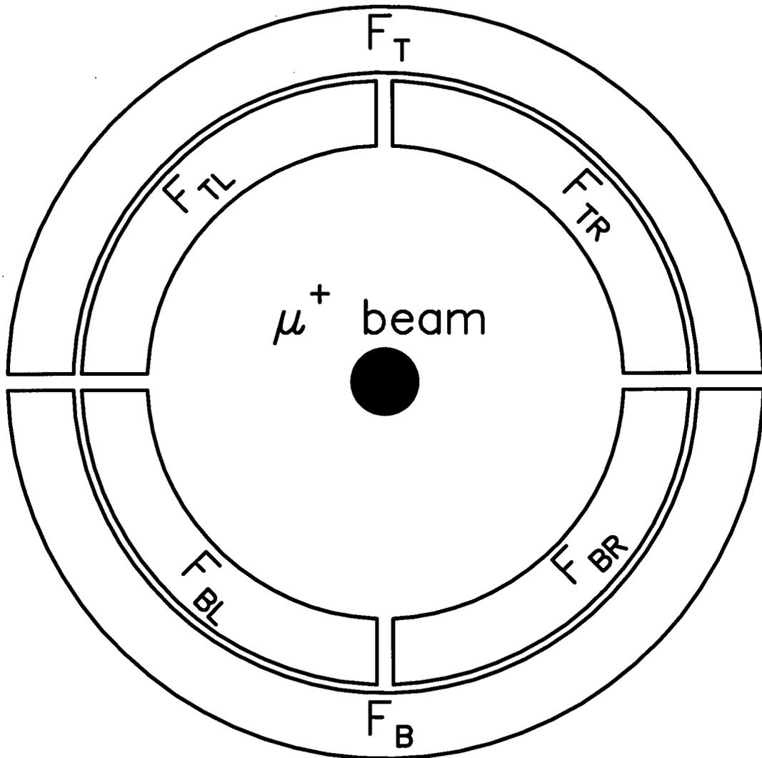
Figure 4.2: Cross-sectional view of forward positron counters  $F_i$  and  $F_{ij}$  ( $i = T$  or  $B$  and  $j = L$  or  $R$ ) as seen by the muon beam (represented as travelling into the page). The valid detection of a decay positron requires both the  $F_i$  and  $F_{ij}$  counters to trigger simultaneously ( $F_i \cdot F_{ij}$ ).
