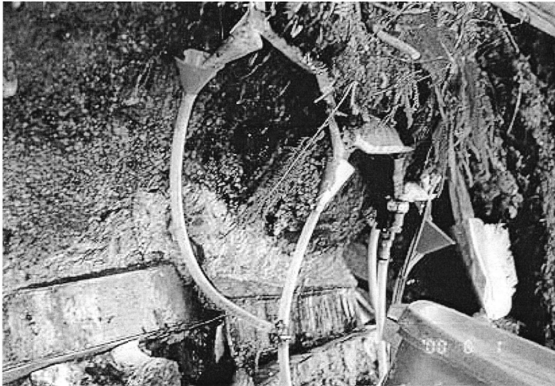
Figure 2.9 Collection of organic (funnels) and mineral (trough) outflows.
