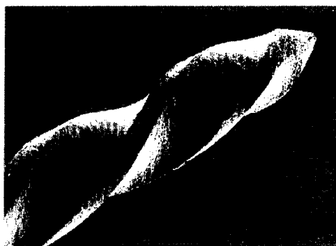
Figure 3- Profile R 0.04 taper series 29 R (Electron microscope image X125), flutes with flat outer edge and bullet nosed tip. (Thompson & Dummer, 1997, 2a)
