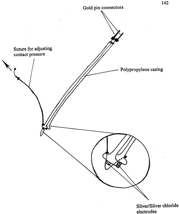
Figure 14. Schematic representation of the contact electrode developed for recording epicardial MAPs.
