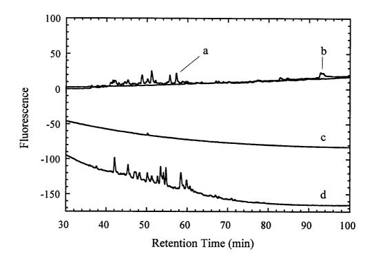
Figure 4: Chromatograms of trypsin digested Pgp labeled with various fluorescent probes.
