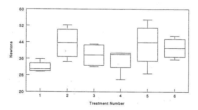
Figure 16 Boxplot of the Instron TPA parameter Hardness 1 for cooked, cultured chinook salmon samples, results by treatment number
