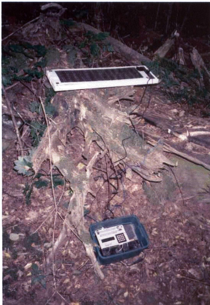
Figure 24. Photo of datalogger setup.
