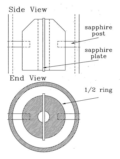
Figure 2.4: The New Resonator - Close up of the rings and plate only
