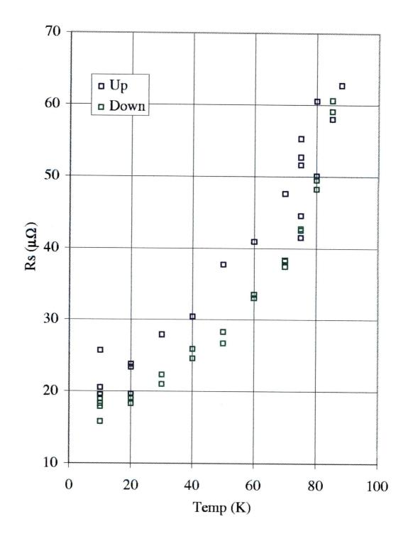
Figure 5.28:  $R_S$  for all samples at 3.7 GHz – Linear Plot
