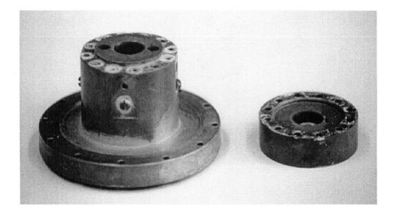
Figure 3.6: Photo of the original design. On the left is the upper portion with the large vacuum flange and on the right is the bottom cap. Corrosion from etchants is clearly visible.
