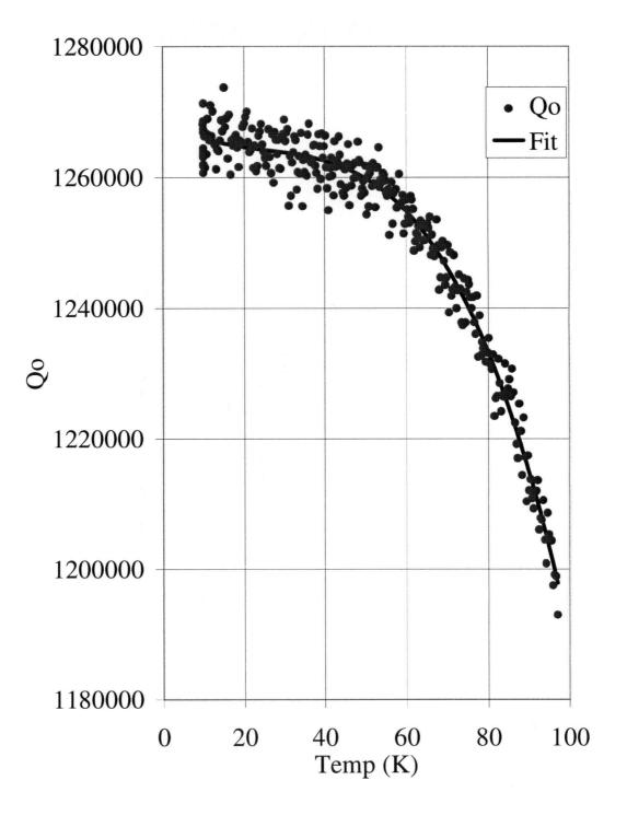
Figure 4.15: Temperature dependence of Qo at 910 MHz including the fitted values
