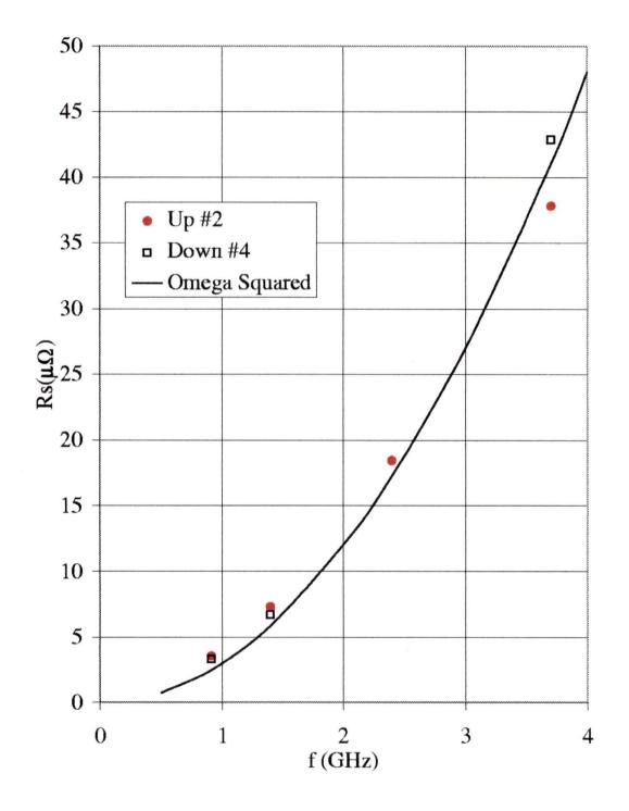
Figure 5.34: Frequency dependence of  $R_S$  at 70K. The solid line is proportional to  $\omega^2$ .
