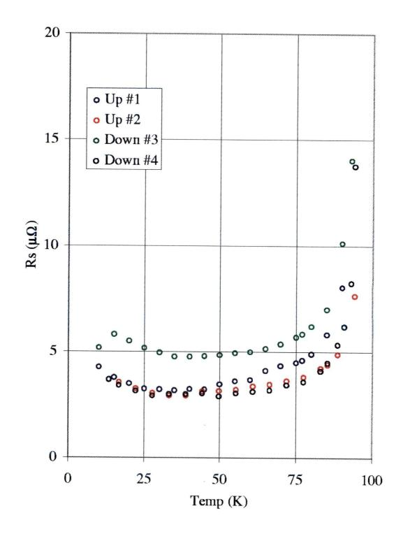
Figure 5.22:  $R_S$  for all samples at 0.95 GHZ – Linear Plot. The losses for Down #3 and the higher temperatures for Down #4 and Up #2 are somewhat in question.
