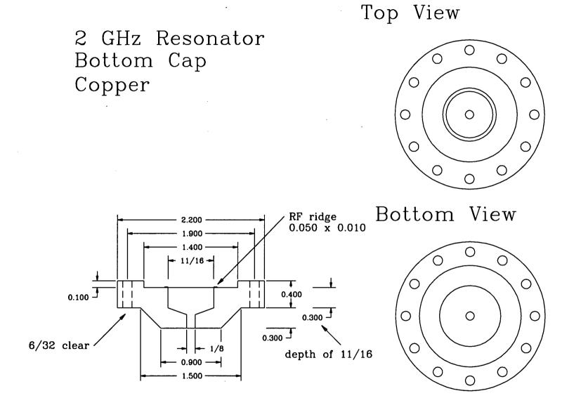
Figure B.40: Resonator Bottom Cap
