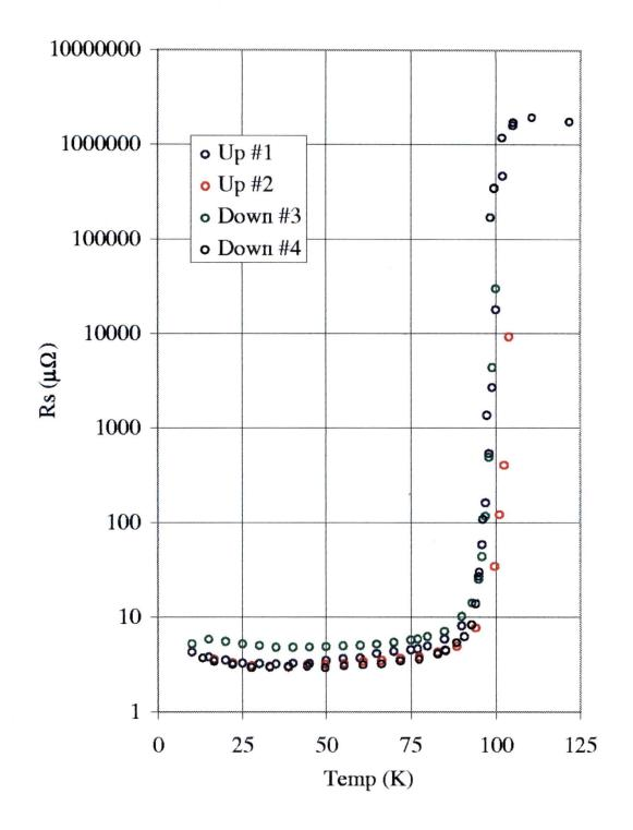
Figure 5.21:  $R_s$  for all samples at 0.95 GHZ – SemiLog Plot. The losses for Down #3 and the higher temperatures for Down #4 and Up #2 are somewhat in question.
