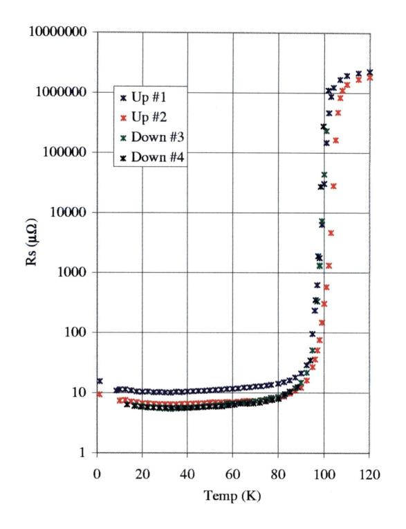
Figure 5.23:  $R_s$  for all samples at 1.4 MHz – Semi-Log Plot. The losses for Up#1 and the temperatures for Down #4 are somewhat in question.
