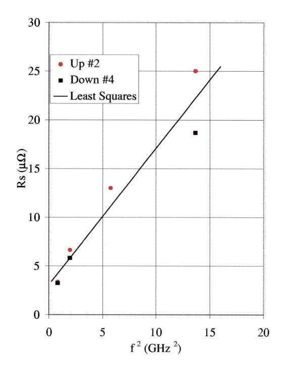
Figure 5.36: Frequency dependence of  $R_S$  at 20K graphed as a function of frequency squared. The intercept of the least squares fit is near  $3.1\mu\Omega$ .
