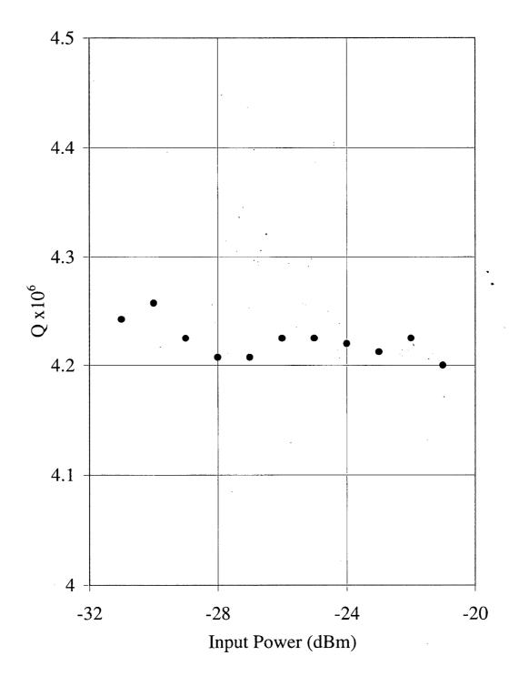
Figure 3.12: Power dependence of the Q factor for the third prototype.
