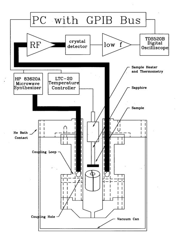
Figure 4.14: Microwave Set-Up
