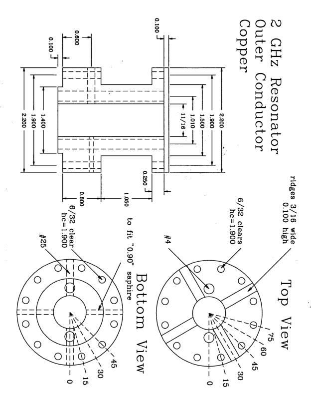
Figure B.39: Resonator Core
