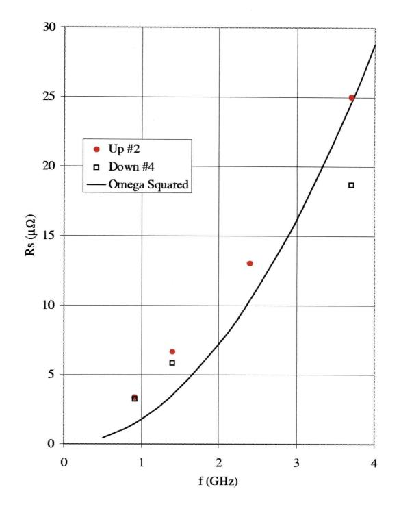
Figure 5.33: Frequency dependence of  $R_S$  at 20K. The solid line is proportional to  $\omega^2$ .
