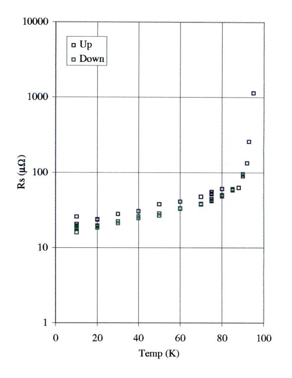
Figure 5.27:  $R_S$  for all samples at 3.7 GHz – Semi-Log Plot
