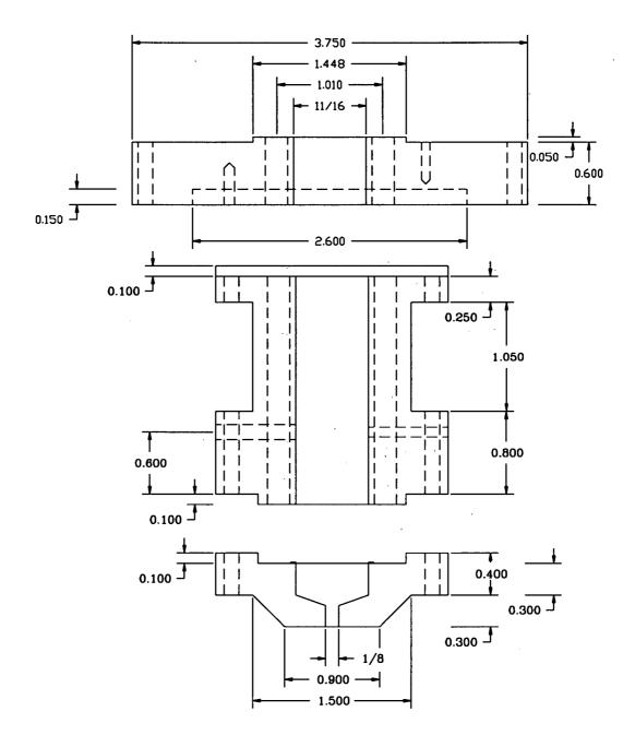
Figure 3.7: Drawing of the 3 pieces stacked together
