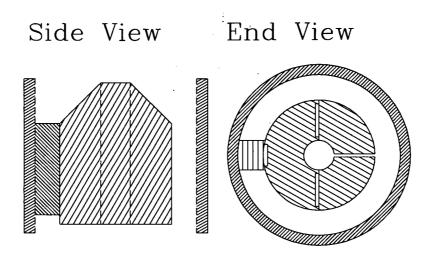
Figure 2.3: The 3.7 GHz Resonator
