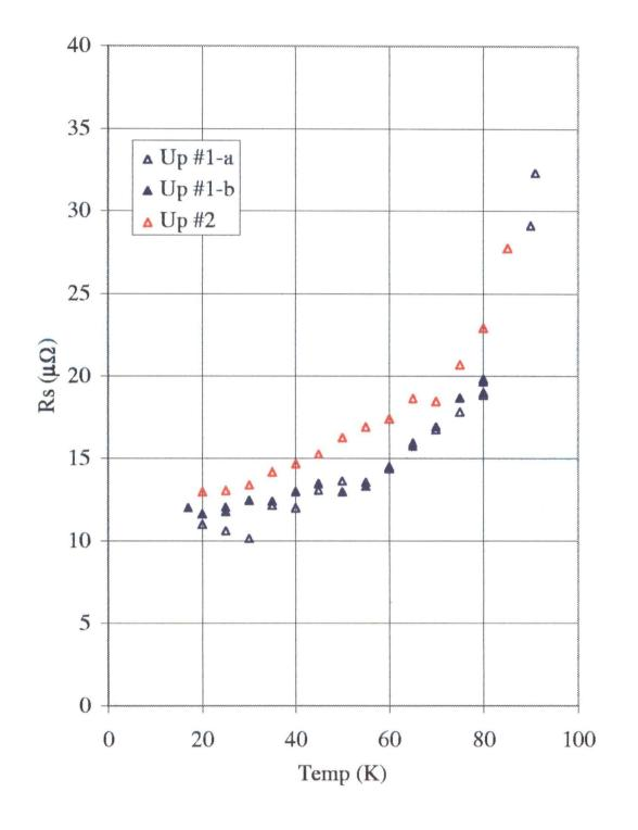
Figure 5.26:  $R_S$  for all samples at 2.4 GHz – Linear Plot
