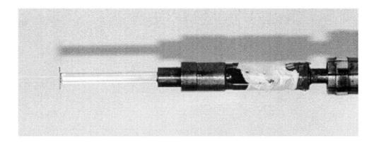
Figure 4.16: Photo of the sample holder used to position the samples near the resonator. The sample holder is also used to regulate the temperature of the sample.
