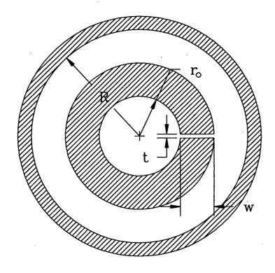
Figure 2.2: Top view of the resonator with labelling used
