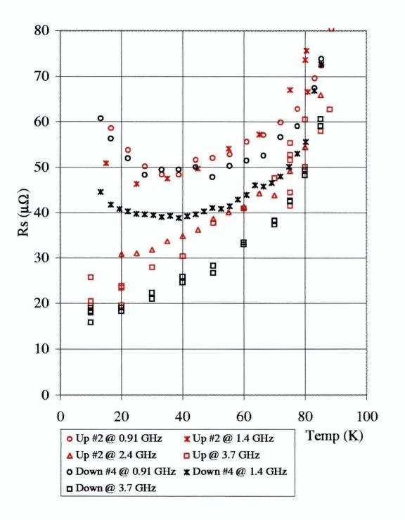
Figure 5.32:  $\omega^2$  Scaled Results for Samples #2 and #4
