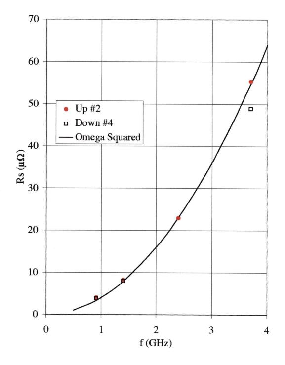
Figure 5.35: Frequency dependence of  $R_s$  at 80K. The solid line is proportional to  $\omega^2$ .
