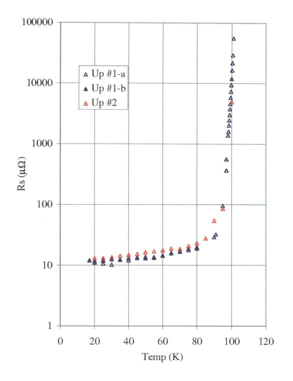
Figure 5.25:  $R_S$  for all samples at 2.4 GHz – Semi-Log Plot
