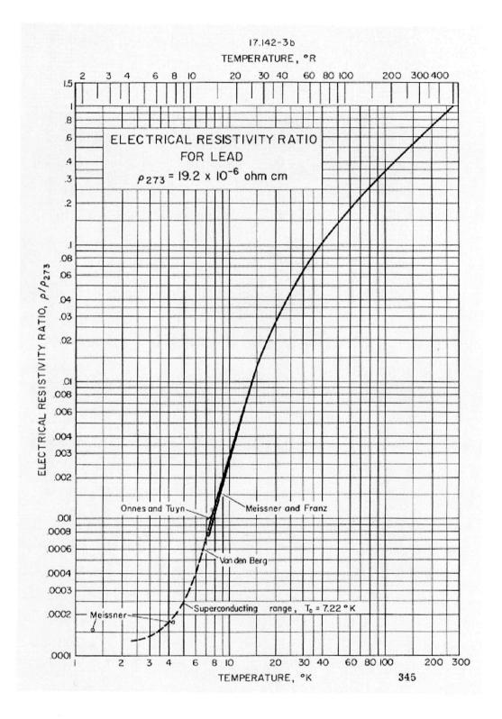
Figure A.37: DC Resistivity of Lead[19]
