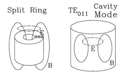
Figure 2.1: General Form of a Split Ring Resonator & a  $TE_{011}$  Cavity Mode
