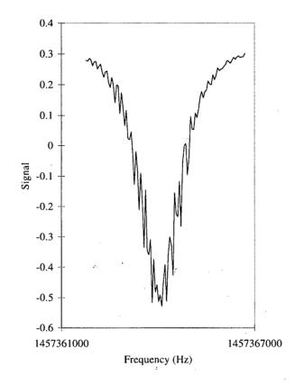
Figure 4.18: A distorted frequency domain wave form due to microphonics in the sample holder.
