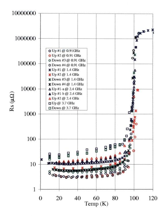
Figure 5.29:  $R_S$  for all Samples , 0–120K Semi-Log Plot
