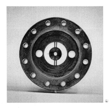
Figure 3.10: Photo of the rings in place within the core also showing the holes used by the coax. The two sapphire support posts are visible above and below the rings. Small coupling holes link the coax hole with the central shielding tube.
