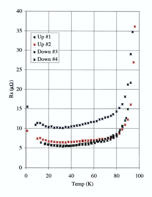
Figure 5.24:  $R_S$  for all samples at 1.4 MHz – Linear Plot. The losses for Up#1 and the temperatures for Down #4 are somewhat in question.
