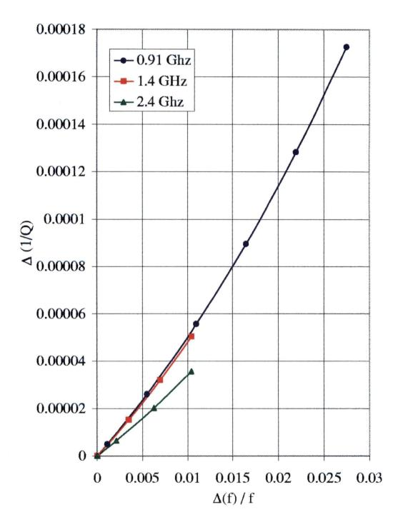
Figure 4.17: Increased losses  $\Delta(1/Q)$  as a function of the frequency change in the resonator. All data is on similar sized samples at 20 K.
