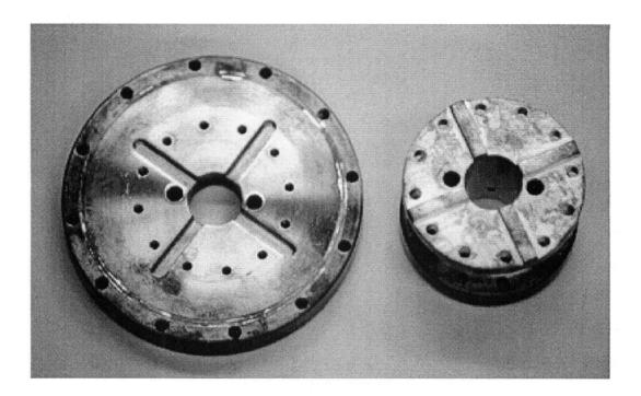
Figure 3.8: Photo of the bottom of the top plate and the top of the core of the resonator. The tongue and groove system aligns the tubes used by the coax.
