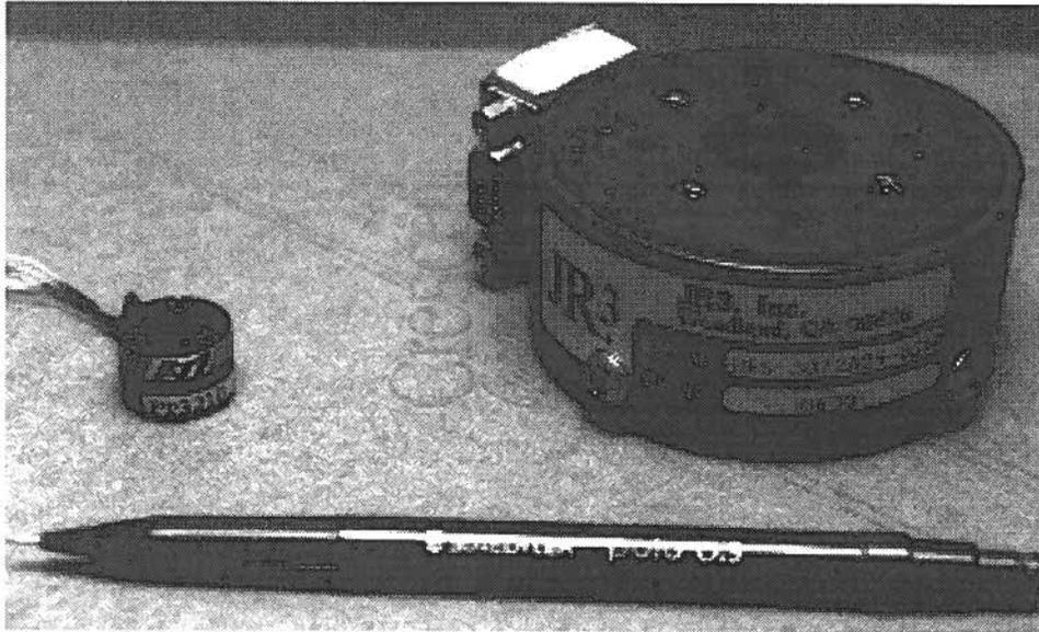
Figure 2.6: 6-DOF Force/Torque Sensors
