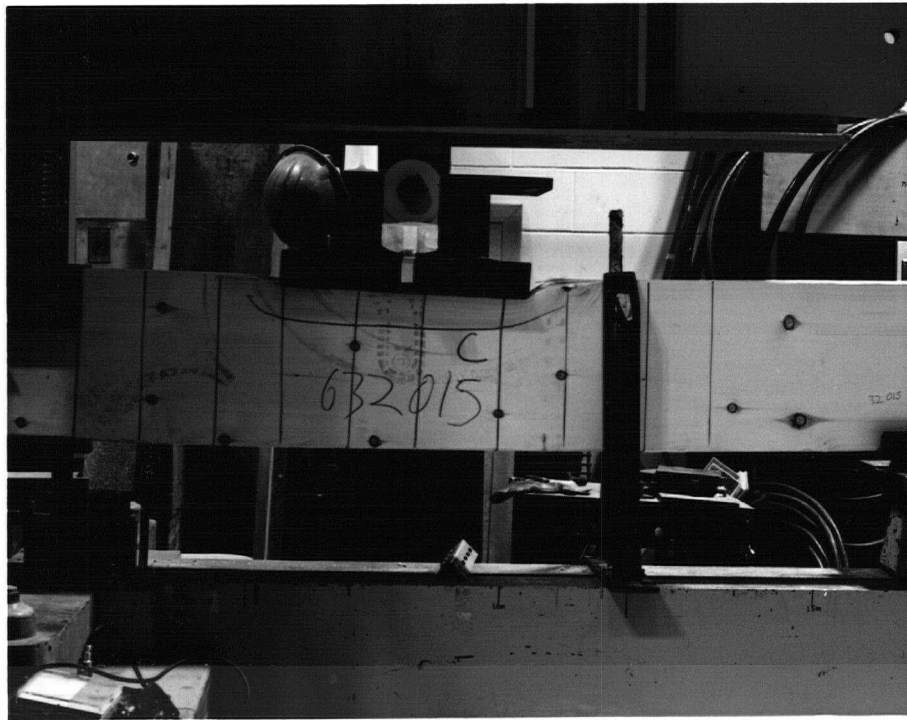
Figure 9. Different modes of failures in the two span five point bending test: (c) bending failure, (d) compression failure
