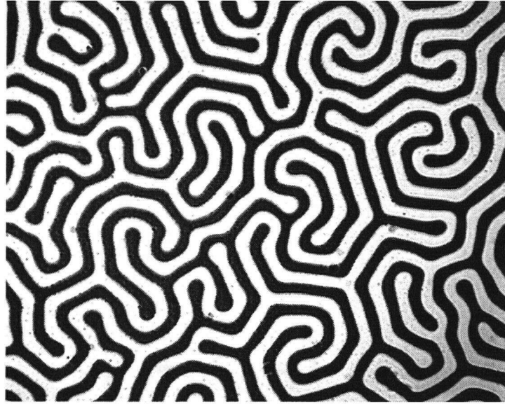
Figure 2.1: Domain structure of a bubble iron-garnet indicator film viewed under polarized light with crossed polarizers. This view is significantly magnified to resolve the domains.
