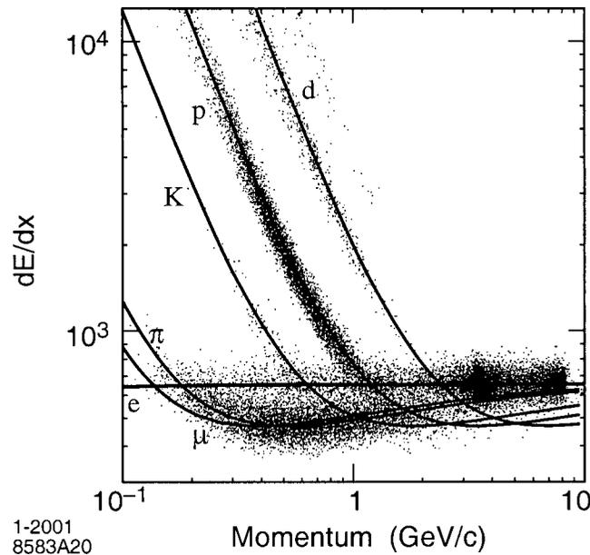
Figure 3.12: Measurements of  $dE/dx$  vs. track momenta. The data include large samples of beam background triggers, as can be seen from the high rate of protons. The superimposed curves represent Bethe-Bloch predictions for different particle species.
