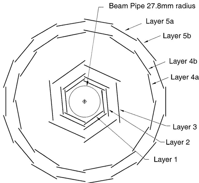
Figure 3.6: Schematic end view of the SVT.
