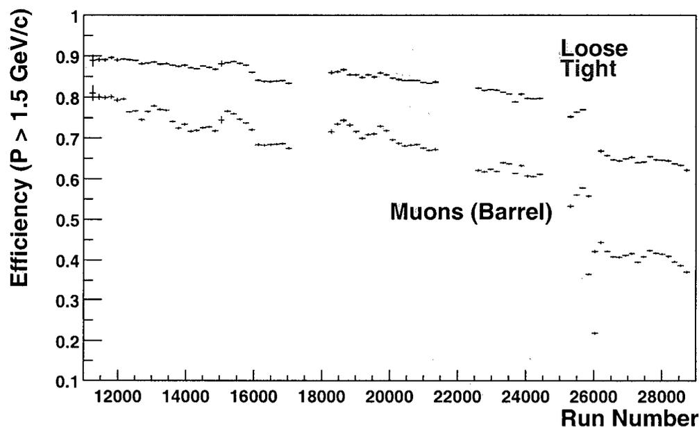
Figure 3.20: Muon detection efficiency vs. run number for data collected from 1999-2002.<sup>[34]</sup> Runs in the the 1999/2000 run period are numbered approximately 10,000 to 17,000. The labels *Loose* and *Tight* refer to the muon identification algorithms described in Section 4.2.1. The *Tight* mode (lower line) shows a worse decline, and is more important to this analysis. Around run number 26,000 there was a temporary failure in the IFR front-end electronics.
