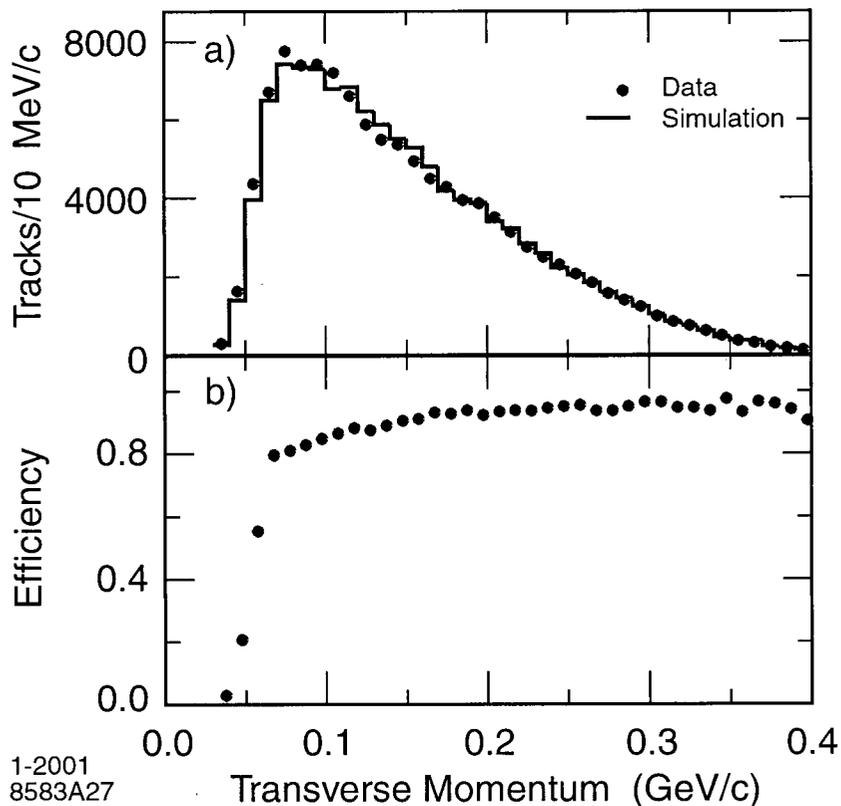
Figure 4.2: Monte Carlo studies of low momentum tracks in the SVT: a) comparison of data (contributions from combinatoric background and non- $B\bar{B}$  events have been subtracted) with simulation of the transverse momentum spectrum of pions from  $D^{*+} \rightarrow D^0\pi^+$  in  $B\bar{B}$  events, and b) efficiency for slow pion detection derived from simulated events.
