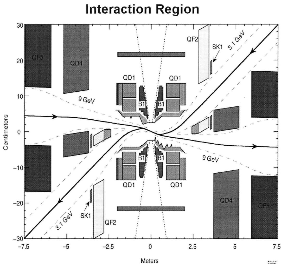
Figure 3.4: The *BABAR* interaction region. Shown are the final bending magnets (B1), focusing magnets, synchrotron radiation masks, and the HER/LER beam trajectories. Note the aspect ratio of the figure is not 1:1.
