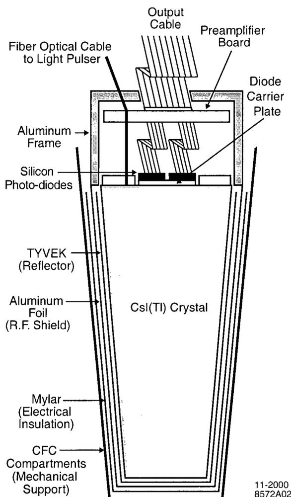
Figure 3.16: Diagram of a CsI(Tl) crystal with wrapping and readout electronics. This drawing is not to scale.
