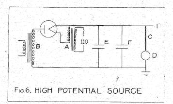
tube is heated by two oil immersion transformers, A, connected in parallel. The high voltage is produced by a 20,000 volt Thordarson transformer, B, whose primary voltage is controlled by a variac. The voltage applied to the accelerating grid of the tube is calculated from the direct current, measured by the milliamometer D, flowing through the resistance C. C consists of 24 I.R.C. resistors of 14 megohms each, enclosed in glass to precent creepage. The resistors were accurate to within 5%.
