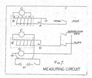
The field current from the point is directed either immediately to ground when the switch A is up, or through the galvanometer C to ground when the switch A is down. When a
