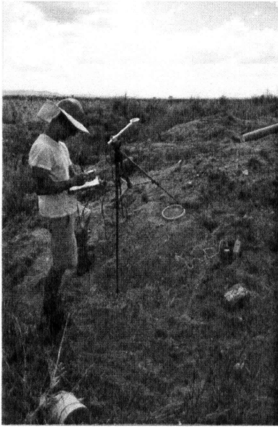
Figure 5.7: Tripod-mounted net radiometer for spot measurements
