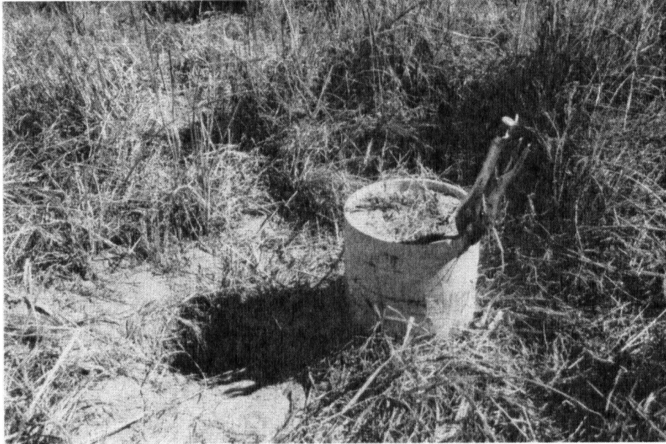
Figure 5.10: Microlysimeter used at Kidston
