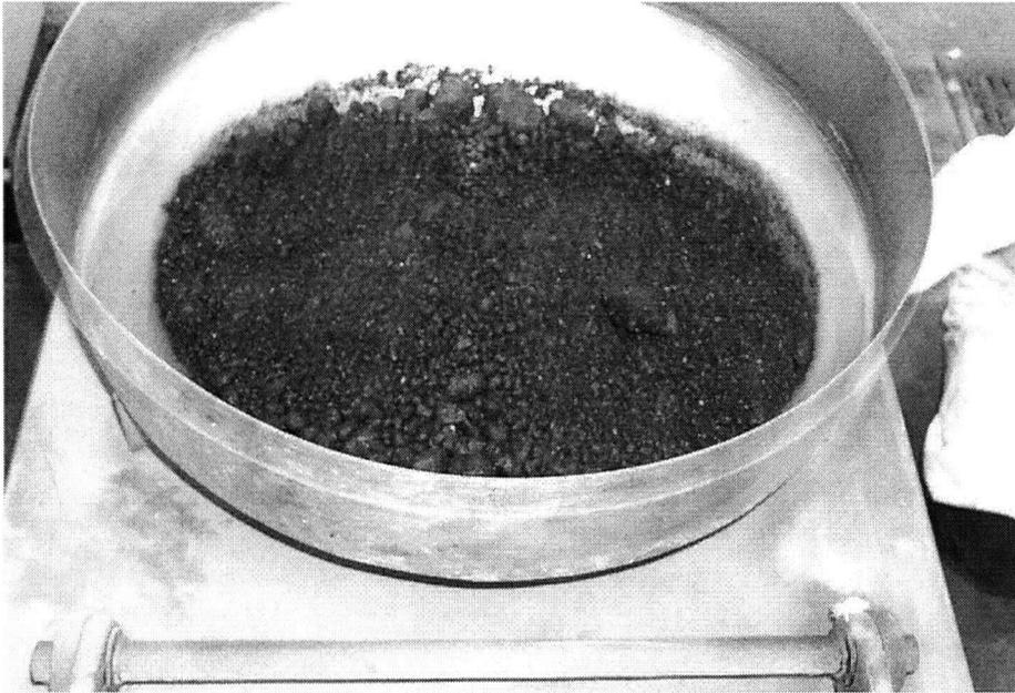
Figure G.5-3 Segregation effects during Durham Cone tests – emptying.
