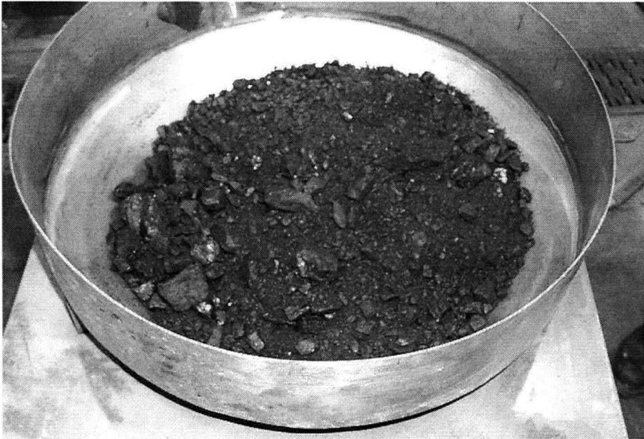
Figure G.5-1 Segregation effects during Durham Cone tests - initial seconds of conditioning.
