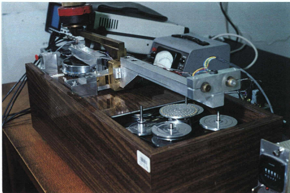
Figure 5.4 Stepper motor arrangement for dynamic loading
