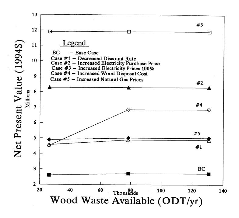
Figure 29: Net Present Value for Option #3 with a Process Heat Requirement of 20,000 kW
