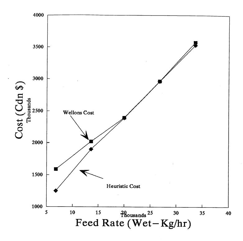
Figure 5: Wood Waste Furnace/Combustor Cost vs Wood Fuel Feed Rate
