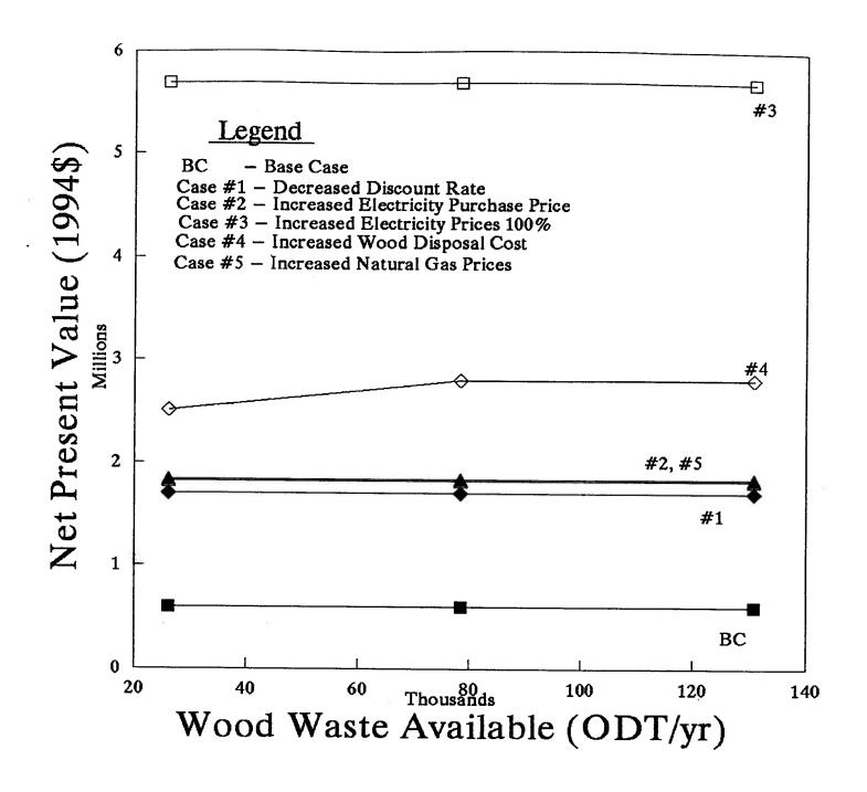
Figure 27: Net Present Value for Option #3 with a Process Heat Requirement of 10,000 kW
