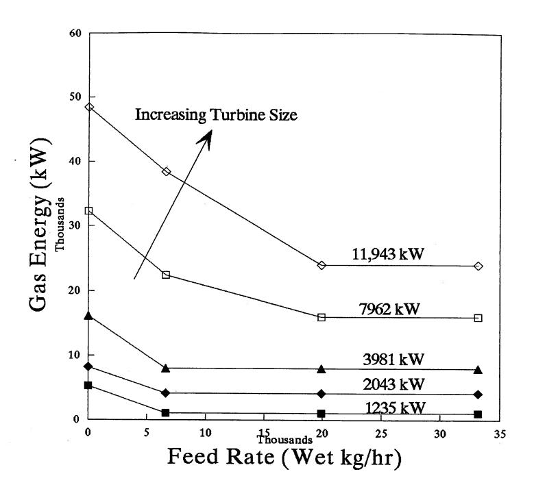
Figure 13: Natural Gas Consumption Required For Top-Up of Turbine Inlet Temperature For Option #3
