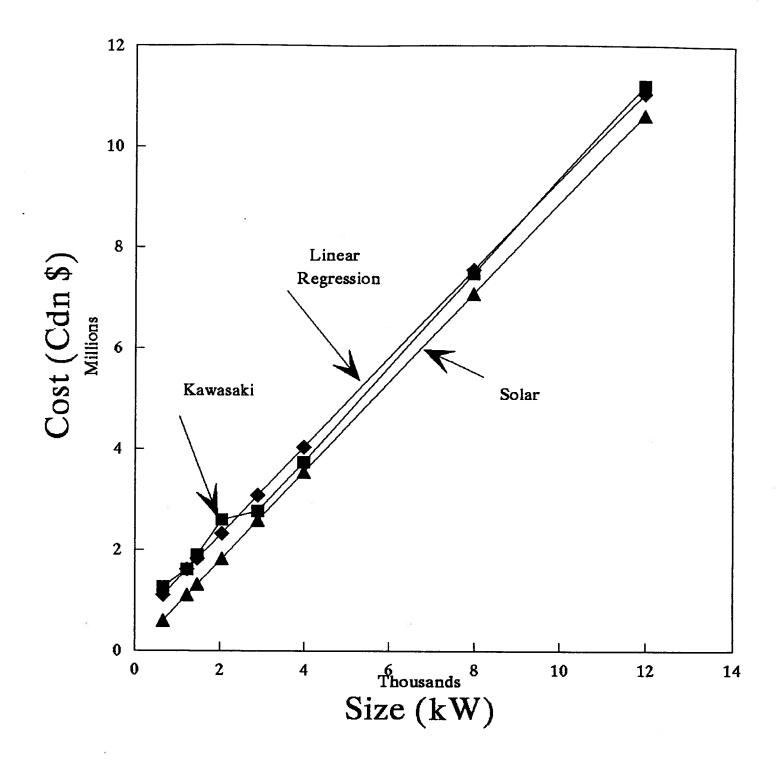
Figure 4: Gas Turbine Cost as a Function of Size
