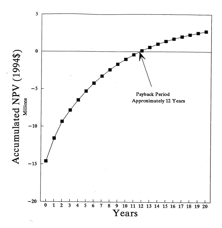
Figure 37: Option #3 Payback Period for a Sawmill Producing 80,000 ODT/yr of Wood Waste and Requiring 20,000 kW of Process Heat
