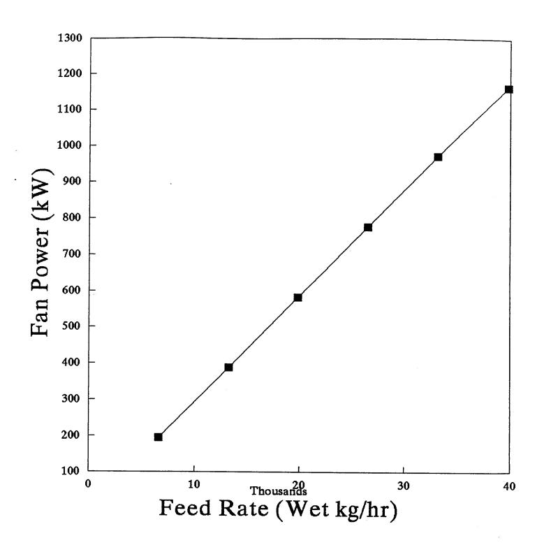
Figure 17: Fan Power Required vs Wood Fuel Feed Rate Into System For Option #3
