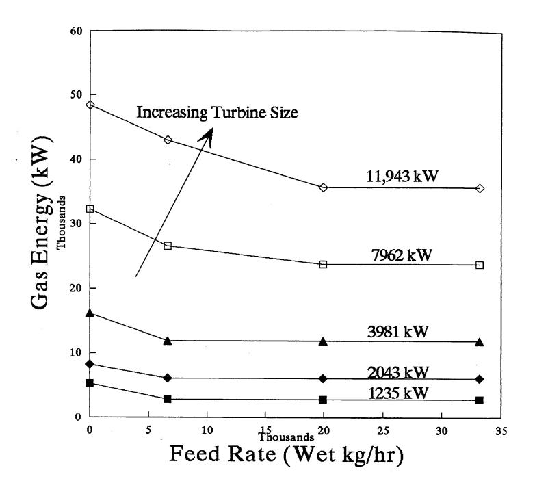
Figure 12: Natural Gas Consumption Required For Top-Up of Turbine Inlet Temperature For Option #1
