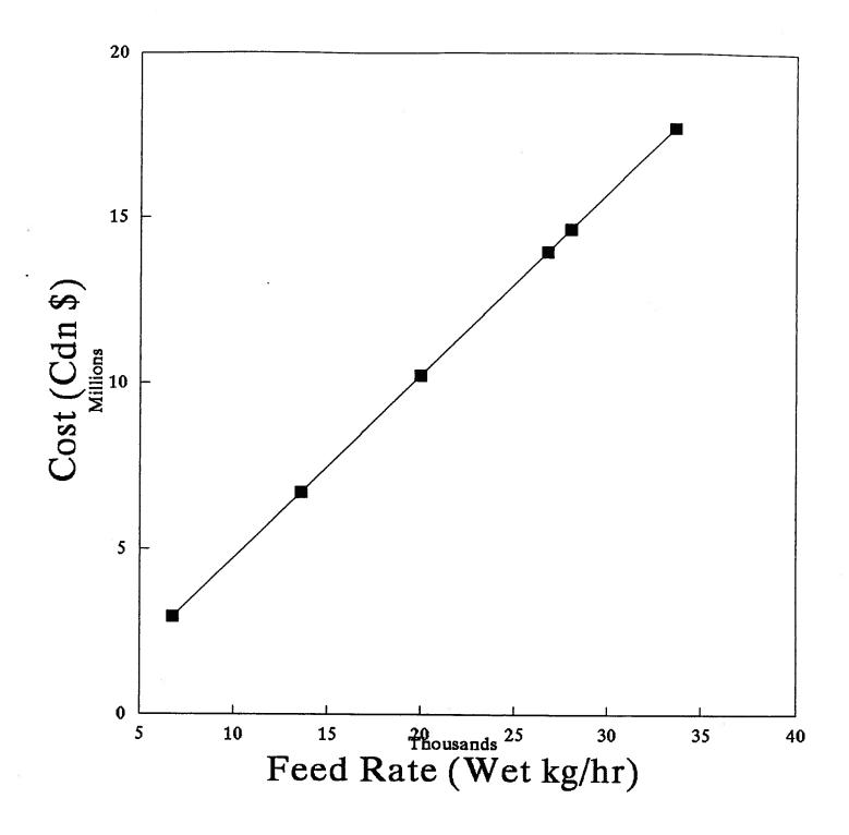
Figure 8: ABB System Cost as a Function of Wood Fuel Feed Rate
