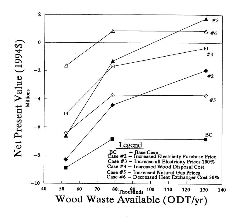
Figure 25: Net Present Value for Option #2 with a Process Heat Requirement of 20,000 kW
