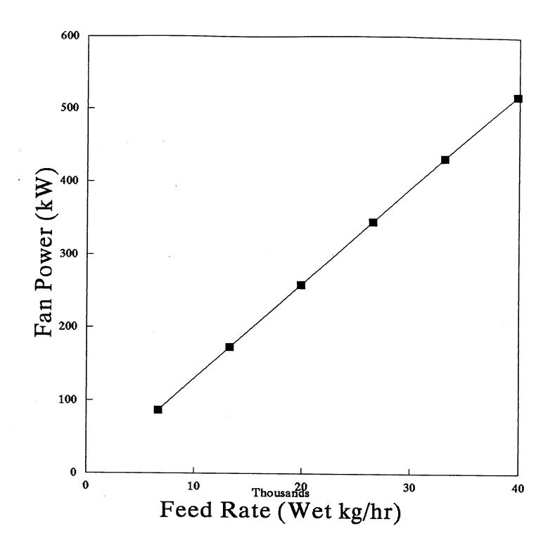
Figure 15: Fan Power Required vs Wood Fuel Feed Rate Into System For Option #1
