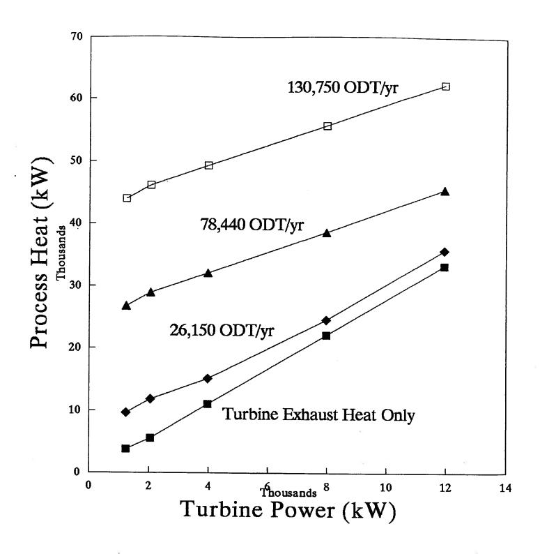
Figure 9: Process Heat Generated as a Function of Turbine Power and Wood Waste Availability For Option #1
