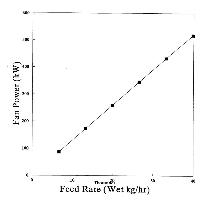
Figure 16: Fan Power Required vs Wood Fuel Feed Rate Into System For Option #2
