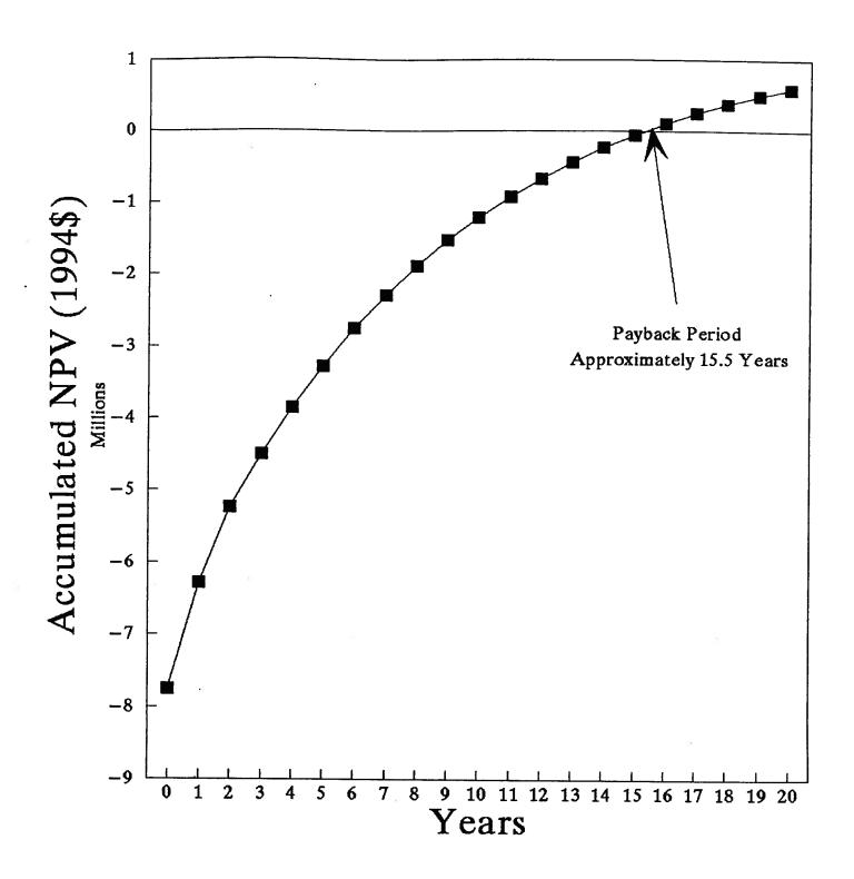
Figure 36: Option #3 Payback Period for a Sawmill Producing 80,000 ODT/yr of Wood Waste and Requiring 10,000 kW of Process Heat
