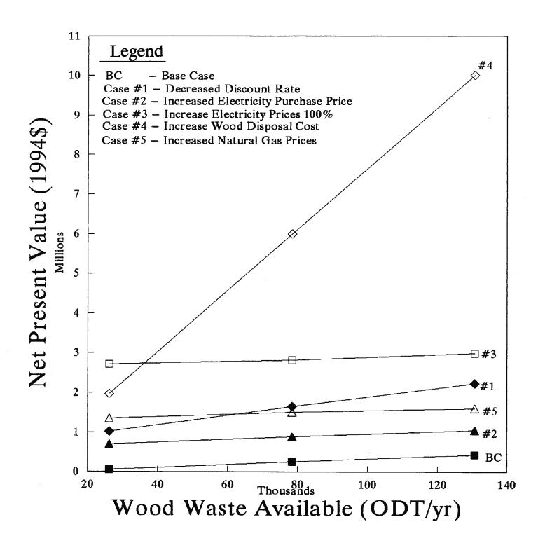
Figure 19: Net Present Value for Option #1 with a Process
