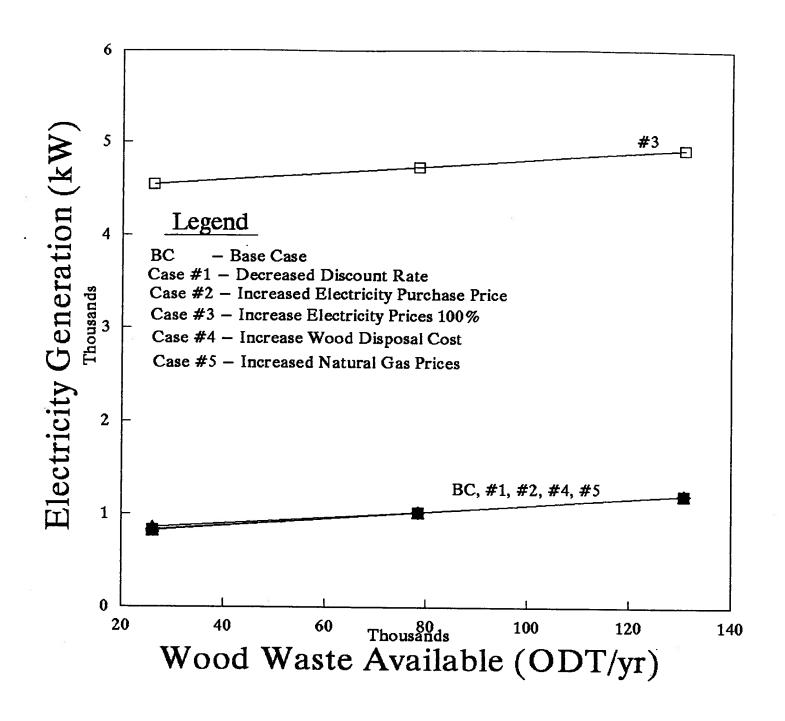
Figure 18: Optimum Electricity Generation for Option #1 with a Process Heat Requirement of 10,000 kW
