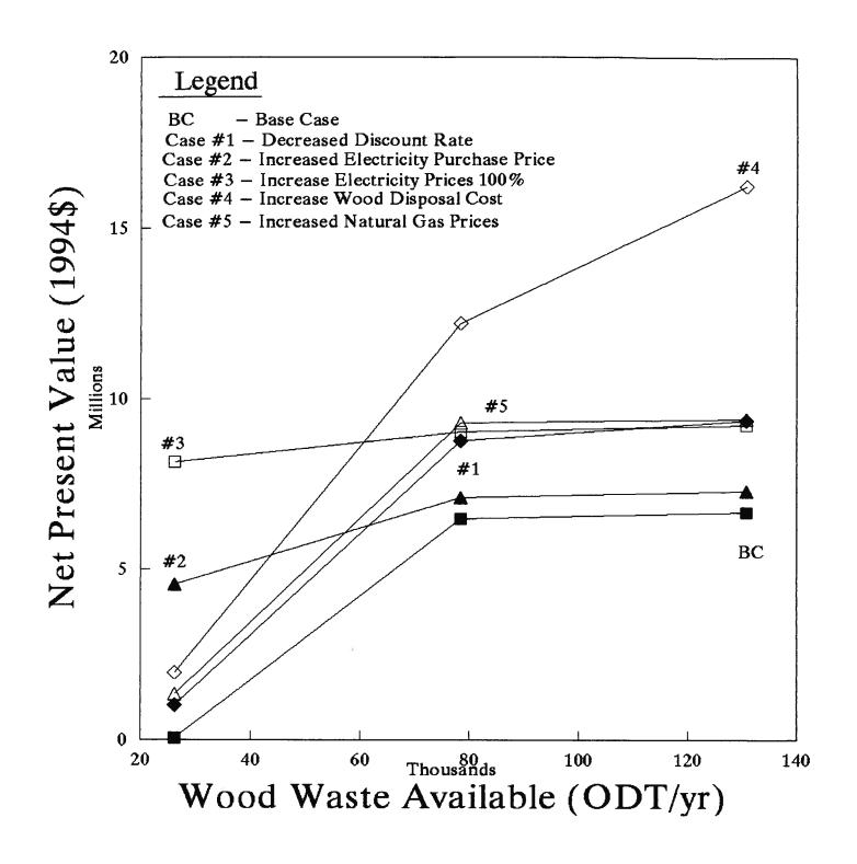
Figure 21: Net Present Value for Option #1 with a Process Heat Requirement of 20,000 kW
