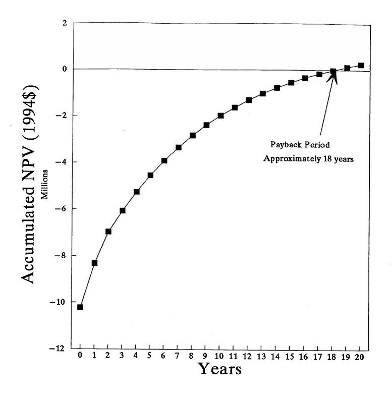
Figure 32: Option #1 Payback Period for a Sawmill Producing 80,000 ODT/yr of Wood Waste and Requiring 10,000 kW of Process Heat
