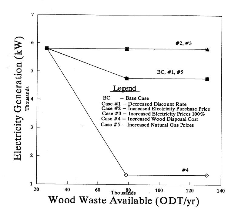
Figure 28: Optimum Electricity Generation for Option #3 with a Process Heat Requirement of 20,000 kW
