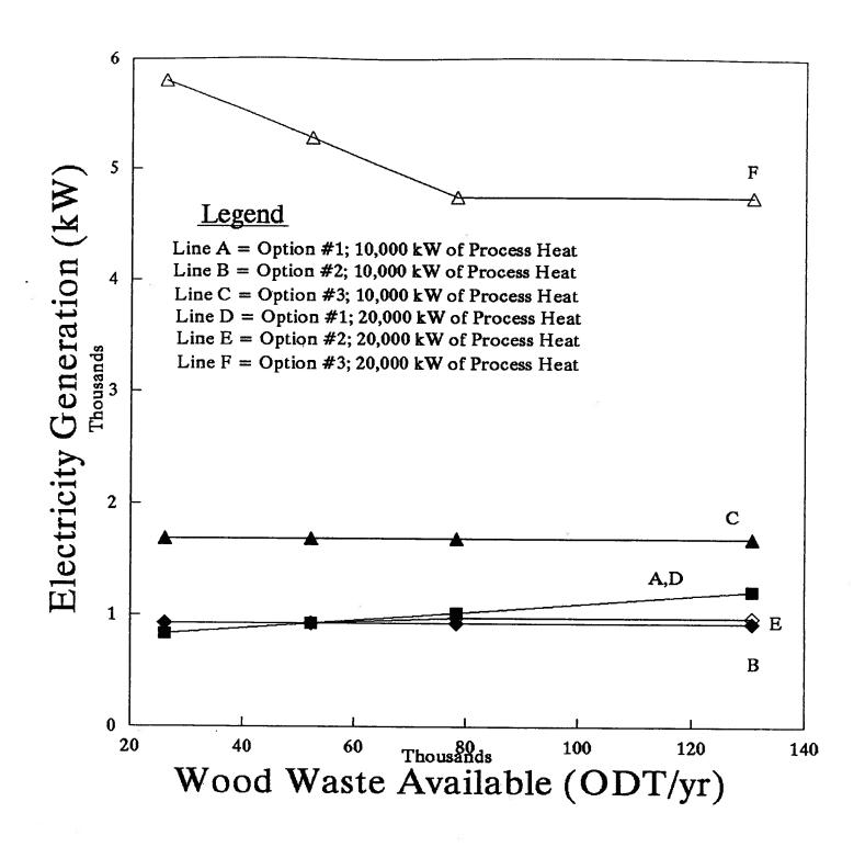
Figure 30: Comparison of the Optimum Electricity Generation for the Base Case Results for Options #1, #2, #3
