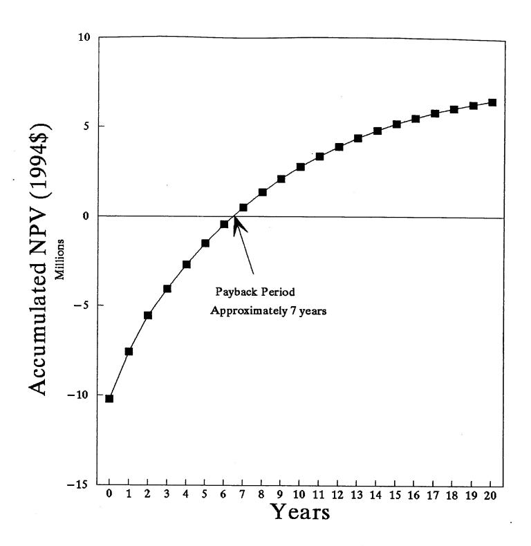
Figure 33: Option #1 Payback Period for a Sawmill Producing 80,000 ODT/yr of Wood Waste and Requiring 20,000 kW of Process Heat
