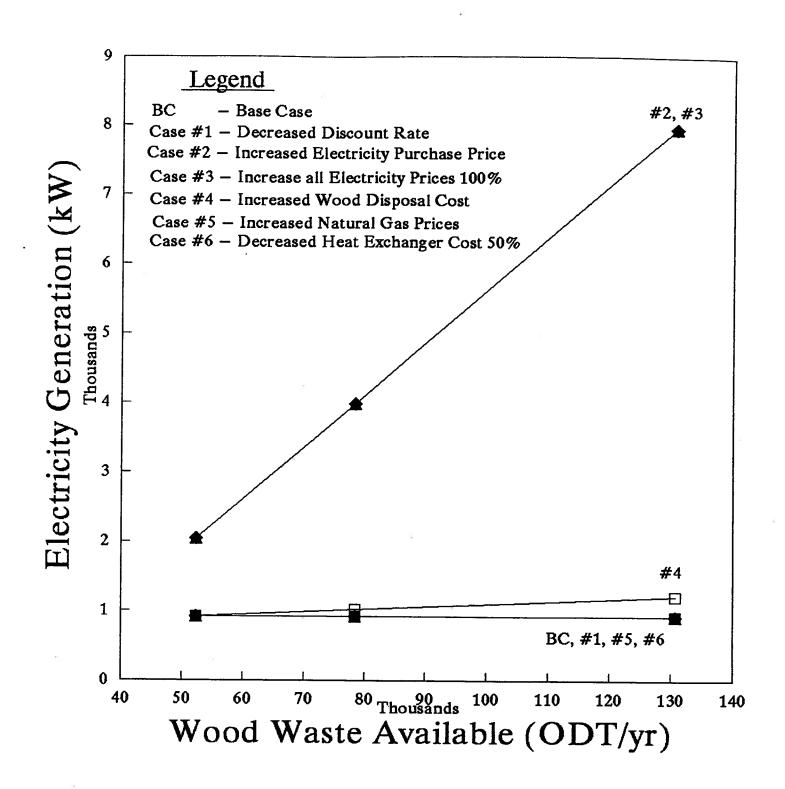
Figure 22: Optimum Electricity Generation for Option #2 with a Process Heat Requirement of 10,000 kW
