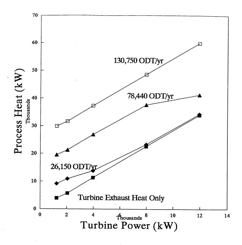
Figure 11: Process Heat Generated as a Function of Turbine Power and Wood Waste Availability For Option #3
