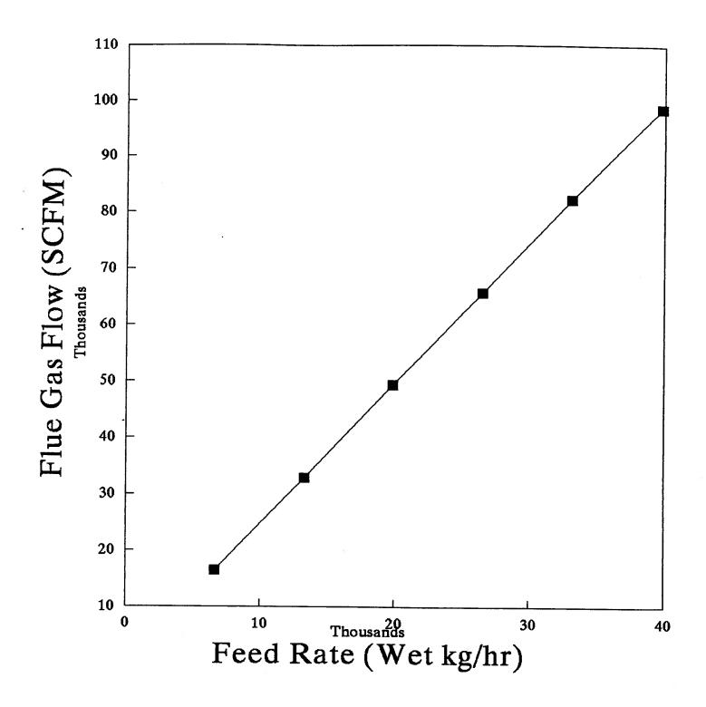
Figure 14: Rate of Flue Gas Production vs Wood Fuel Feed Rate Into System
