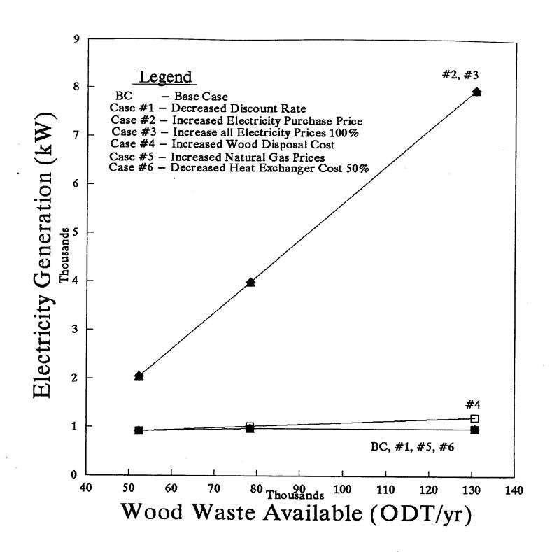
Figure 24: Optimum Electricity Generation for Option #2 with a Process Heat Requirement of 20,000 kW
