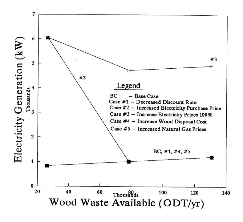
Figure 20: Optimum Electricity Generation for Option #1 with a Process Heat Requirement of 20,000 kW
