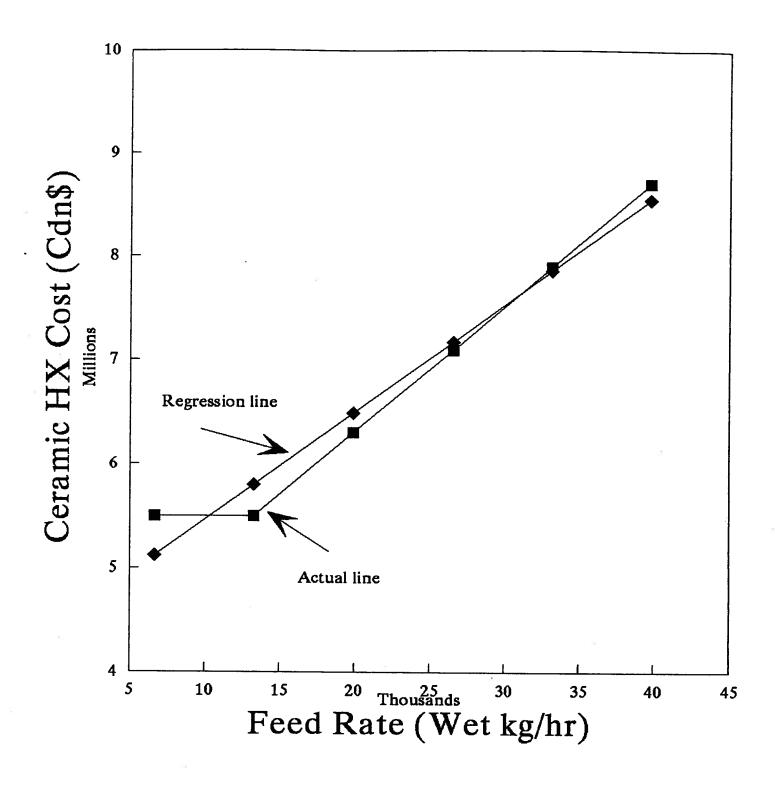
Figure 7: Ceramic Heat Exchanger Cost vs Wood Fuel Feed Rate
