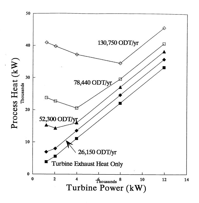
Figure 10: Process Heat Generated as a Function of Turbine Power and Wood Waste Availability For Option #2
