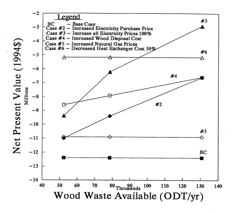
Figure 23: Net Present Value for Option #2 with a Process Heat Requirement of 10,000 kW
