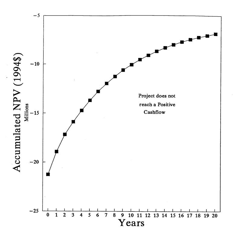
Figure 35: Option #2 Payback Period for a Sawmill Producing 80,000 ODT/yr of Wood Waste and Requiring 20,000 kW of Process Heat
