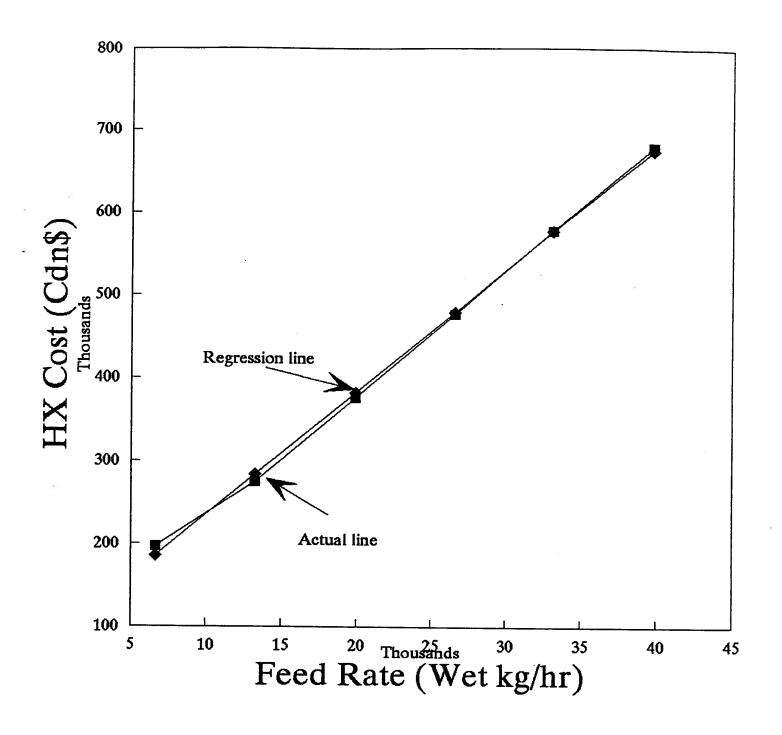
Figure 6: Metal Heat Exchanger Cost vs Wood Fuel Feed Rate
