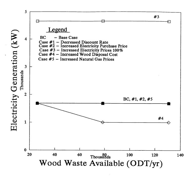
Figure 26: Optimum Electricity Generation for Option #3 with a Process Heat Requirement of 10,000 kW
