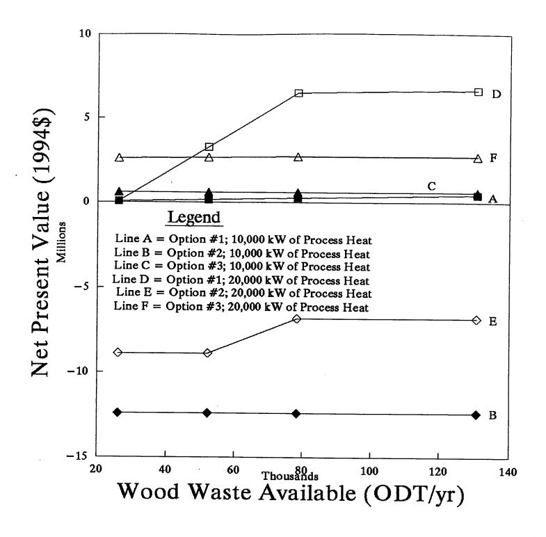
Figure 31: Comparison of the Net Present Value for the Base Case Results for Options #1, #2, #3
