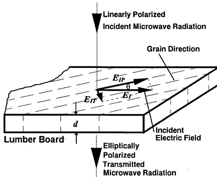
Figure 2-2 Microwave Field Transmission through Wood
