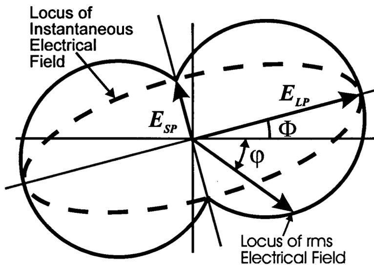
Figure 3-2 Locus of the Instantaneous Electrical Field and  $k|\mathbf{E} \cdot \mathbf{u}|$  Measured from a Dipole
