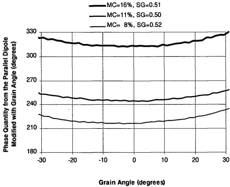
Fig. 6-6 Phase Quantity  $\bar{P}$  Calculated with the Actual Grain Angle for a Range of Moisture Content
