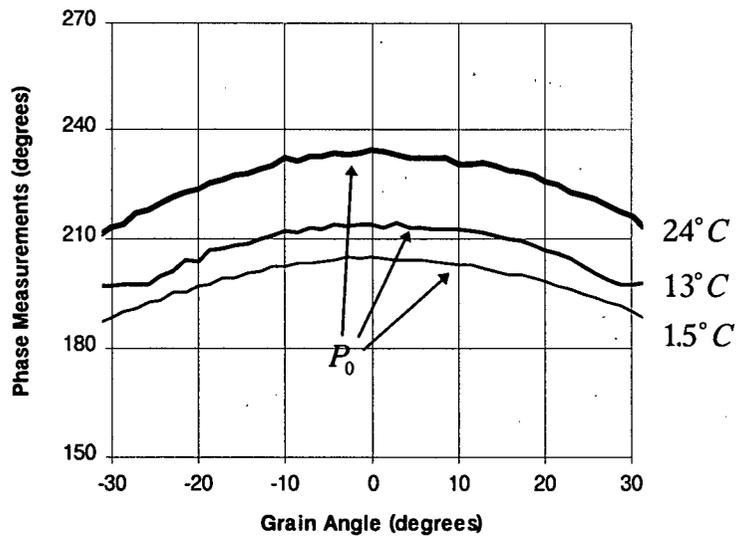
Fig. 7-1 Microwave Measurements vs. Temperature
