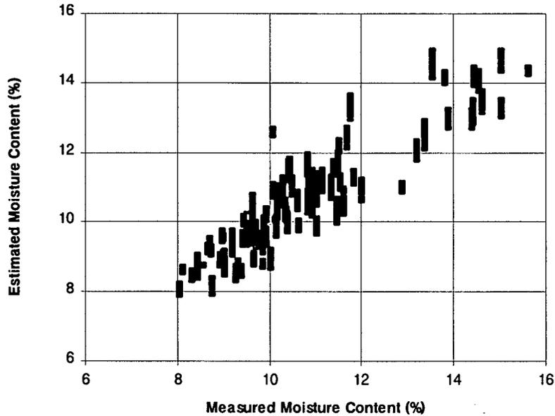
Fig. 6-10 Moisture Content Determined from Equation (6-18) Using Microwave Measurements vs. Gravimetrically Measured Moisture Content
