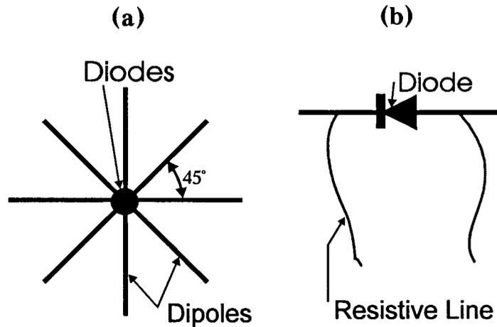
Figure 3-3 Schematic of the New Microwave Probe
