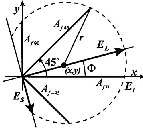
Figure 3-4 Geometric Representation of Measurements from the Probe's Four Dipoles and the Field Vectors
