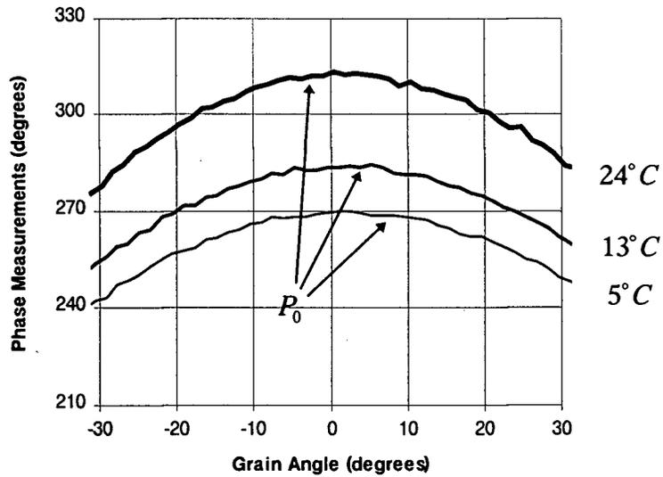
Fig. 7-2 Microwave Measurements vs. Temperature
