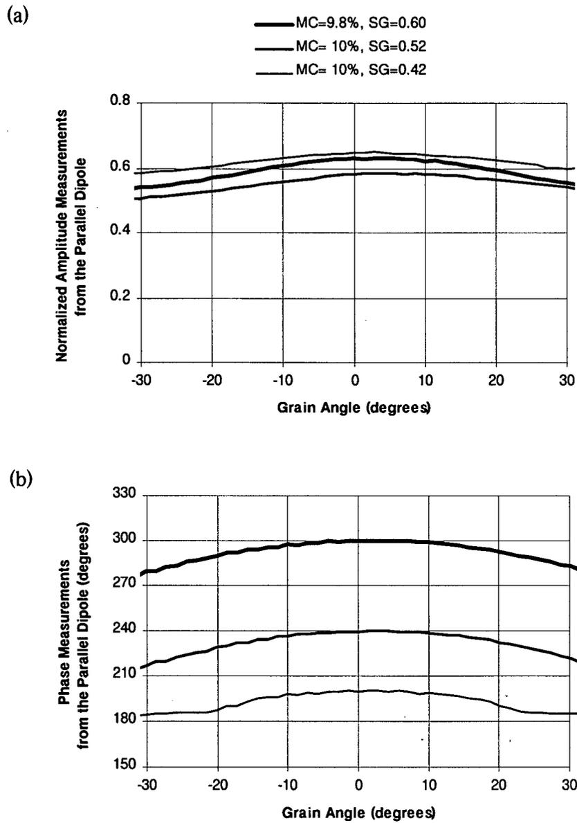
Fig. 6-3 Microwave Measurements vs. Grain Angle
