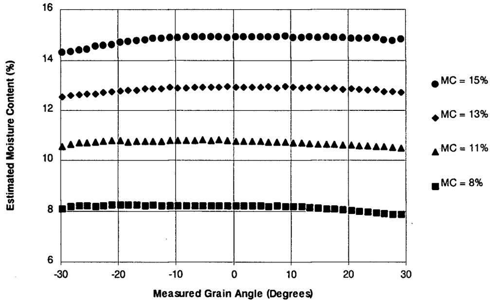
Fig. 6-11 Estimated Moisture Content vs. Grain Angle
