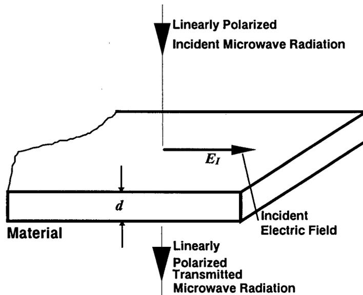
Figure 2-1 Microwave Field Transmission through Isotropic Material
