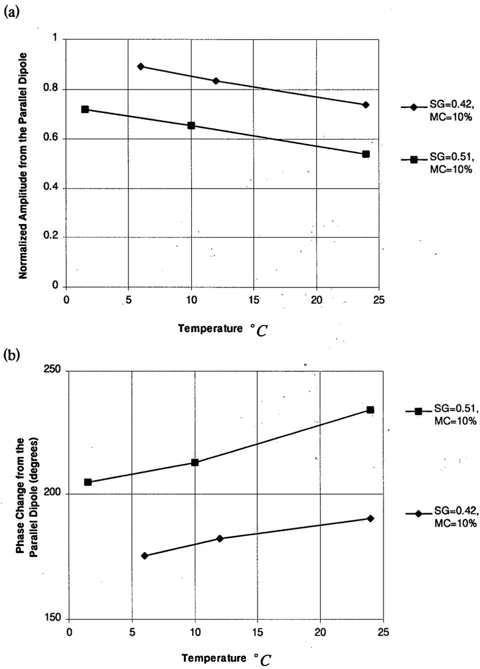
Fig. 7-6 Microwave Measurements at 0° Grain Angle vs. Temperature with Different Specific Gravity Douglas-fir Sample:  $SG = 0.42$  and  $0.51$ ,  $MC = 10\%$
