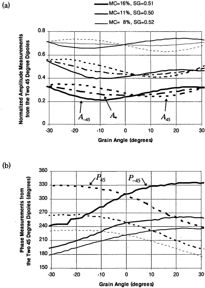
Fig. 6-2 Microwave Measurements vs. Grain Angle
