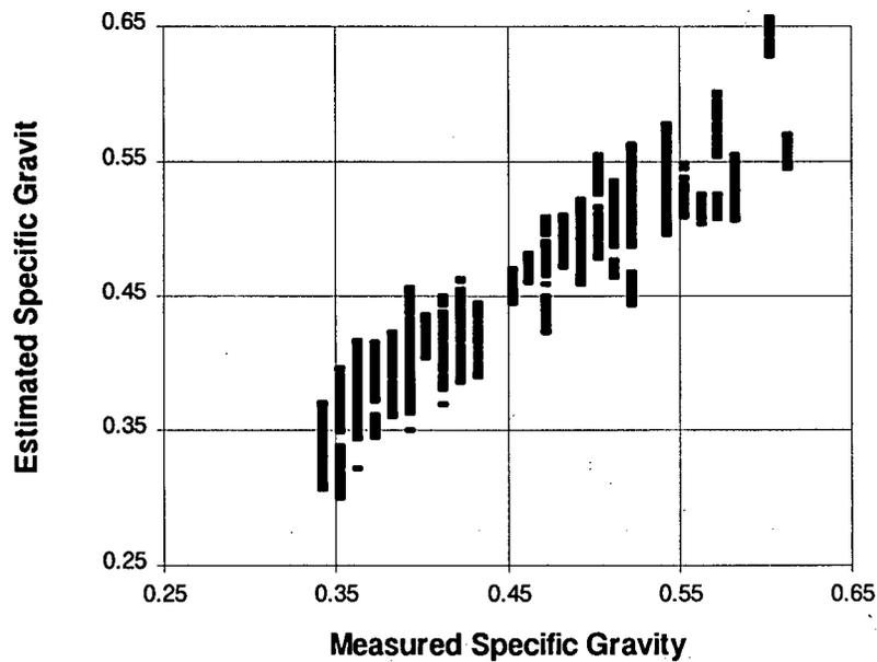
Fig. 6-8 Specific Gravity Determined from Equation (6-11) Using Microwave Measurements vs. Gravimetrically Measured Specific Gravity
