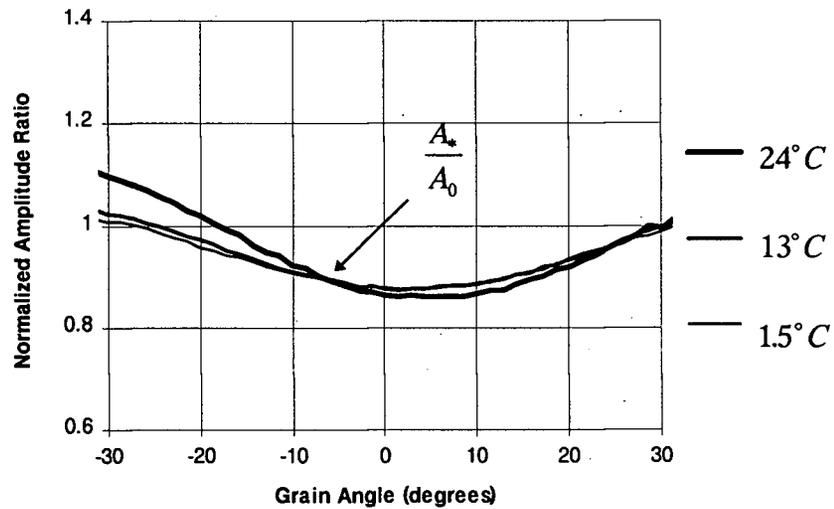
Fig. 7-4 Microwave Amplitude Ratio,  $A_*/A_0$ , vs. Temperature
