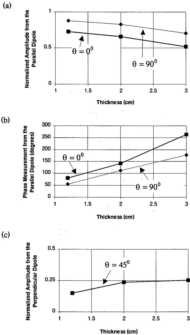
Fig. 4-6 Specimen Thickness Effect in Microwave Amplitude and Phase Measurements from Matched Douglas-fir Specimens
