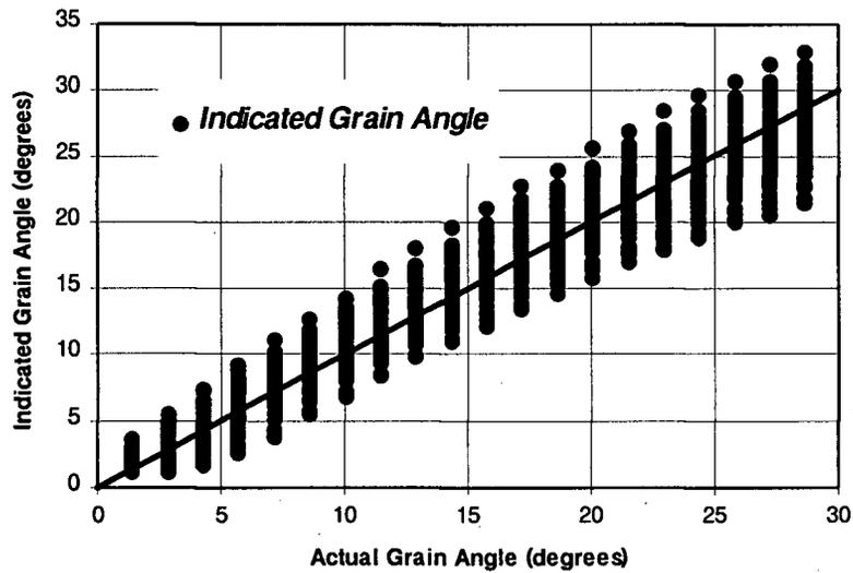
Fig. 5-3 Positive Grain Angle Identification Using the Amplitude Measurement from the Perpendicular Dipole with Equation (5-14)
