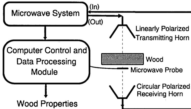
Figure 3-1 Schematic of the Wood Property Measurement System
