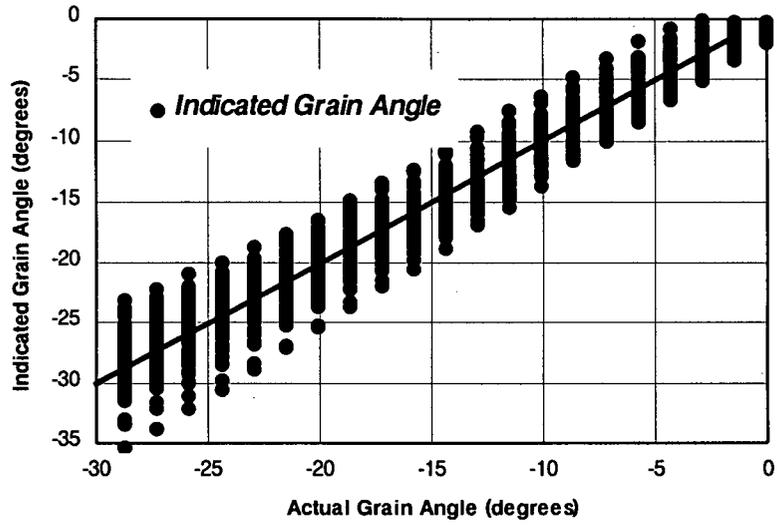
Fig. 5-4 Negative Grain Angle Identification Using the Amplitude Measurements from all Dipoles with Equation (5-16)
