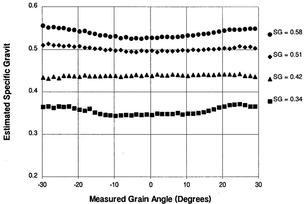
Fig. 6-9 Estimated Specific Gravity vs. Grain Angle
