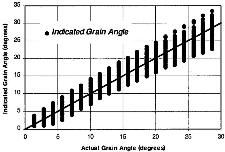
Fig. 5-5 Positive Grain Angle Identification Using the Amplitude Measurements from all Dipoles with Equation (5-17)
