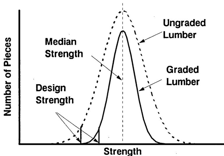
Figure 1-1 Strength Variation within a Batch of Lumber
