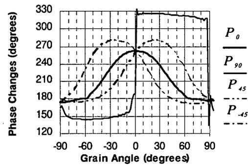
Fig. 4-5 Specimen Thickness Effect in Microwave Amplitude and Phase Measurements from Matched Douglas-fir Specimens
