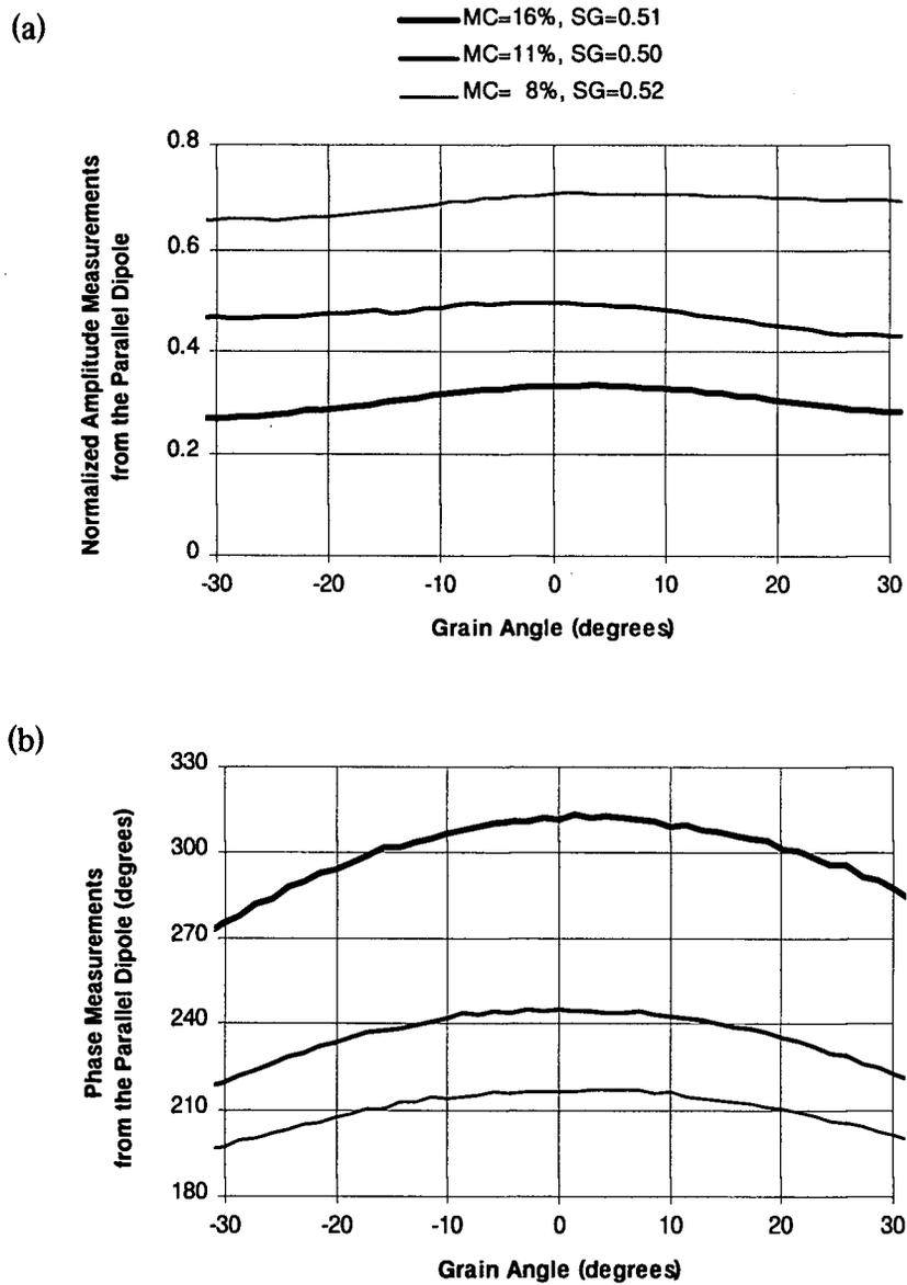
Fig. 6-1 Microwave Measurements vs. Grain Angle
