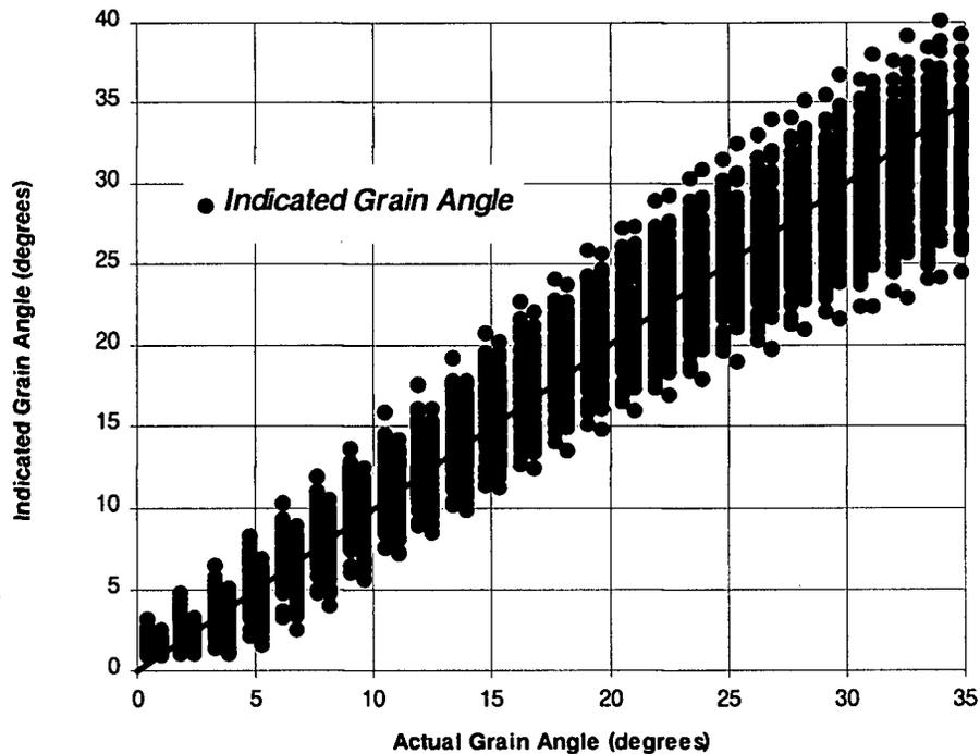
Fig. 5-1 Grain Angle Identification Using the Amplitude Measurement of the Perpendicular Dipole  $A_{90}$  with Equation (5-10)
