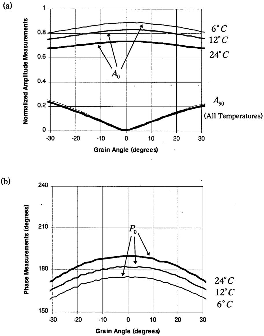
Fig. 7-3 Microwave Measurements vs. Temperature
