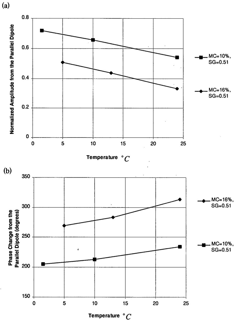
Fig. 7-5 Microwave Measurements at 0° Grain Angle vs. Temperature with Different Moisture Content Douglas-fir Sample:  $SG = 0.51$ ,  $MC = 10\%$  and  $16\%$
