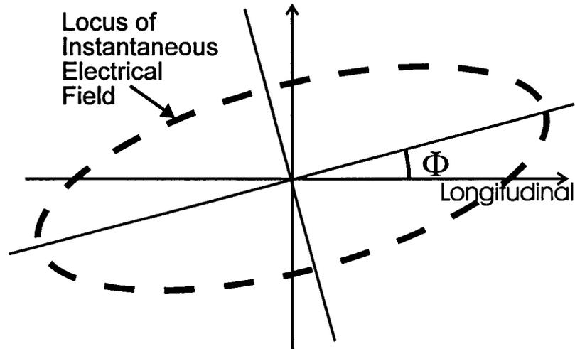
Figure 2-3 Elliptical Polarization
