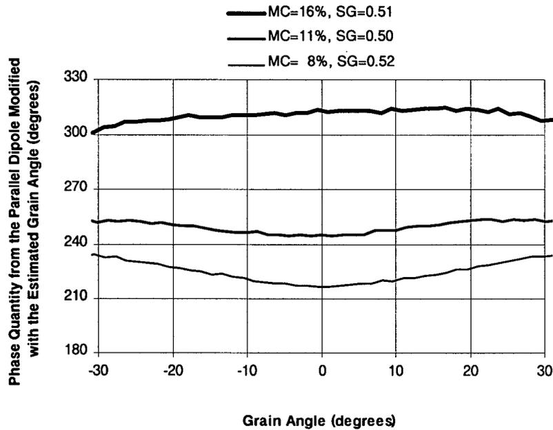
Fig. 6-7 Phase Quantity  $\bar{P}$  Calculated with the Estimated Grain Angle for a Range of Moisture Content
