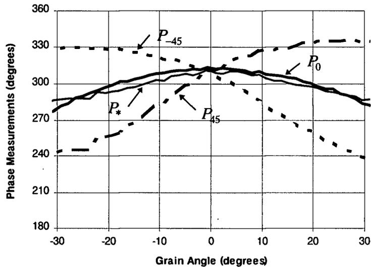
Fig. 6-5 Microwave Phase Measurements vs. Grain Angle for a Range of Moisture Content
