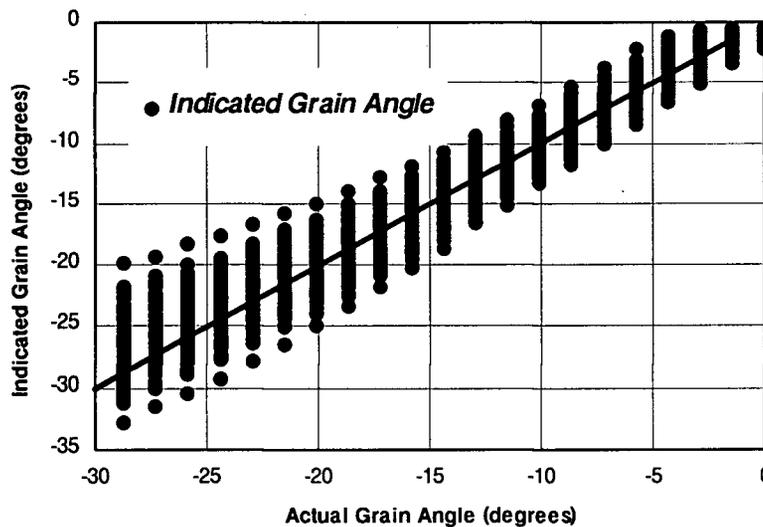
Fig. 5-2 Negative Grain Angle Identification Using the Amplitude Measurement from the Perpendicular Dipole with Equation (5-13)
