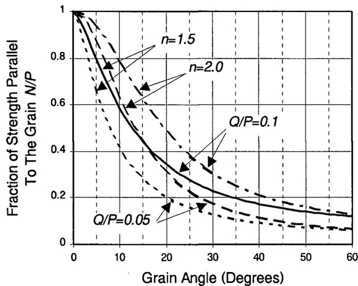
Figure 1-3 Effect of Grain Angle on Strength
