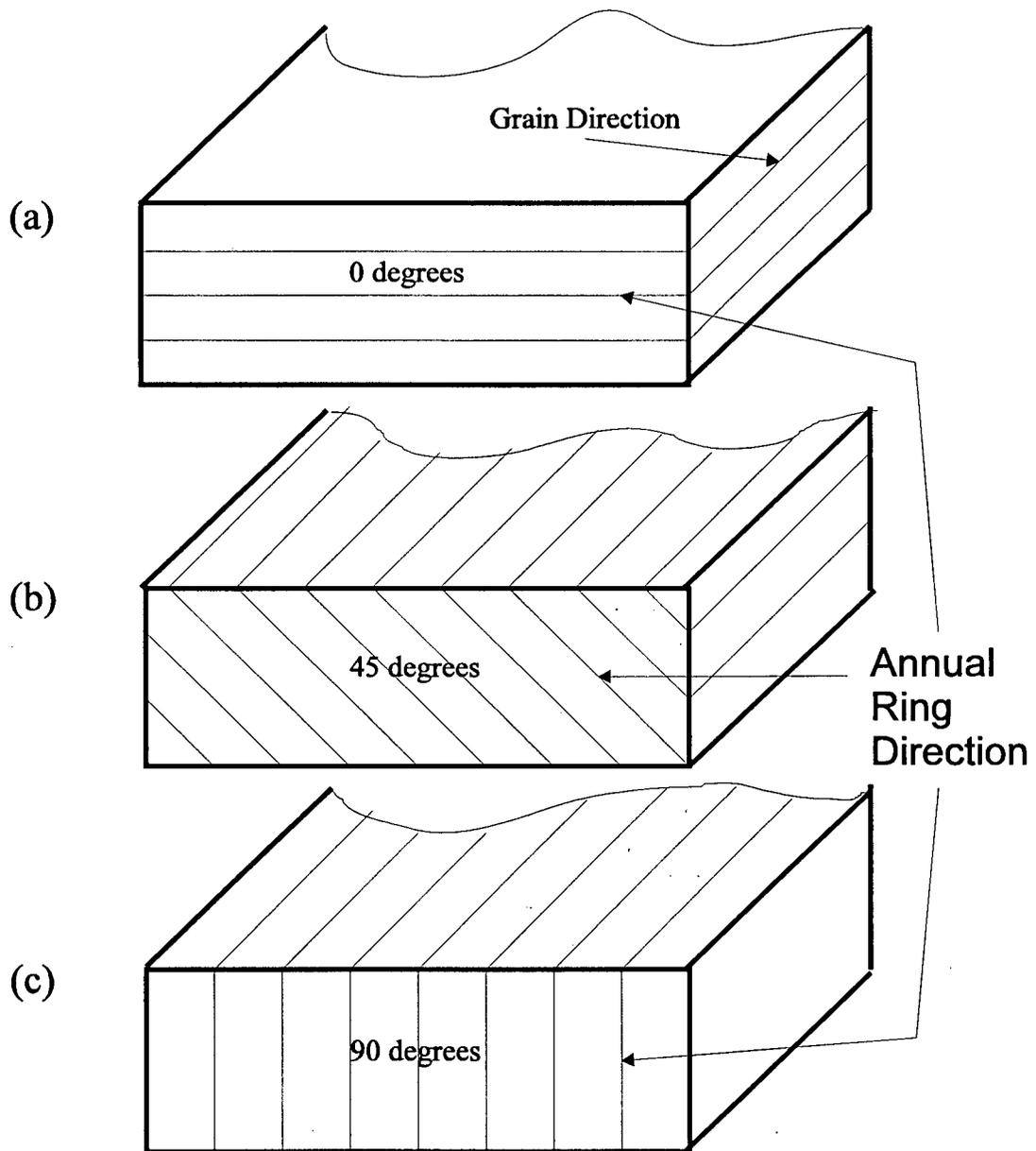
Fig. 4-1 Sketch of Cross Sections of Samples with Different Annual Ring Direction
