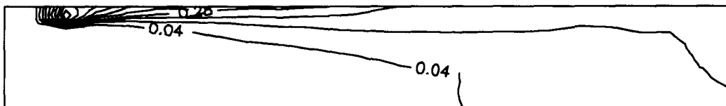
Figure 6.3.3 Concentration fields for cases 8 and 10 showing pressure ratio effects, jet angle 10 deg., engine speed 1200 RPM, contour interval 0.08 (kg/kg), injector tip in top left corners.
