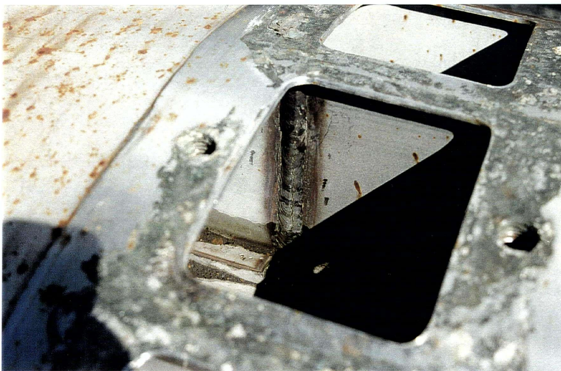
Figure 1.5 Severe Cracking through the Core Pipe Division Bar
