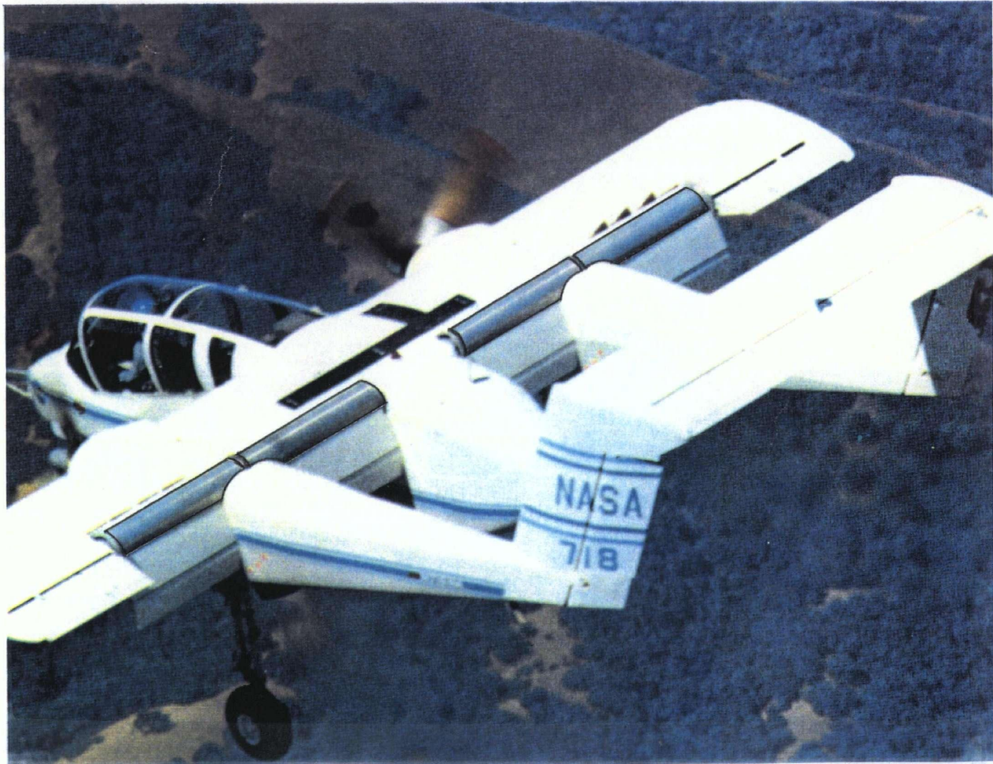
Figure 1-5 The North American Rockwell OV-10A aircraft in flight demonstrating a successful application of the rotating cylinder as a high-lift device.
