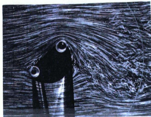
Figure 4-12 Flow visualization photographs showing effectiveness of the Moving Surface Boundary-layer Control (MSBC) as applied to the D-section. Note, at U_C/U = 4 , the fluid motion tends to approach the potential character.
