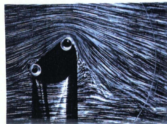
Figure 4-12 Flow visualization photographs showing effectiveness of the Moving Surface Boundary-layer Control (MSBC) as applied to the D-section. Note, at U_C/U = 4 , the fluid motion tends to approach the potential character.
