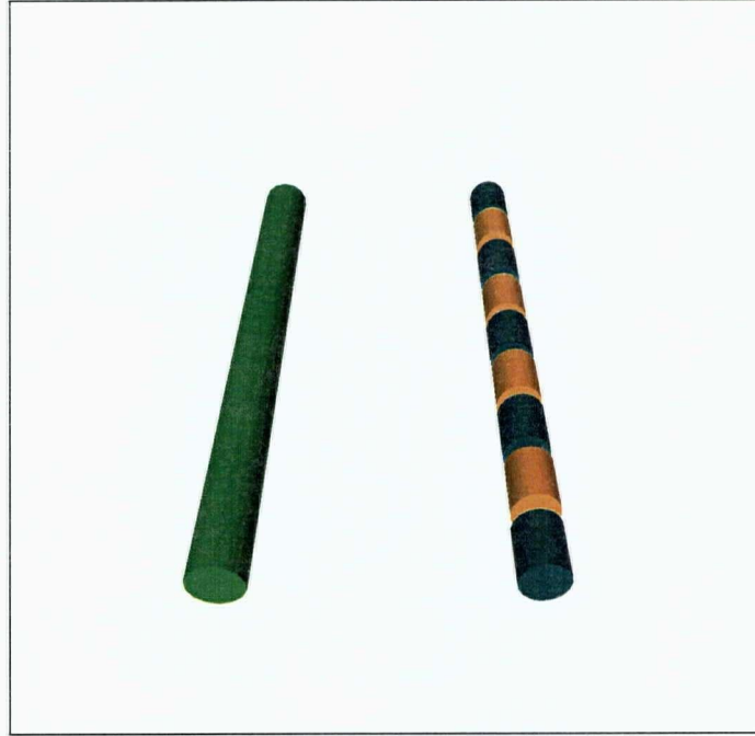
Figure 2.8: Schematic diagram of a continuous fibre and its representation by a series of cylindrical elements
