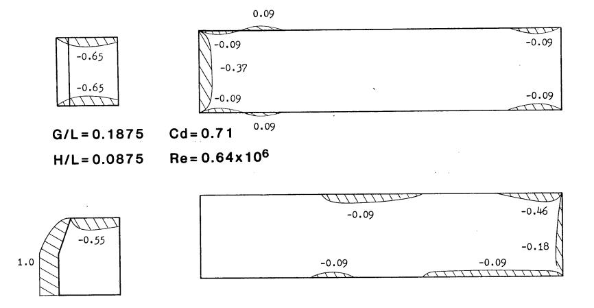
Figure 3-4. Typical pressure distribution on a conventional tractor-trailer configuration (G/L = 0.1875, H/L = 0.0875)
