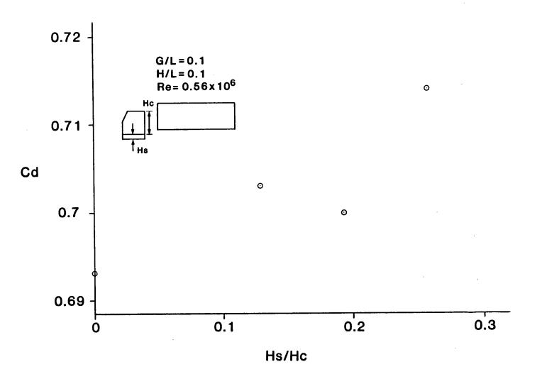
Figure 3-12. Drag coefficient versus non-dimensional tractor spoiler width Hs/Hc
