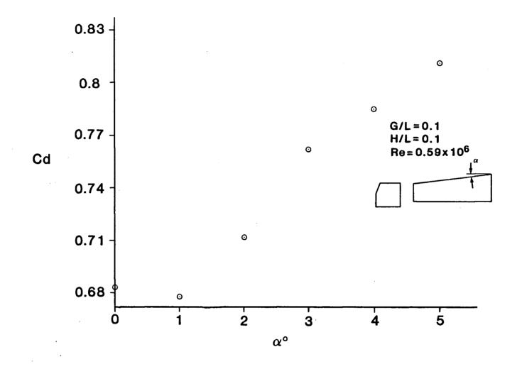
Figure 3-8. Variation of drag coefficient with trailer roof angle  $\alpha$  for forward sloping roofs
