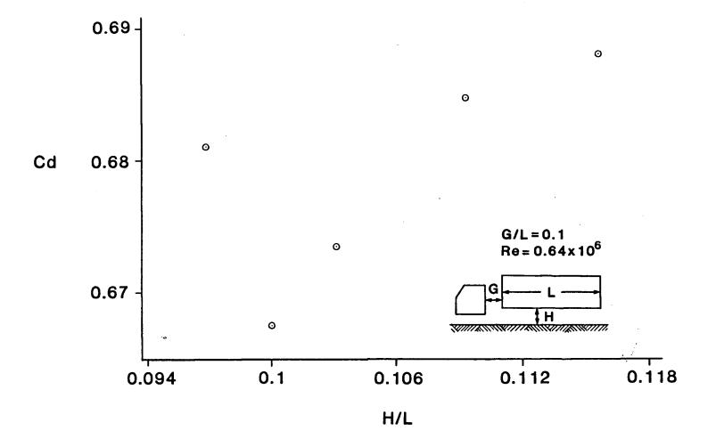
Figure 3-3. Effect of ground clearance on drag coefficient for a fixed tractor-trailer gap G/L = 0.1
