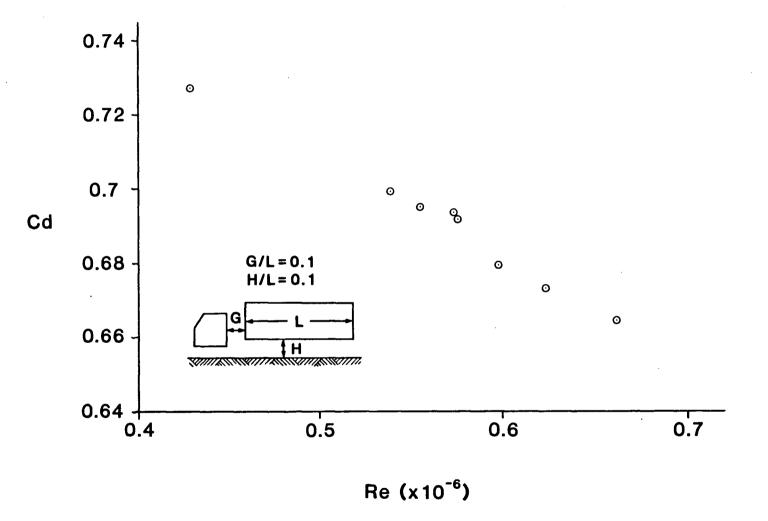
Figure 3-11. Variation of drag coefficient with Reynolds number for the optimum tractor-trailer configuration
