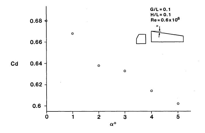
Figure 3-9. Variation of drag coefficient with trailer roof angle  $\alpha$  for backward sloping roofs
