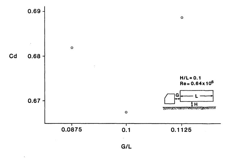
Figure 3-2. Variation of drag coefficient with tractor-trailer gap for a fixed ground clearance H/L = 0.1
