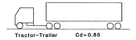
Figure 1-1. Drag coefficient of several common bluff bodies, automobiles and a typical tractor-trailer configuration.
