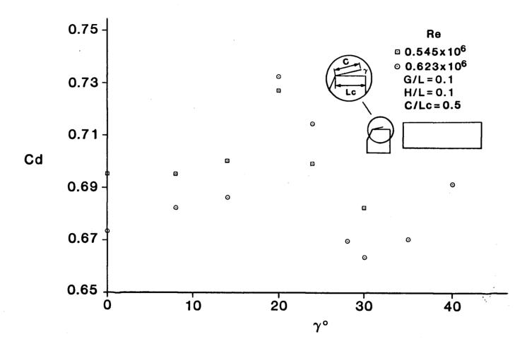
Figure 3-14. Variation of drag coefficient with tractor roof deflector angle  $\gamma$  for a given deflector length C/Lc = 0.5
