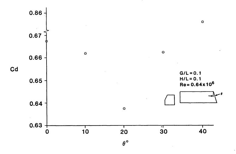
Figure 3-6. Drag coefficient versus trailer back angle  $\boldsymbol{\theta}$
