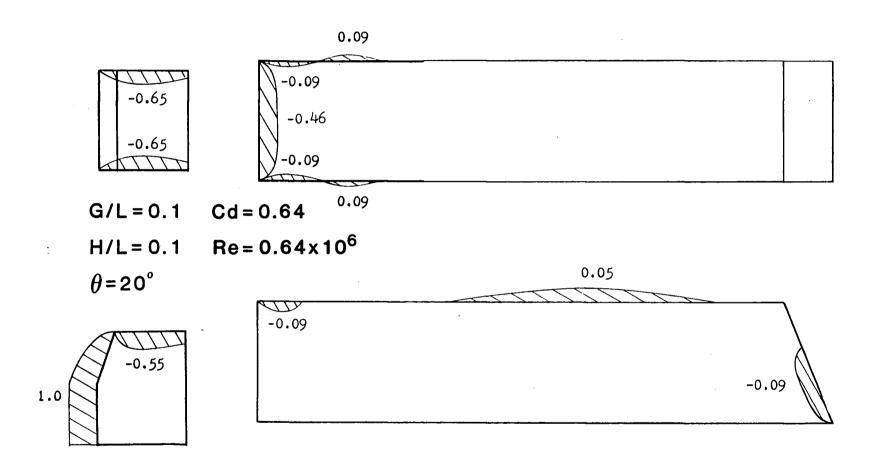
Figure 3-7. Pressure distribution on the optimum tractor-trailer configuration with  $20^{\circ}$  back angle
