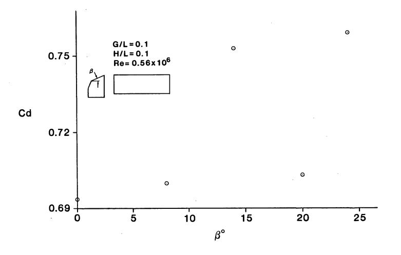
Figure 3-10. Effect of tractor roof angle  $\beta$  on drag coefficient
