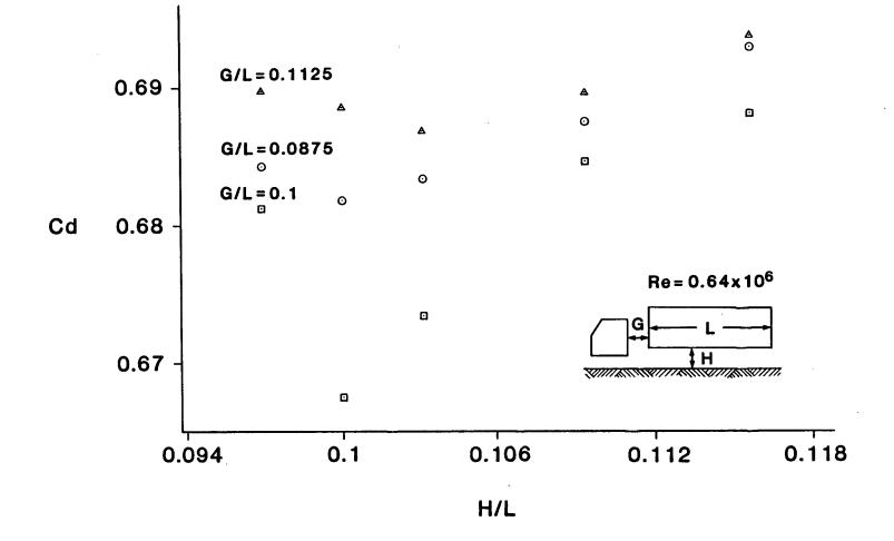
Figure 3-1. Drag coefficient versus ground clearance (H/L) for three different tractor-trailer gaps (G/L)
