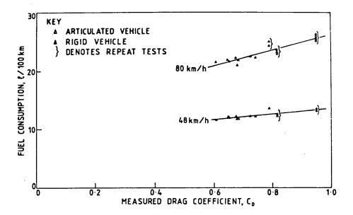
Figure 1-5. Correlation of fuel consumption and drag coefficient for full scale trucks as reported by Rose [7].
