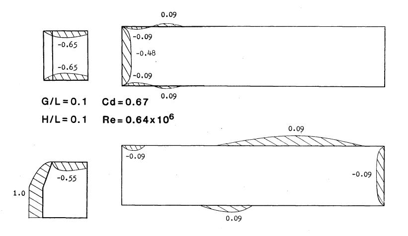
Figure 3-5. Pressure distribution on the optimum tractor-trailer configuration (G/L = 0.1, H/L = 0.1)
