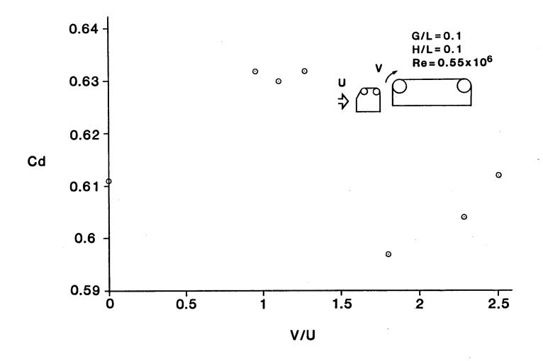
Figure 3-15. Effect of the trailer leading edge cylinder rotation on drag coefficient
