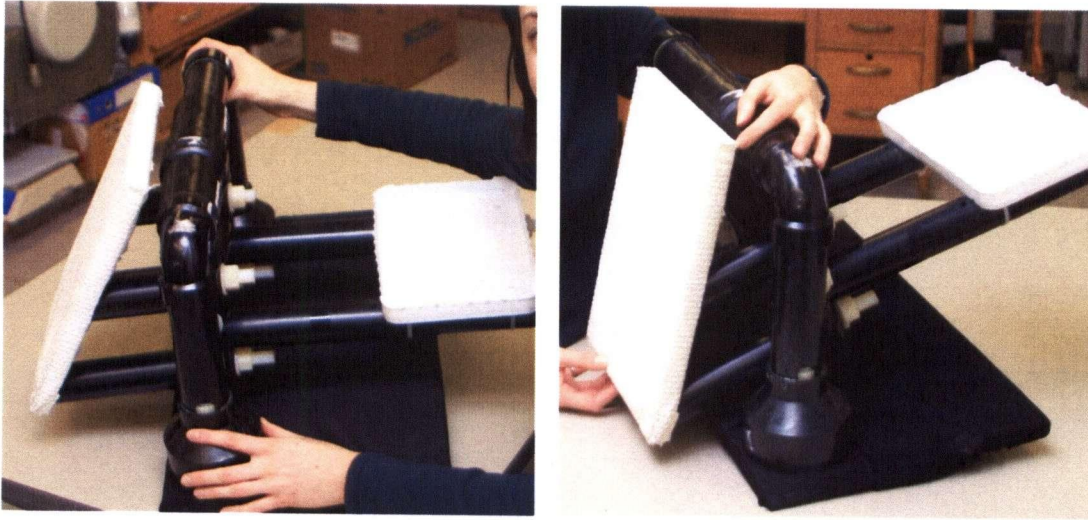
Figure 4.4: MR compatible loading rig. Left: Side view of the loading rig showing pedal, loading bed and frame. Right, Oblique view of the loading rig showing the pedal and loading bed rotating about the U-shaped frame.
