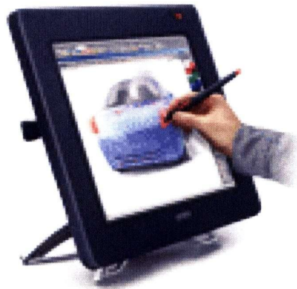
Figure 3.2: The Cintiq 18SX by Wacom, a touch-sensitive screen on which the user can write with a digitizing pen to move the cursor through the workspace. Ref: http://www.wacom.com/lcdtablets/index.cfm
