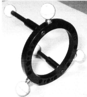
Figure 2.4: MDMArray. Halo of optical passive marker balls used for optical position tracking. The infrared camera tracks faces (3 balls) of the array.
