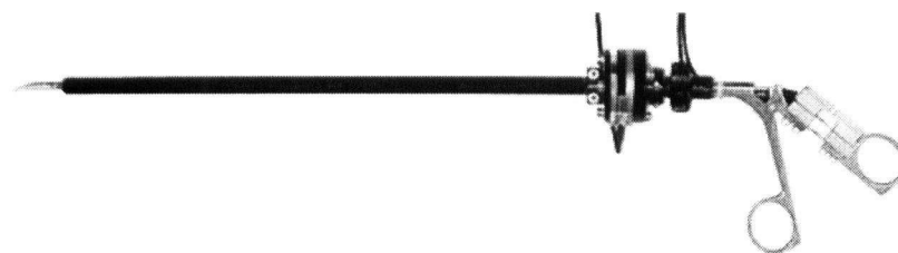
Figure 2.6: F/T system of Rosen (1999). A custom-designed F/T sensor was mounted directly onto the surgical tool shaft. This sensor has a hole through the center. A strain gauge system is mounted onto the tool handle.
