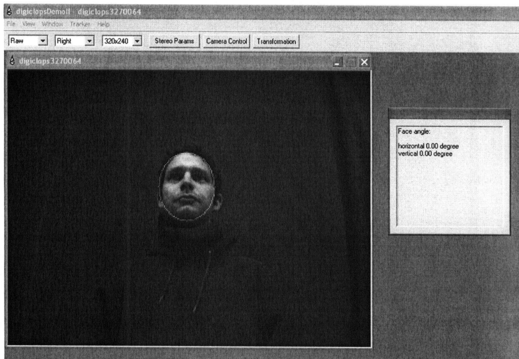
Figure 7.25. Head orientation tracking (horizontal angle = 0, vertical angle = 0).
