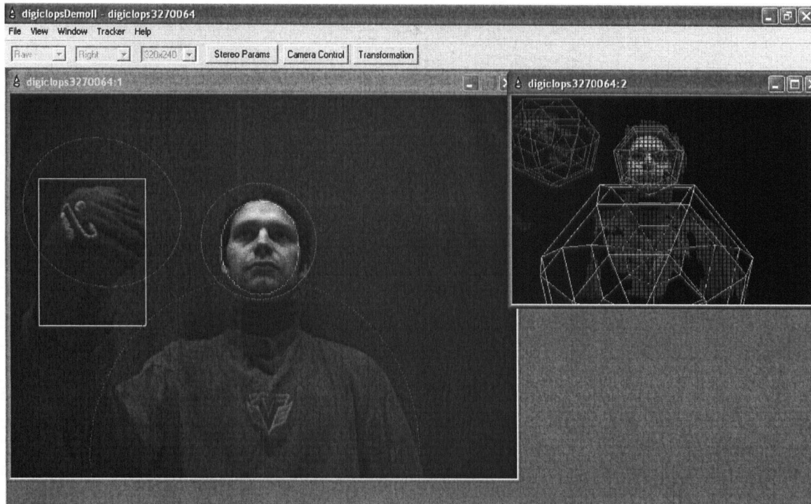
Figure 7.10. Hand and body tracking results (ending hand position).
