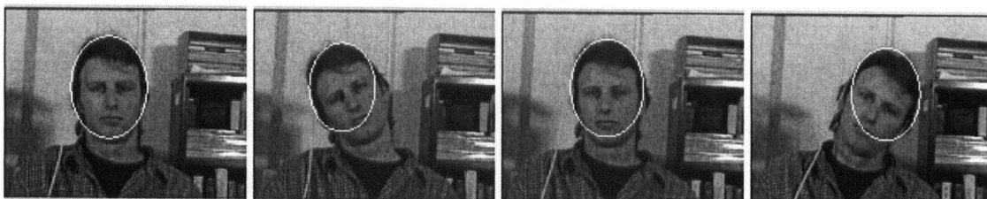
Figure 6.19. Tracking results when estimating the face location and scale only.
