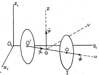
reference system fixed in space and let the wheels move on the plane Z=0 (the wheel with centre 0' having a contact without friction and that with centre 0 having a perfectly rough contact).
