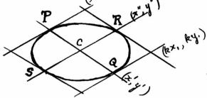
Let (x, y, ) and (kx, ky) be parallel lines tangent to the conic  $ax^2+2hxy+by^2+2gx+2fy+c = 0$ at the points P and Q respectively. The equations of P and Q are (ax, +hy, +g)x + (hx, +by, +f)y + gx, +fy+c = 0and (k(ax, +hy) + g)x + (k(hx, +by) + f)y + k(gx, +fy) + c = 0respectively. On solving, we obtain the co-ordinates of the diameter through P and Q, viz.,
