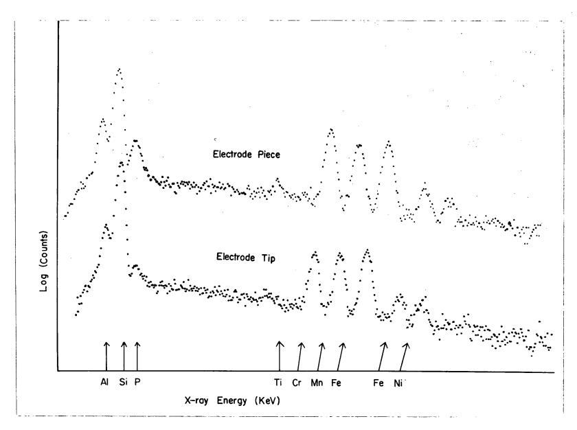
Figure 46(a). EDXA plots of inclusions in the electrode piece dropped in Valve No. 9 and the electrode tip.
