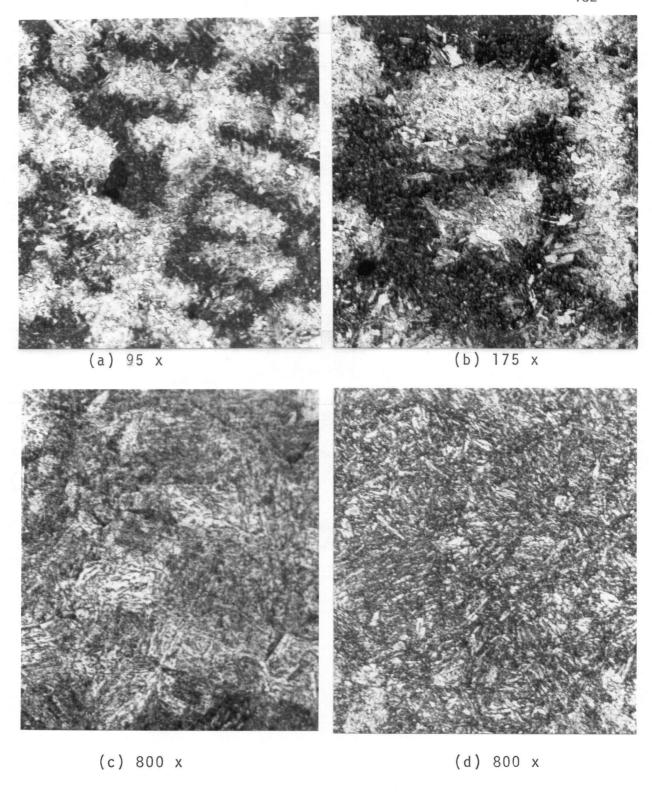
Figure 76. Microstructure of AISI 4340 ESC Valve No. 13 in heat-treated condition.
