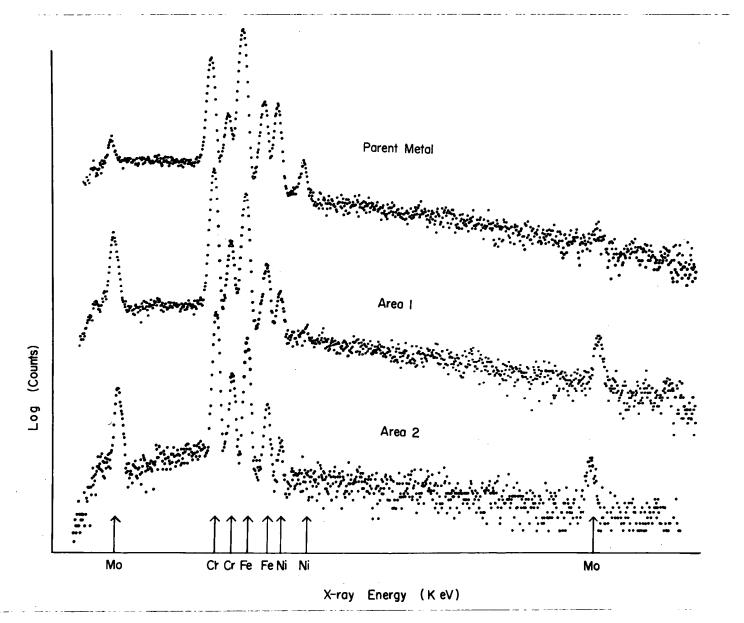
Figure 39. EDXA plots of agglomerated ferro alloy powder in areas 1 and 2 and the parent metal (Valve No. 10).
