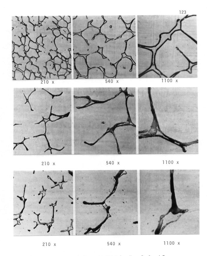
Figure 21. Microstructure of as-cast ESC Valve Nos. 5, 6 and 7 (etchant - oxalic acid).
