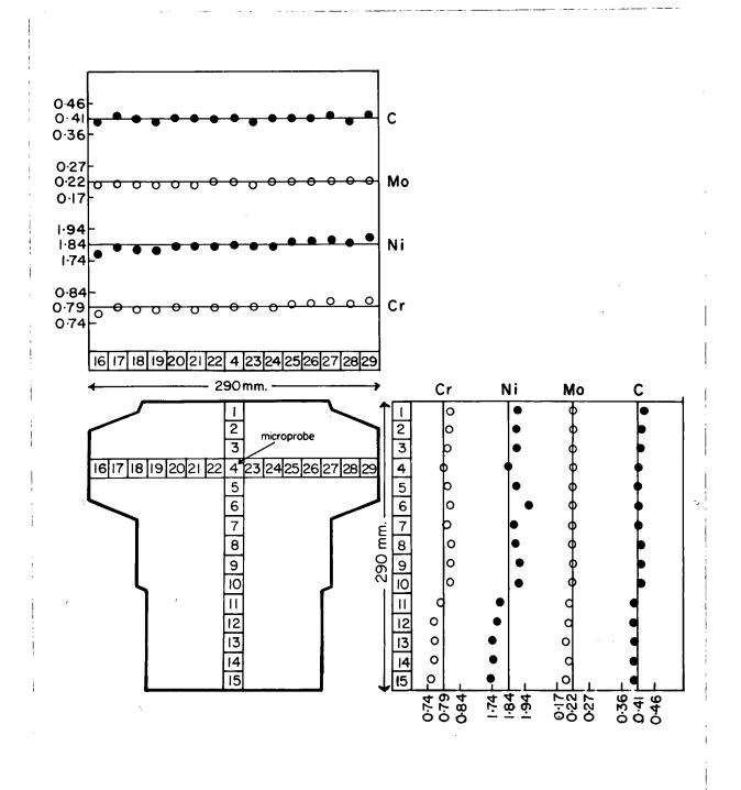
Figure 68. Composition variation in Valve No. 8. (The solid line shows the overall average composition.)
