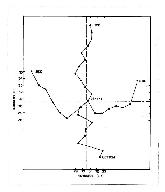
Figure 74. Hardness variation in heat-treated Valve No. 14.
