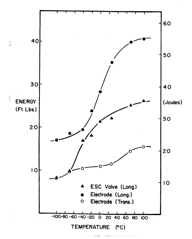
Figure 79. Ductile Brittle transition characteristics of Valve No. 3 and the electrode.
