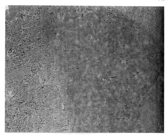
Figure 42. Macrostructure of the electrode piece that dropped in Valve No. 9.
