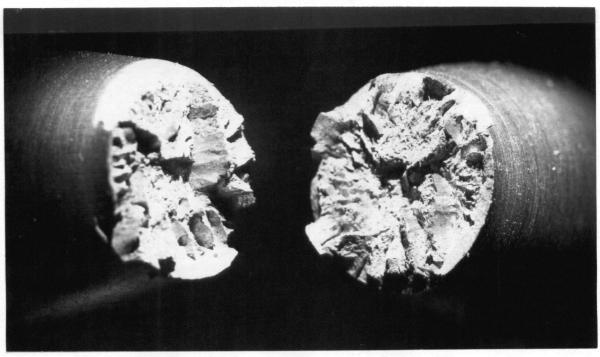
Figure 77. Fractographs of large tensile specimens of AISI 4340 from ESC Valve No. 8.
