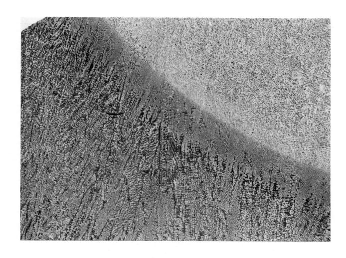
Figure 48. Macrostructure of the peculiar pool profile observed in Valve No. 9. (5.5X)
