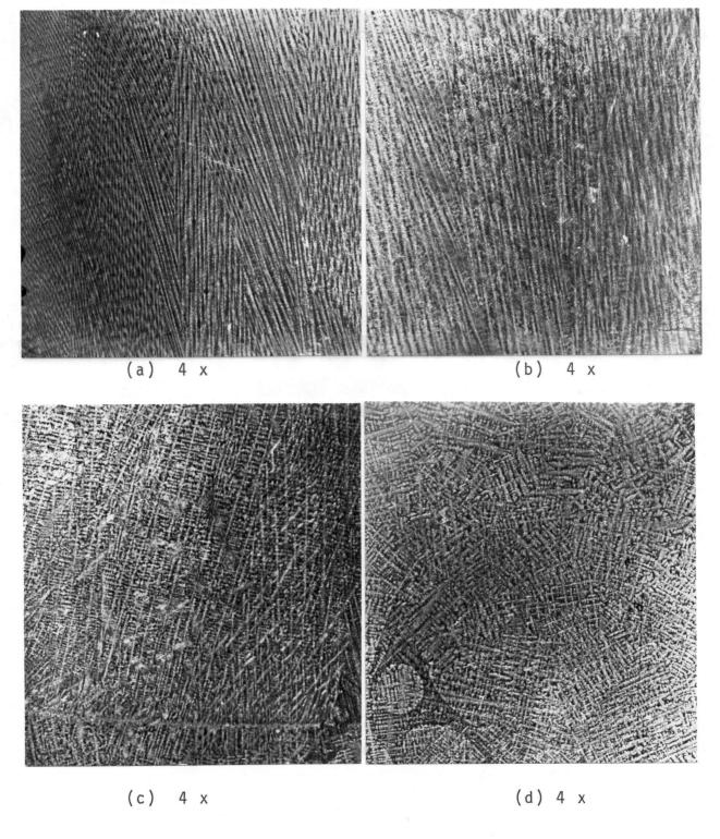
Figure 61. Dendritic structure of Valve No. 3.
