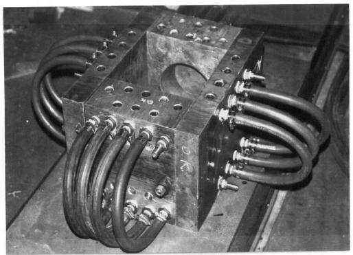
Figure 8. Assembled valve mold.
