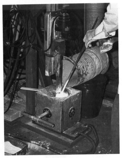
Figure 9. Slag melting furnace.
