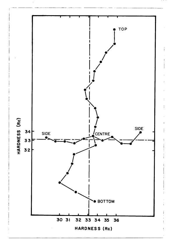
Figure 73. Hardness variation in heat-treated Valve No. 13.
