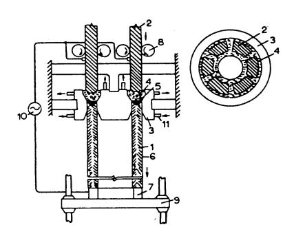
1 straight tube, 2 source material, 3 ringtype mould, 4 molten-slag bath, 5 moltenmetal pool, 6 slag film, 7 start piece, 8 feed roller for source material, 9 drawing apparatus, 10 electric power source, 11 cooling water
