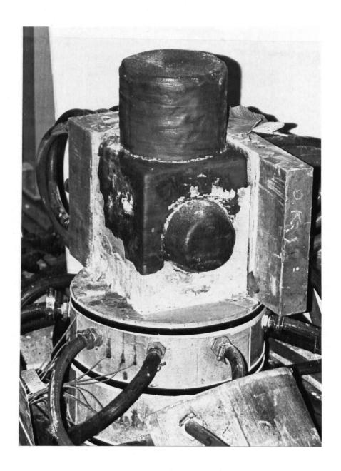
Figure 10. Solidified slag skin on the casting.
