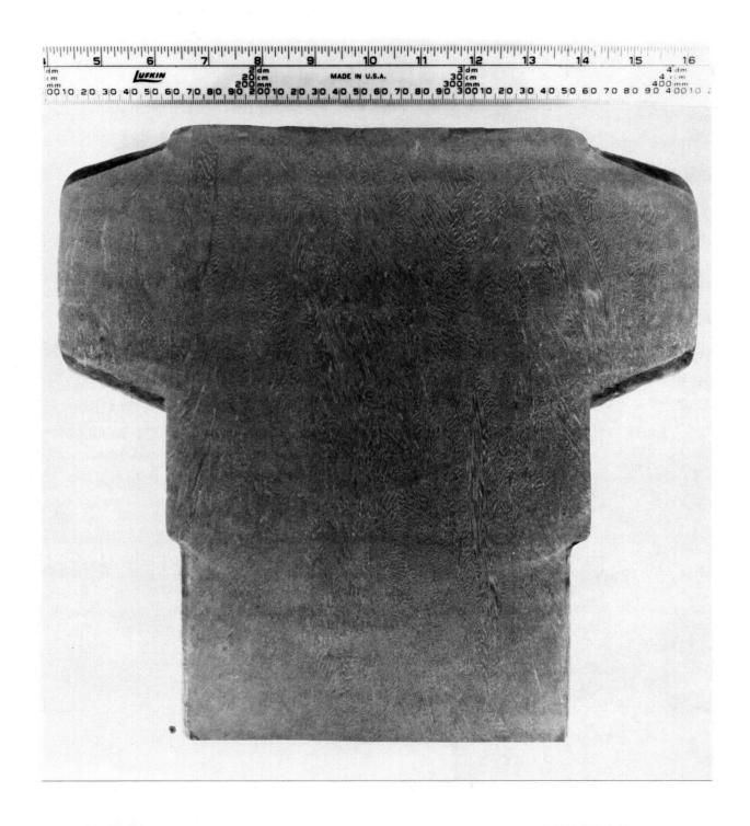
Figure 57. Macrostructure of Valve No. 8 (HCl etch).
