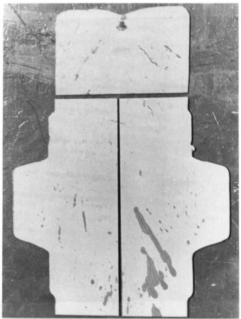
Figure 54. Cracks in Valve No. 14 revealed by dye-penetrant test.
