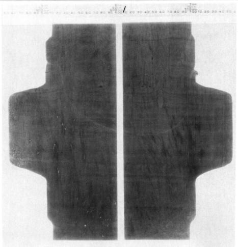
Figure 59. Macrostructure of Valve No. 14 (Hcl etch) (top part etched for a longer time).
