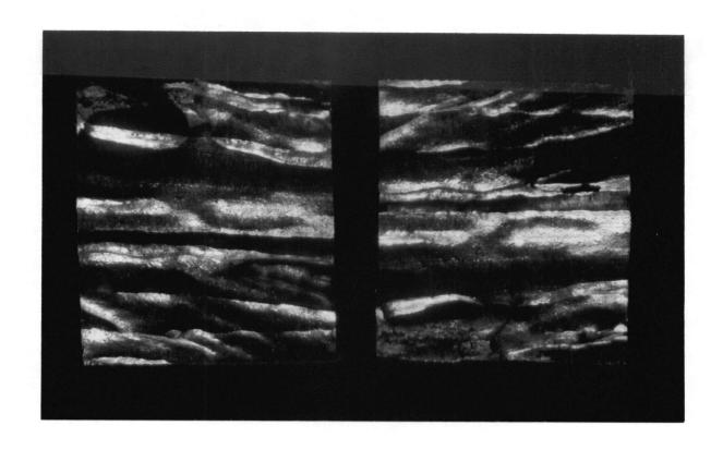
Figure 72. Separated surfaces along a crack in Valve No. 14.
