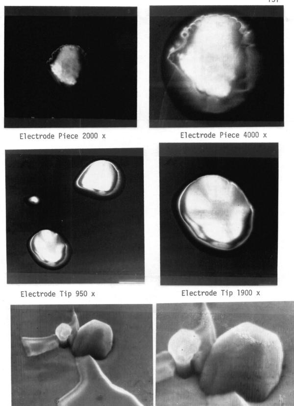
Figure 45. Inclusions in the electrode piece dropped in Valve No. 9, electrode tip and the parent casting (Valve No. 9).
