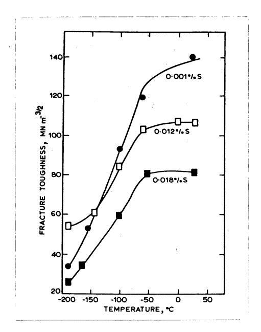
Figure 4. Fracture toughness of ESC AISI 4340 steel containing varying amounts of sulphur. <sup>2</sup>
