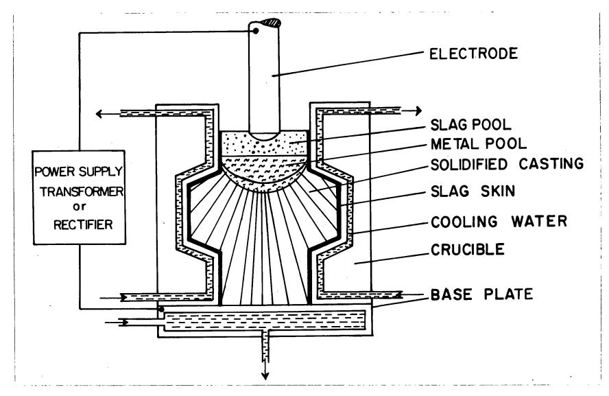
Figure 3. Schematic of the ESC process.
