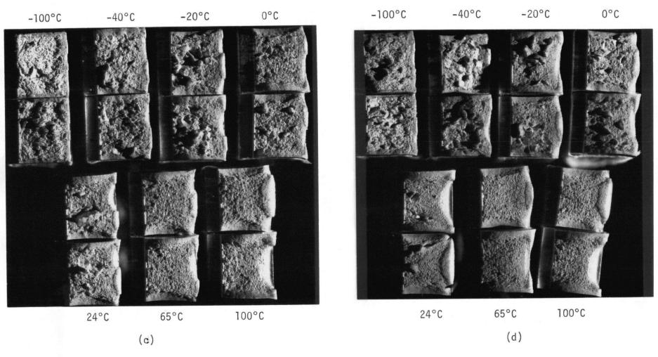
Figure 82. Optical fractographs of charpy specimens from Valve No. 8 tested at different temperatures and orientations.
