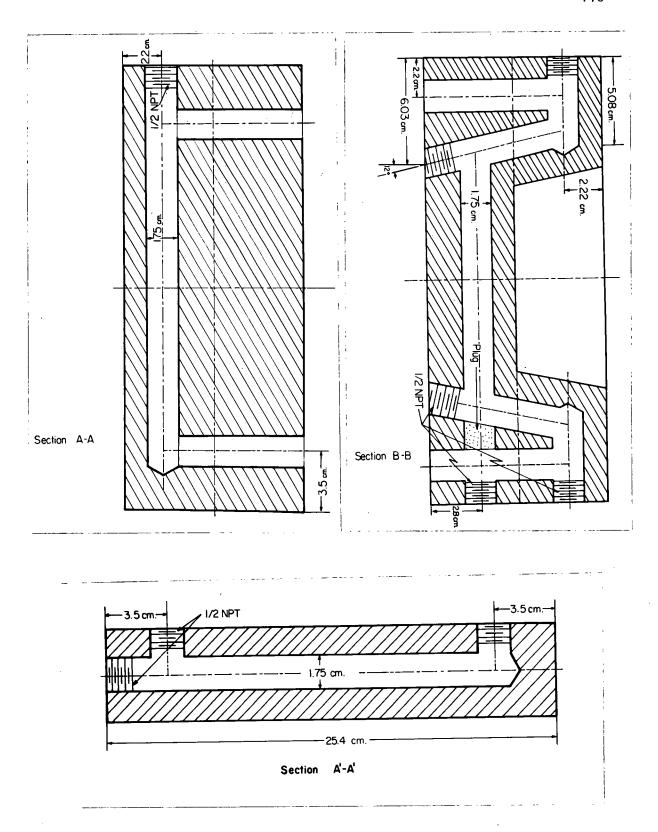
Figure 7(b). Sections through the valve mold segments.
