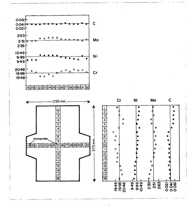
Figure 34. Composition variation in Valve No. 9 (CF-8M). (The solid line shows the overall average composition.)
