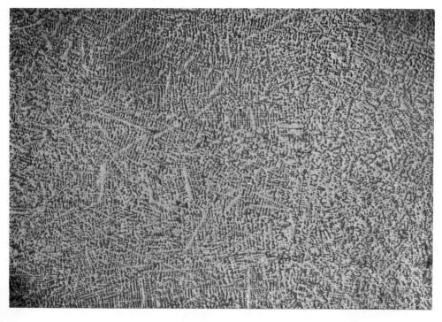
Figure 43. Macrostructure of the CF-8M electrode.
