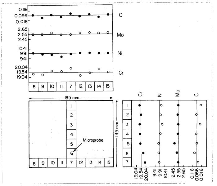
Figure 31. Composition variation in Valve No. 5 (CF-8M). (The solid line shows the overall average composition.)
