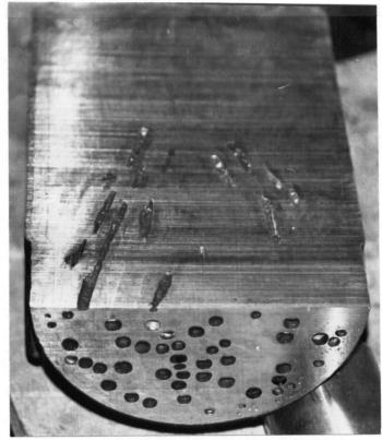
Figure 13. Longitudinal holes in the castings due to moisture.
