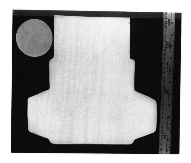
Figure 63. Sulphur Prints of Valve No. 8.
