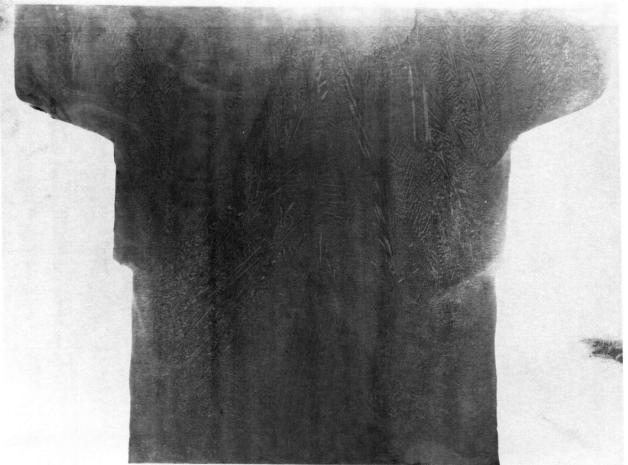
Figure 56. Macrostructure of Valve No. 3 Top - HCl etch. Bottom -  $(NH_4)_2$   $SO_4$  etch.
