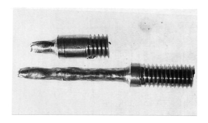
Figure 51. Photograph of the deformed and fractured areas of small tensile specimen from Valve No. 6.
