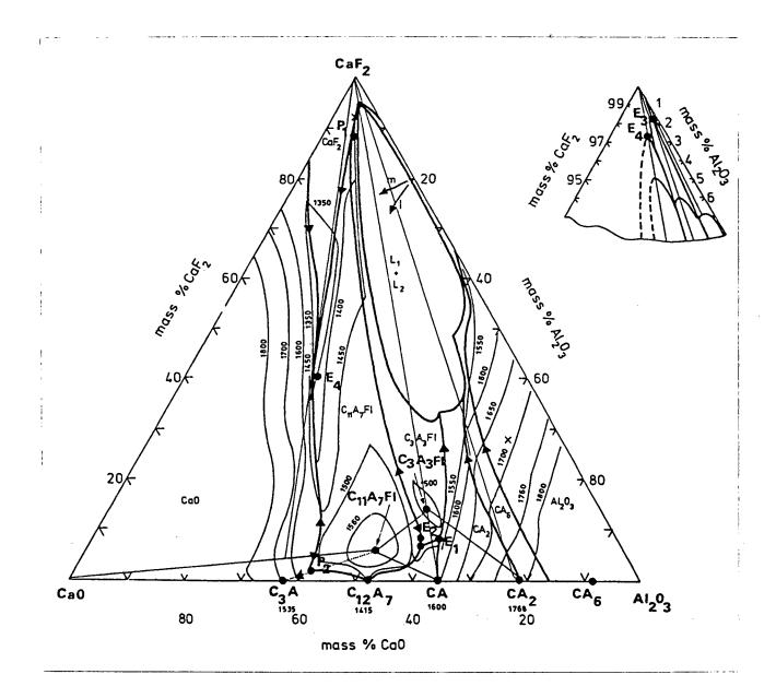
Figure 11. Phase diagram for  $CaF_2-A\ell_2^0_3$ -CaO system. 48
