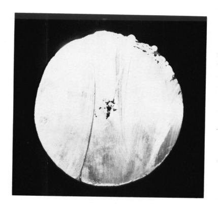
Figure 41. Macroporosity in the Centre of the CF-8M electrode.
