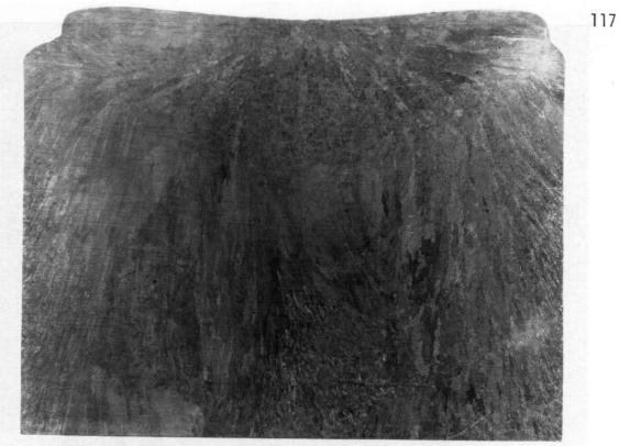
Figure 15. Macrostructure of Valve No. 5 (CF-8M).
