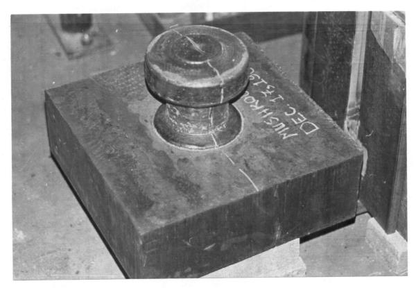
Figure 88. Electroslag casting of a flange for use in valve bodies.
