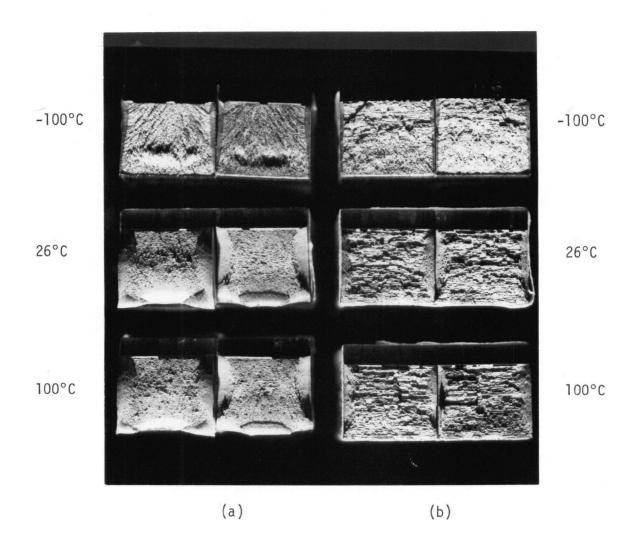
Figure 83. Optical fractographs of charpy specimens from the AISI 4340 electrode.
