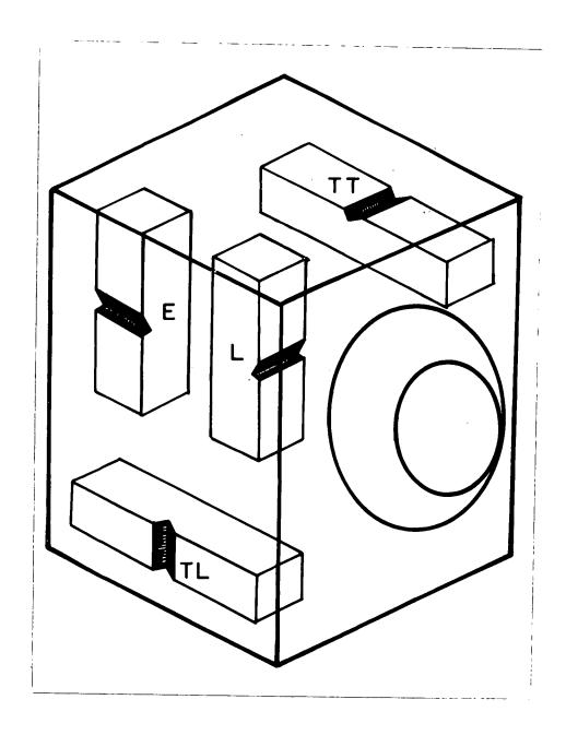
Figure 78. Orientation of the charpy specimens and the notch in Valve No. 8.
