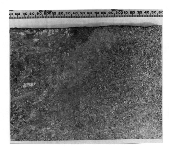
Figure 19. Macrostructure of conventional casting (CF-8M).
