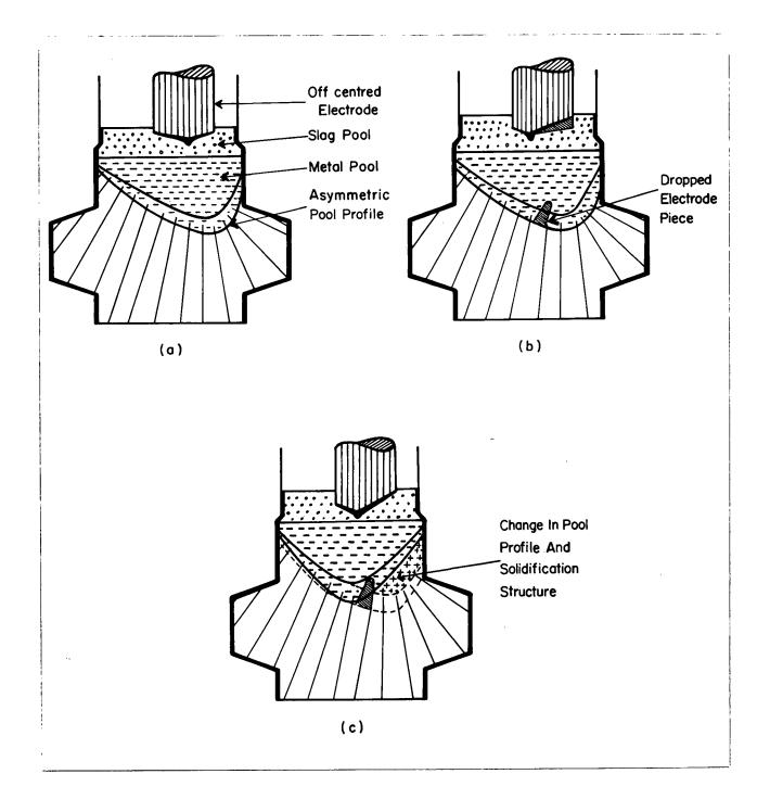
Figure 47. Schematic to explain the peculiar pool profile observed in Valve No. 9.
