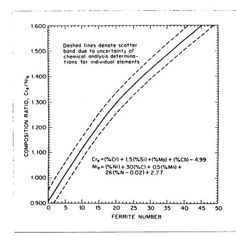
Figure 28. Schoefer's diagram for determination of ferrite numbers of stainless steel castings.
