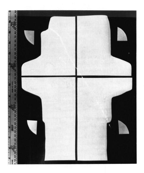
Figure 62. Sulphur prints of Valve No. 3.
