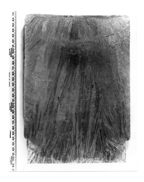
Figure 18. Macrostructure of Valve No. 10 (316+Cr+Mo).
