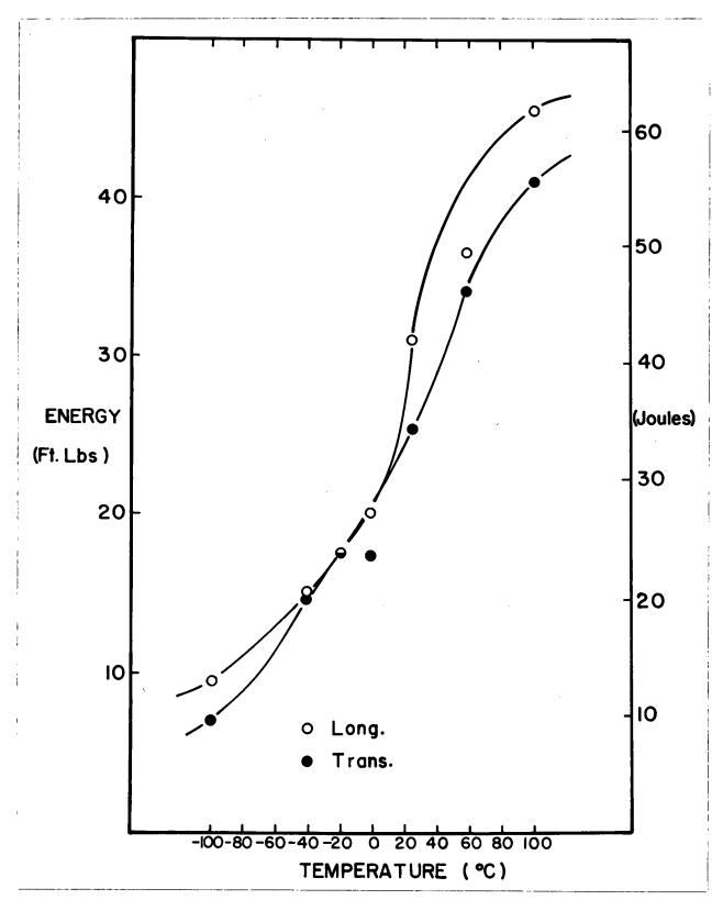
Figure 81. Ductile brittle transition characteristics of Valve No. 13. Heat Treatment: 1 hour at  $845^{\circ}\text{C}$  - oil quench. Temper at  $560^{\circ}\text{C}$  to a hardness of 35 Rc.
