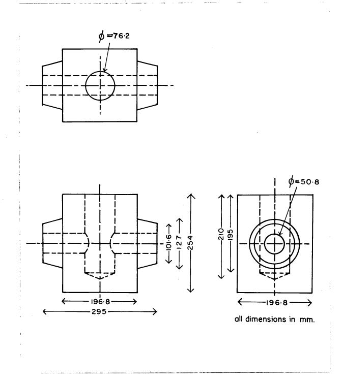
Figure 6. Onthogonal views of ESC valve body.
