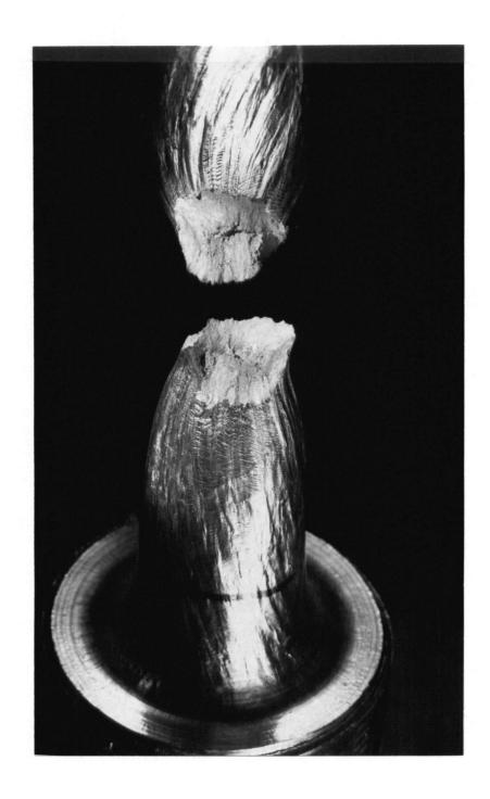
Figure 52. Photograph of the deformed and fractured areas of large tensile specimen from Valve No. 6.
