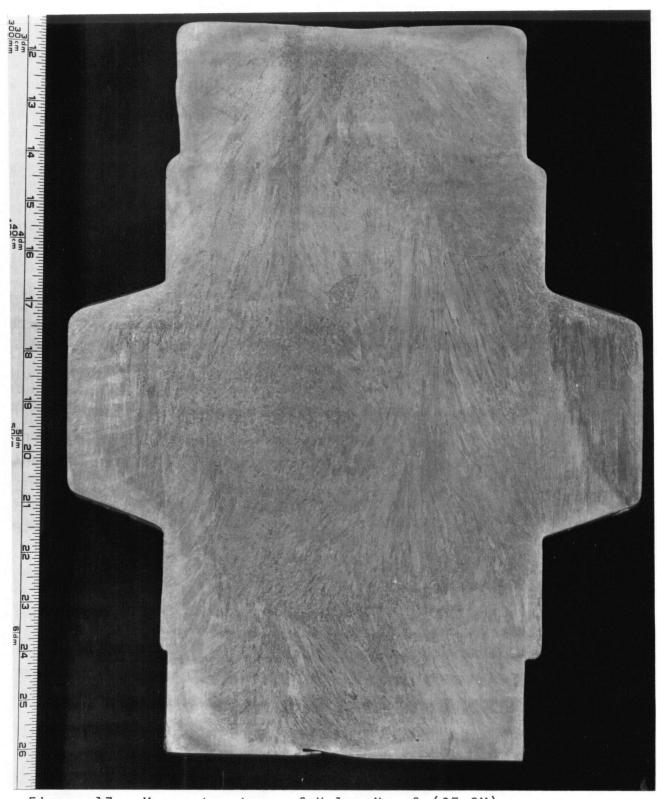
Figure 17. Macrostructure of Valve No. 9 (CF-8M).
