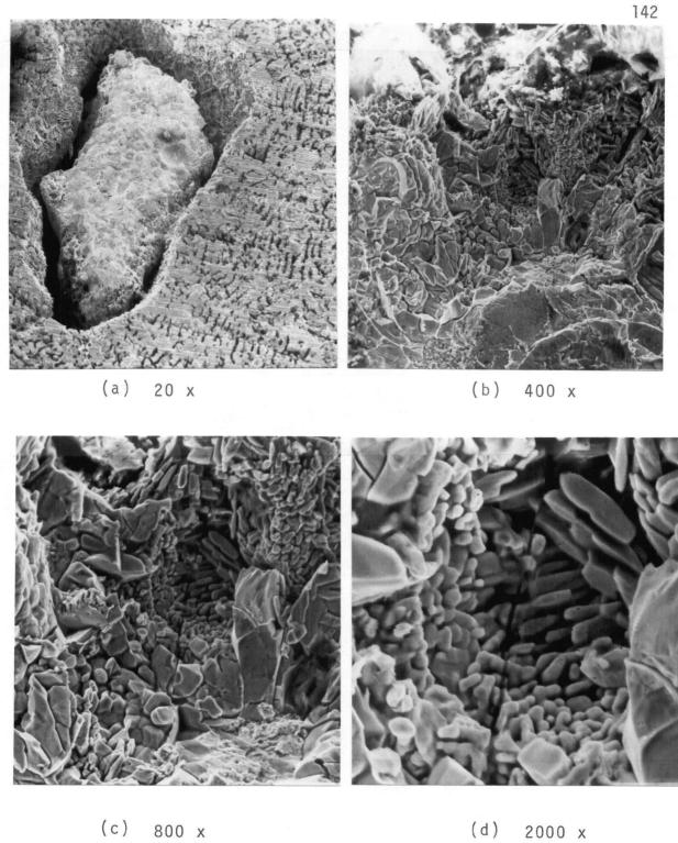
Figure 37. SEM photographs of agglomerated ferro alloy powder in area 1 in Valve No. 10.
