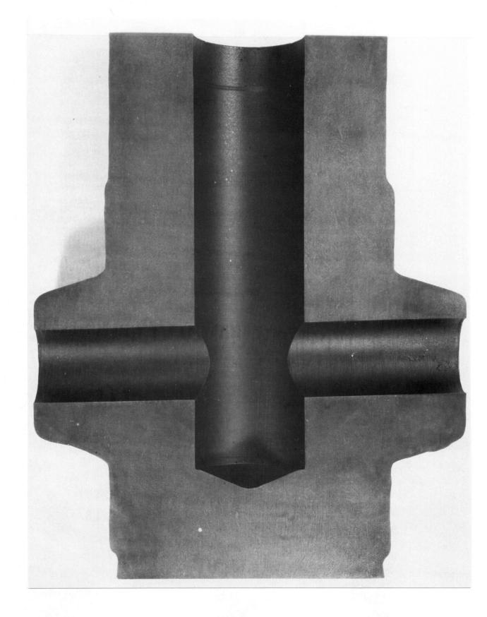
Figure 58. Macrostructure of Valve No. 13 (HCl etch).
