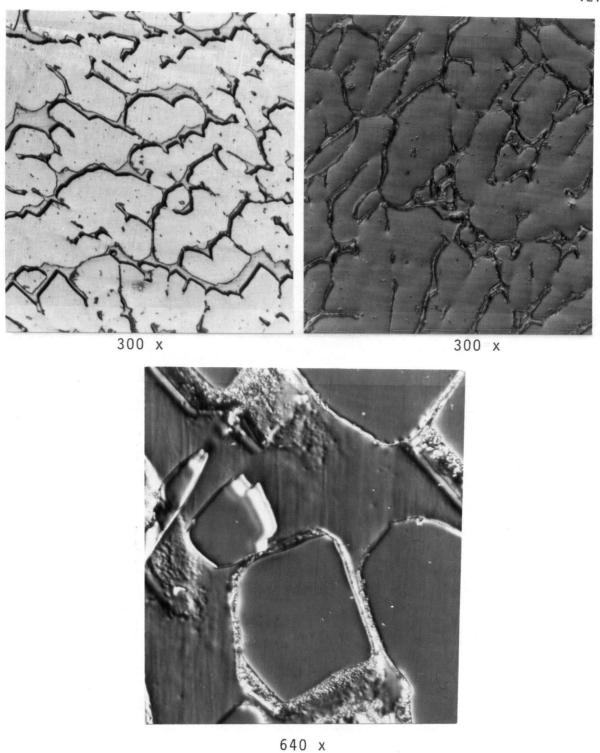
Figure 20(a). Microstructure of CF-8M ESC valves before heat treatment (etchant - oxalic acid).
