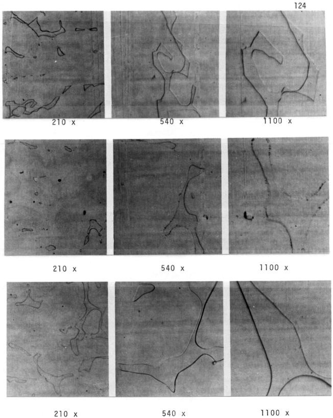
Figure 22. Microstructure of heat-treated ESC Valve Nos. 5, 6 and 7 (echant - oxalic acid). Top Row - Valve No. 5 (CF-8M), Middle Row - Valve No. 6 (316) Bottom Row - Valve No. 7 (316+Cr).
