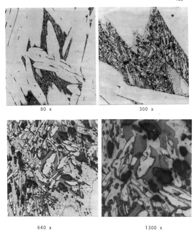
Figure 23. Microstructure of CF-8M specimen heated to  $850\,^{\circ}\text{C}$  (etchant - KOH).
