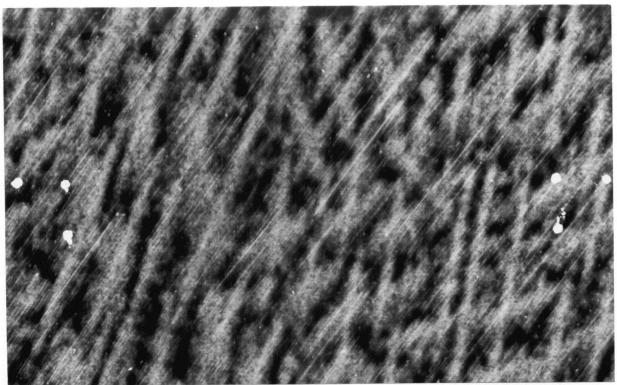
Figure 65. Variation of Cr, Ni and Mo across the dendritic direction in Valve No. 13.
