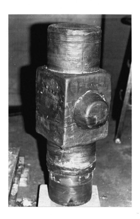
Figure 53. AISI 4340 ESC valve.
