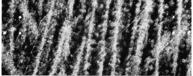
Figure 66. Variation of Cr, Ni and Mo across the dendritic direction in Valve No. 14.
