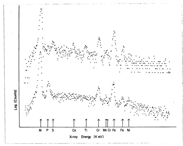
Figure 46(b). EDXA plots of inclusions in the parent casting (Valve No. 9).
