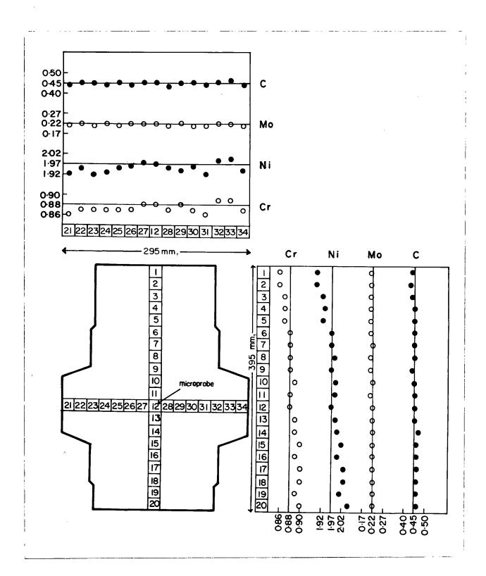
Figure 70. Composition variation in Valve No. 14. (The solid line shows the overall average composition.)
