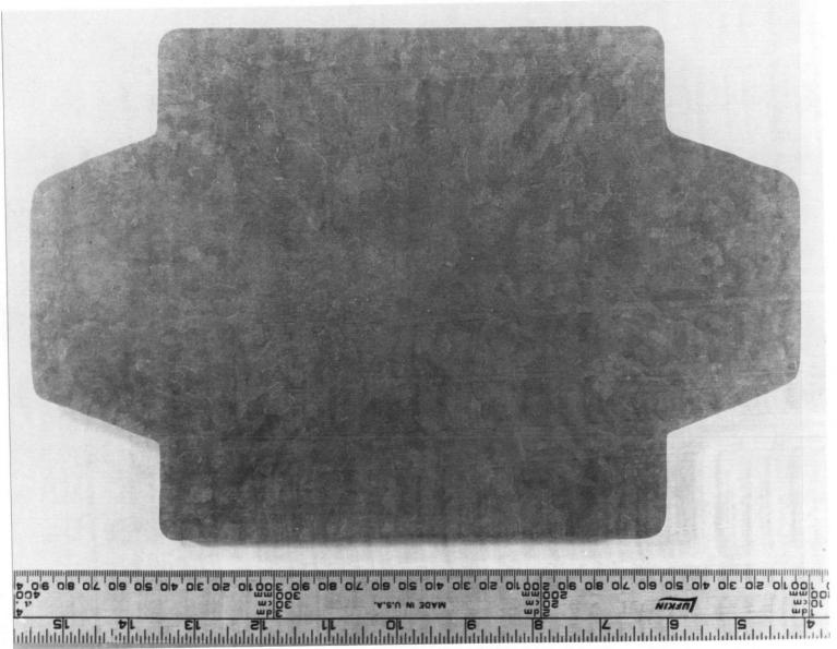
Figure 60. Macrostructure of the transverse section of a mild steel ESC valve (HC $_{\ell}$  etch).
