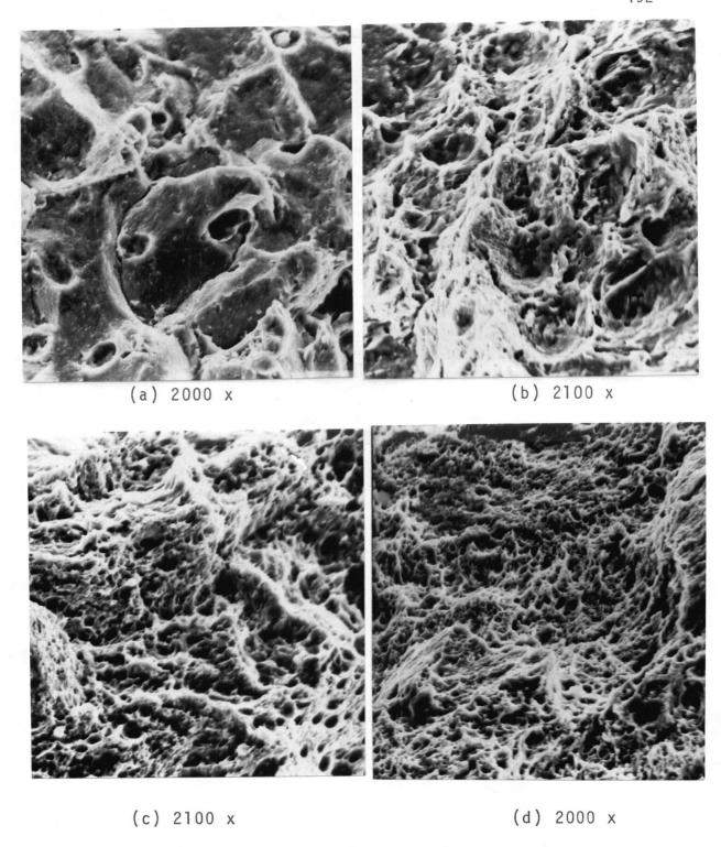
Figure 85. SEM fractographs of different regions of a charpy specimen.
