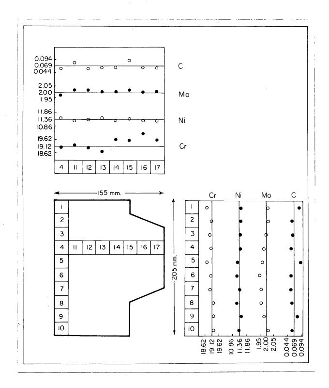
Figure 33. Composition variation in Valve No. 7 (316+Cr). (The solid line shows the overall average composition.)
