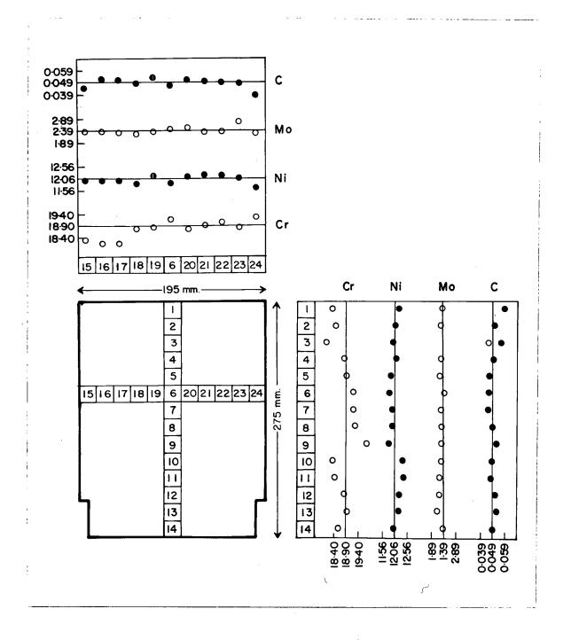
Figure 35. Composition variation in Valve No. 10 (316+Cr+Mo). (The solid line shows the overall average composition.)
