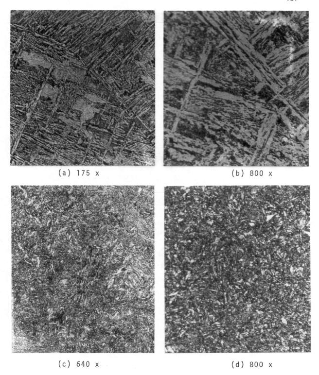
Figure 75. Microstructure AISI 4340 valve in as-cast and heat-treated conditions; electrode in heat treated condition.
