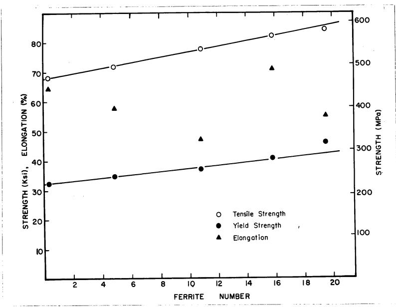
Figure 50. Variation of tensile properties with ferrite number of stainless steel castings.
