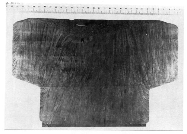
Figure 16. Macrostructure of Valve No. 6 (316).
