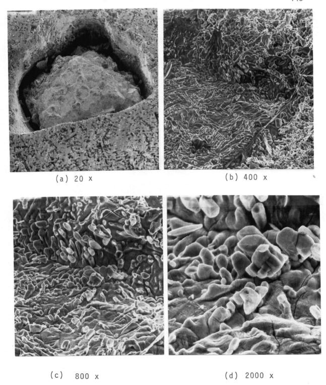
Figure 38. SEM photographs of agglomerated ferro alloy powder in area 2 in Valve No. 10.
