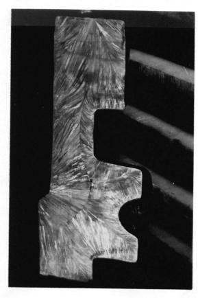
Figure 86. Soviet electroslag cast valve.
