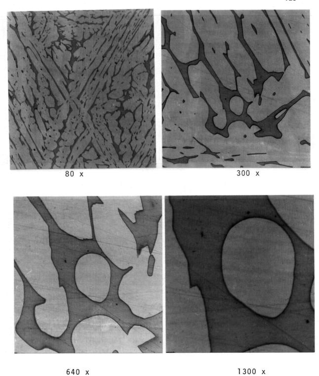
Figure 26. Microstructure of Valve No. 9 in heat-treated condition (etchant - KOH).
