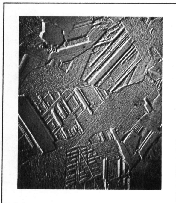
Fig. 20 99.998% cobalt, 47 micron grain size, 2000X
