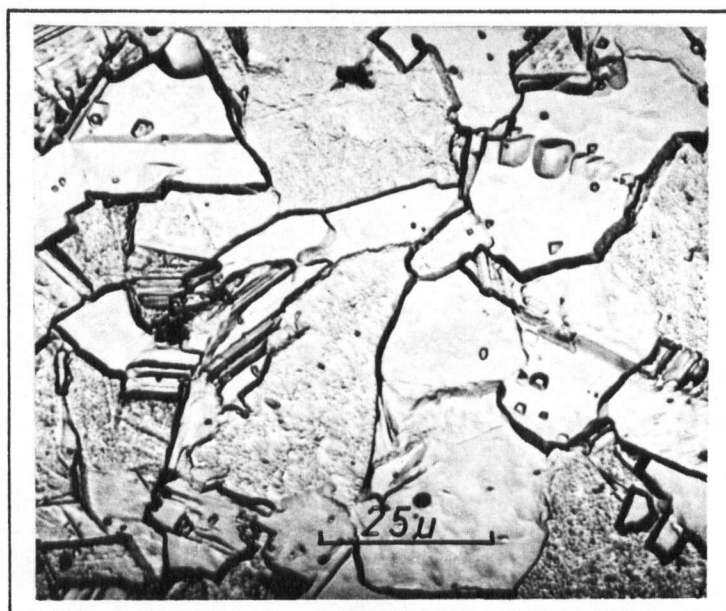
Fig. 8 99.9% cobalt, annealed at 900^{\circ}\text{C} for 1 hr. 39\mu .
