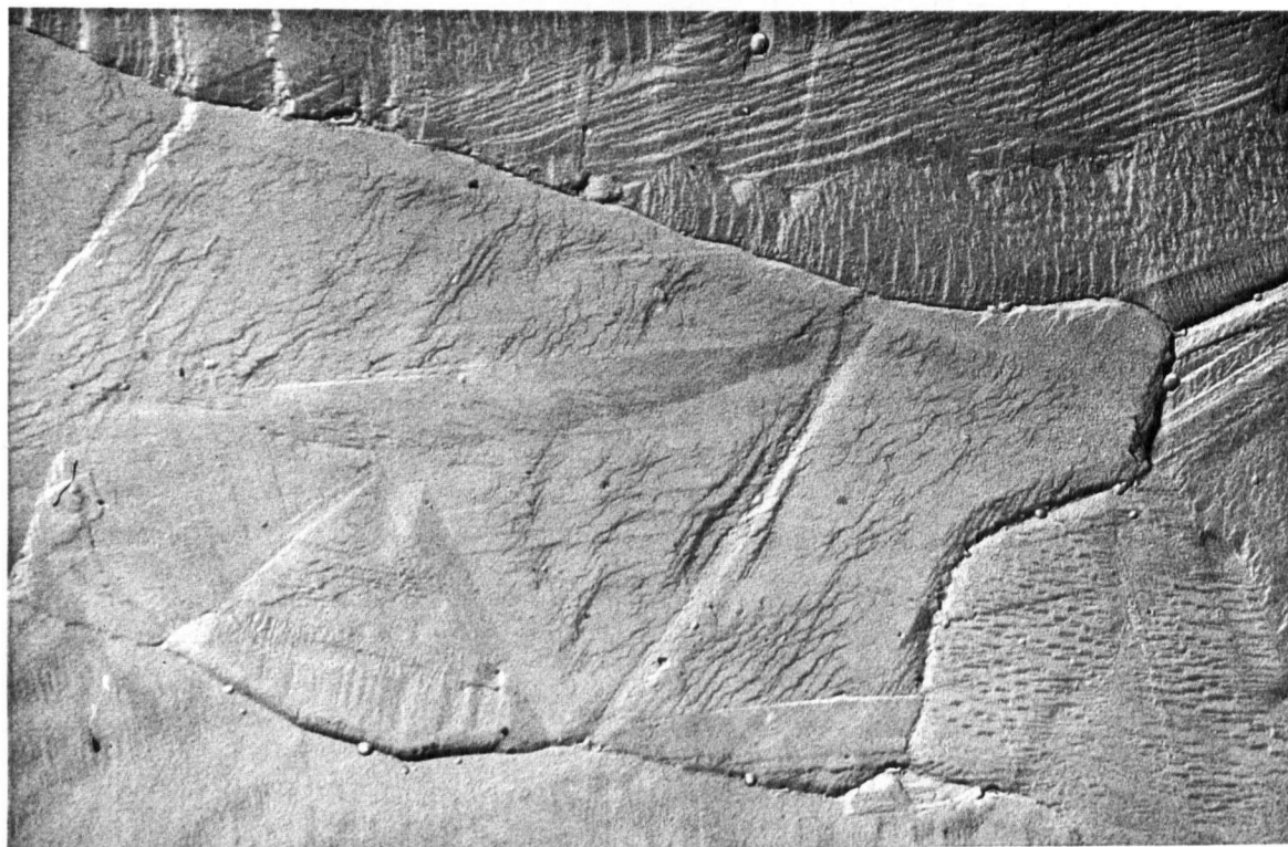
Fig. 61 Twinning in cobalt at 250^{\circ}\text{C} . 3700X
