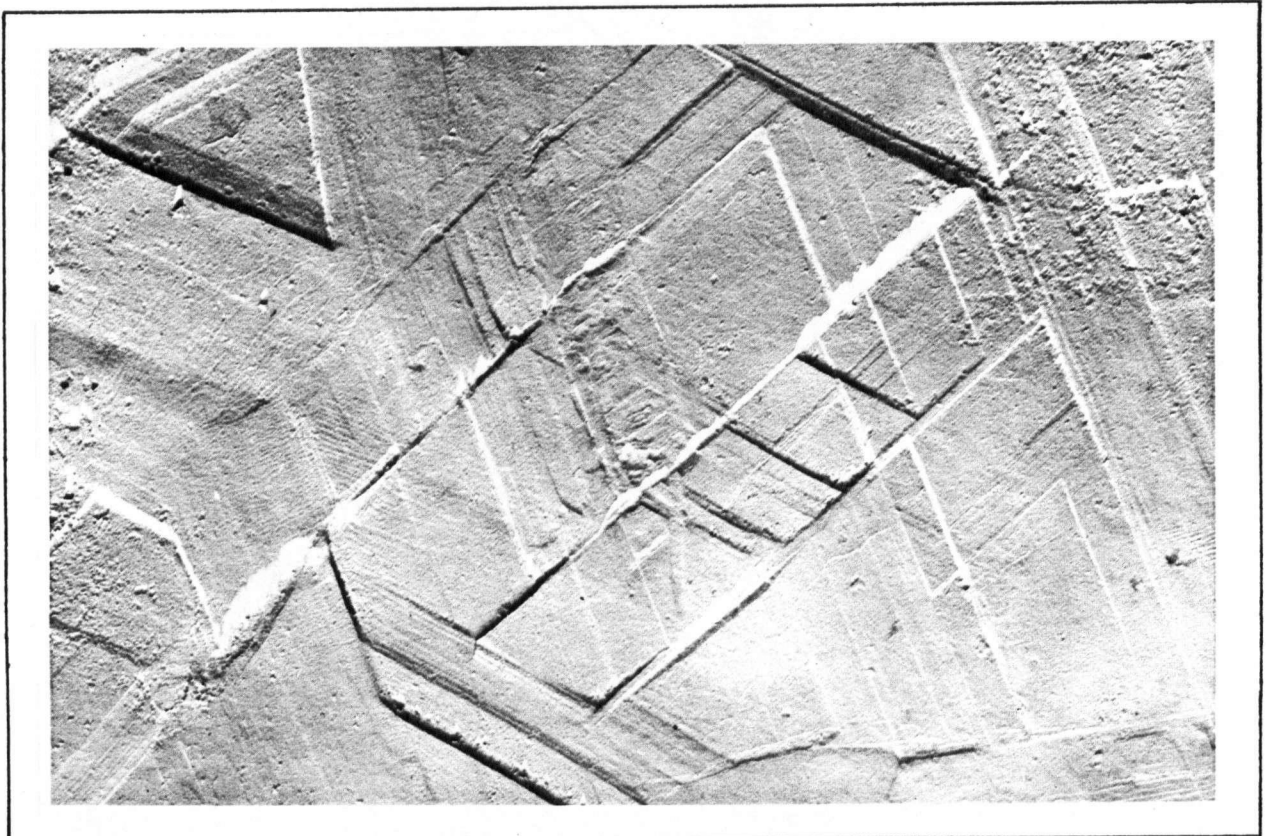
Fig. 59 Typical surface shear markings in cobalt. -196^{\circ}\text{C} Test. 6500X
